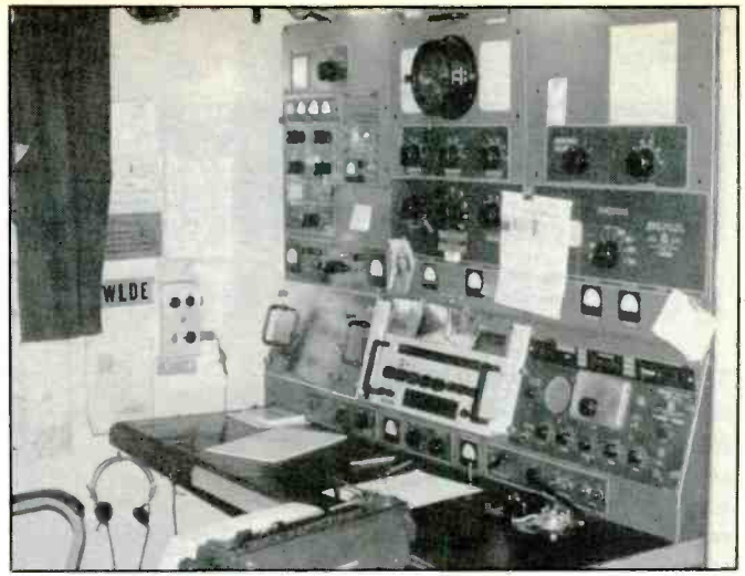
This shipboard console contains an emergency battery-operated transmitter and receiver, an auto-alarm (which rings very loud bells in the radio officers cabin if a distress signal comes in while he is off watch), as well as the main MF transmitter, HF transmitter and two all-band receivers.
