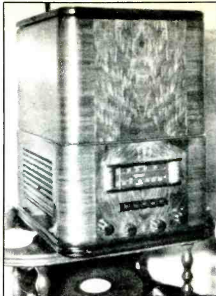
The Crosley Model 758 "Reado" receiver was designed to pick up FAX transmissions sent out by mediumwave broadcasting stations.
