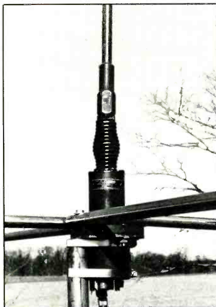
Converting the AS-1729/VCR to base operation is simple: just add four 1/4-wave ground plane radials (eight feet long). Standard seven-eighths inch (OD) steel electrical tubing is used.
