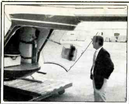
Boston MedFlight Director Alasdair Conn, MD, checks the interior of the BK 117. The "clamshell" doors at the rear of the helicopter allow greater access for two stretcher-borne patients.
