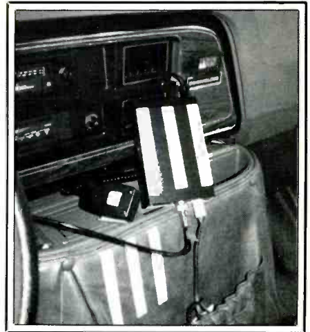
The Velcro strips shown in place on the rig and the mounting location. Note small Velcro patch used as mic hanger.
