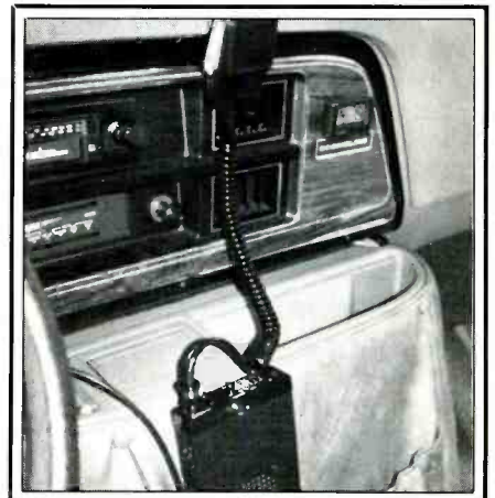
The Velcro-mounted CB installation shown completed.
