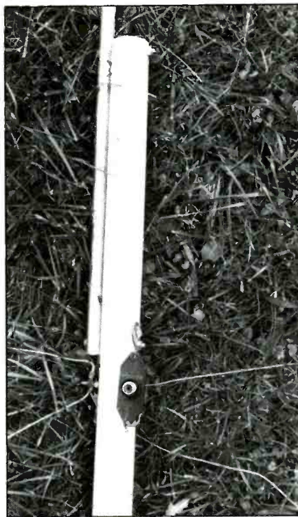
Figure 2: Mast tap arrangement showing lower part of aluminum radiator, four radial wires, and dipole-to-line connector.
