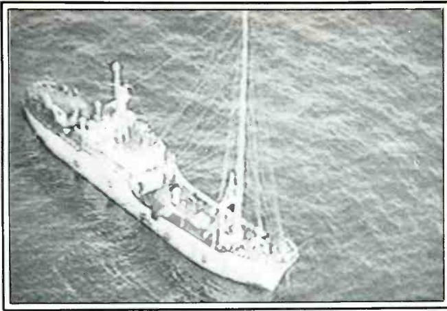
Aerial view of the M/V Sarah shows the antenna mast located towards the vessel's bow, and heavily guyed.
