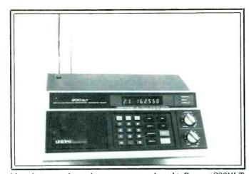
Many better grade modern scanners, such as this Bearcat 800XLT can receive frequencies higher in the spectrum than the old 512 MHz UHF-T band limit. Converters are also available to permit older scanners to receive various frequencies above 500 MHz.
