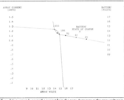
Self regulation occurs because the current from the array decreases as the array voltage increases. As the state of charge of the battery increases the terminal voltage increases. The sudden rise in battery voltage at full charge is what the array needs to "see" to shut down the current. (Courtesy BHC, Inc., Houston, Texas.)
