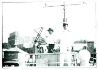
This U.S. Coast Guard cutter was equipped with a radio direction finder used to zero in on radio transmissions from offshore rum runners during the Prohibition years.
