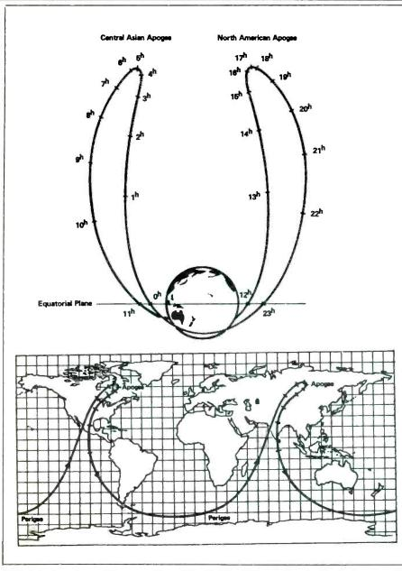
Figure 1: An orthographic projection of the Stabilized Ground Track of a Molniya satellite relative to a stationary Earth.
