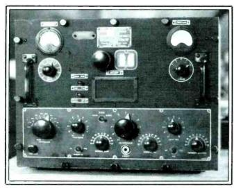
Like to DX on those low frequencies? This WWIIU.S. Navy RAL-7 TRF receiver tunes down to 15 kHz and really pulls 'em in from far away. It weighs a ton and is filled with cast aluminum and ceramics. Thanks to Fred Gwyer, M.D., W9BIU, of La Grange, IL for giving us a look at this great old veteran that still performs like a champ.
