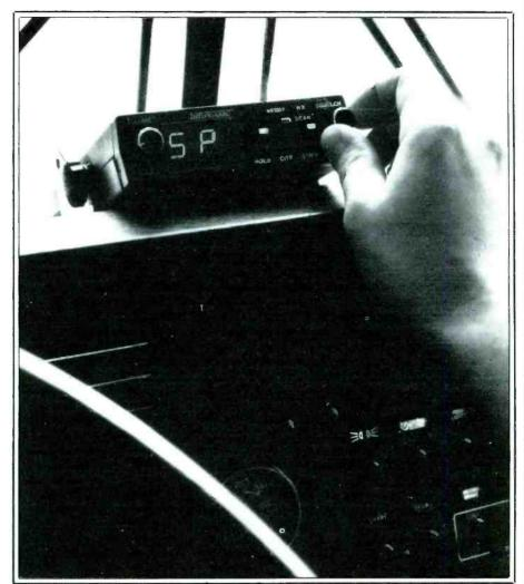
The Regency Informant scanner looks more like a radar detector (explain that to a cop) but is preprogrammed with local, state and national police frequencies for all 50 states. As you travel into a different state, the dial is adjusted so frequencies for that state can be received. TurboScan technology enables the radio to scan 50 channels per second!
