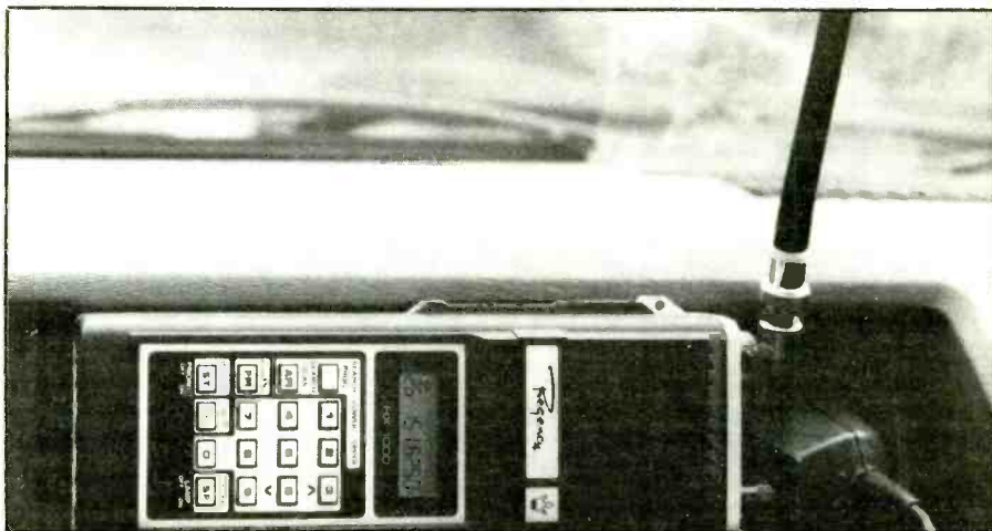
Here's the scanner installation in your columnist's car. The Regency HX1000 sits on the dashboard ledge and an angle adapter adjusts the rubber duck so it is vertical. Excellent reception is obtained without an outside antenna. (Photo by Chuck Gysi, N2DUP)
