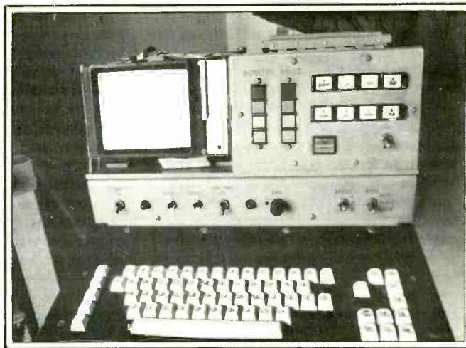
The "local copy unit" that puts the moving letters on the side of the blimp. (Photo by G. E. Glidewell)
