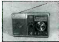
Panasonic RF-B300 Portable. Dual conversion FM/MW/SW; 1.6-30 MHz in 4 bands; LCD readout, LSB/USB/AM; wide/narrow sw.
