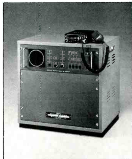
The IC-RP1210 repeater can be used with the IC-120 mobile transceiver, as shown.
