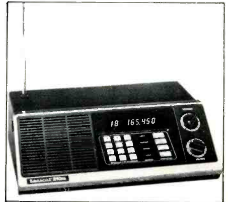
If you plan to monitor the Olympic Games, a scanner that can operate on AC from home or motel room or DC from the car, such as the Bearcat 210XL, is the best bet.
