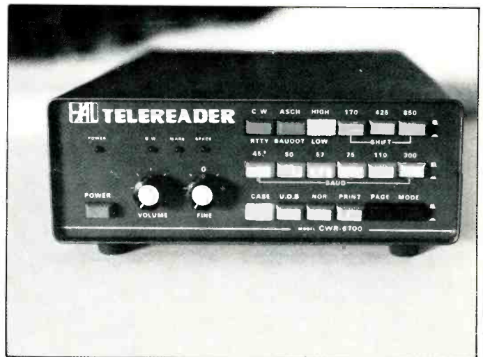
This is the HAL Telereader, a very useful device for those who wish to explore a wide variety of RTTY formats.
