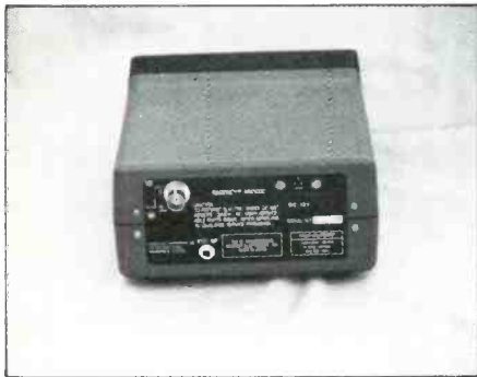
The rear deck of the MX-5000 is relatively simple and uncluttered. You may have to get used to the BNC antenna connector, though.
