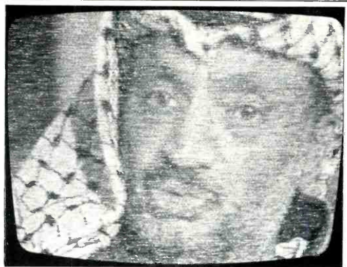
This photo illustrates the quality of reception when viewing occasional news feed transmission from INTELSAT global beam transponders while using a 20 foot dish antenna.
