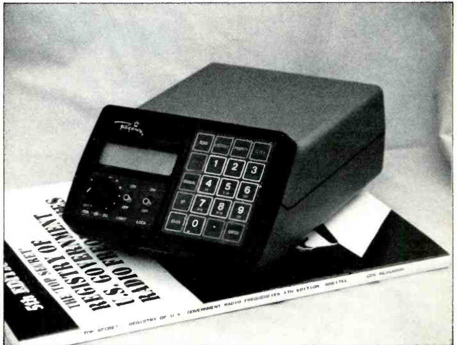
Regency's MX-5000 offers a chance to scan 200 to 400 MHz UHF aero band in addition to standard scanner frequencies.
