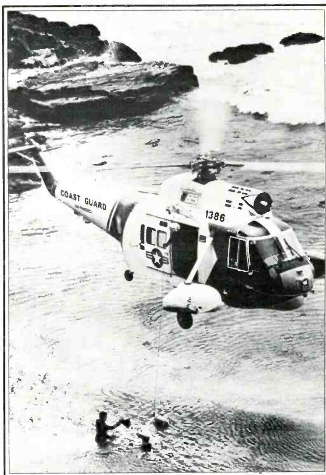
A type HH52A Sikorsky "SeaGuard" search and rescue helicopter as used by the Coast Guard.
