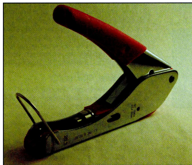
Photo B. This compression tool, required to attach the connectors, goes on sale at Harbor Freight Tools for about $15. It's not as flexible as more-expensive tools, but it gets the job done. (Internet screen grab)
