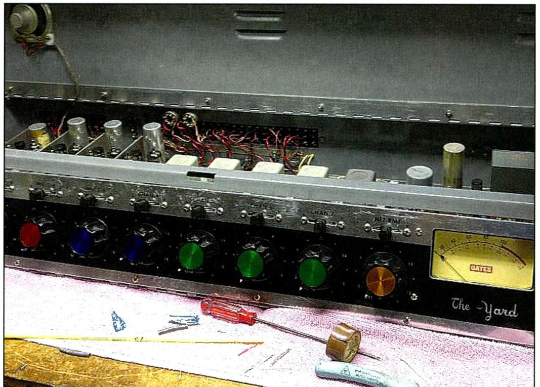
Photo A. Restoration of a classic Yard board in progress is shown here with the top opened. (Courtesy of Lane Lindstrom, “I Take Pictures of Transmitter Sites” Facebook group)
