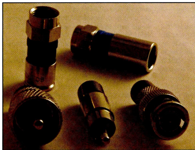
Photo A. Compression-style F connectors (back row) and a variety of Type-F adapters (PL-259, RCA, and BNC) transform RG-6 sat cable into whatever you need! (Courtesy of KPCØZZZ/NTØZ)
