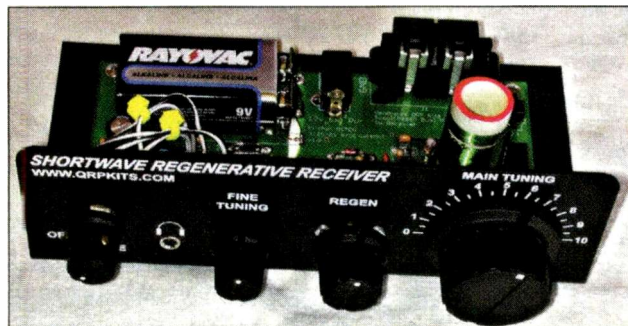
Photo A. The Hendricks ORP Kits Scout Regenerative Receiver is a handsome all solid-state kit designed for two coverage ranges: 3.3 to 5.1 MHz and 5.1 to 10+ MHz — perfect for shortwave AM and sideband monitoring, as well as "reading the mail" on some popular amateur bands. (Photography by KPC6PC)
