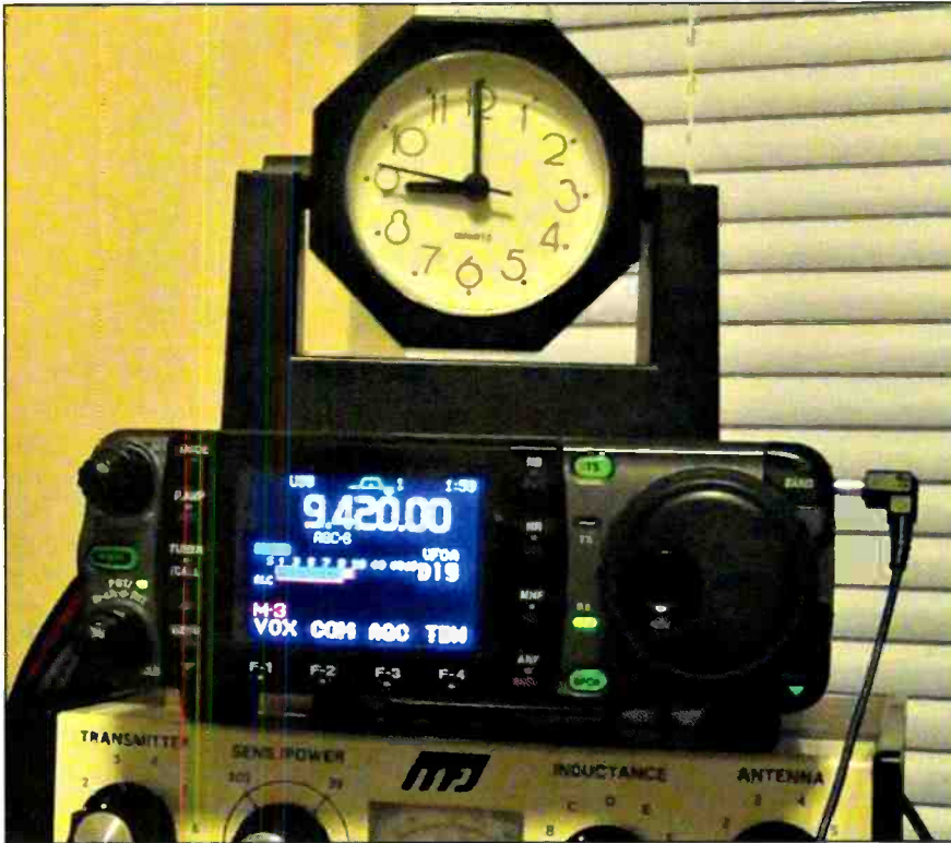
Photo C. Tuned to 9.420 MHz, WPC7USA's ICOM IC-7000 is shown atop an MFJ 940B Versa Tuner II at his listening post. (Internet screen grab)
