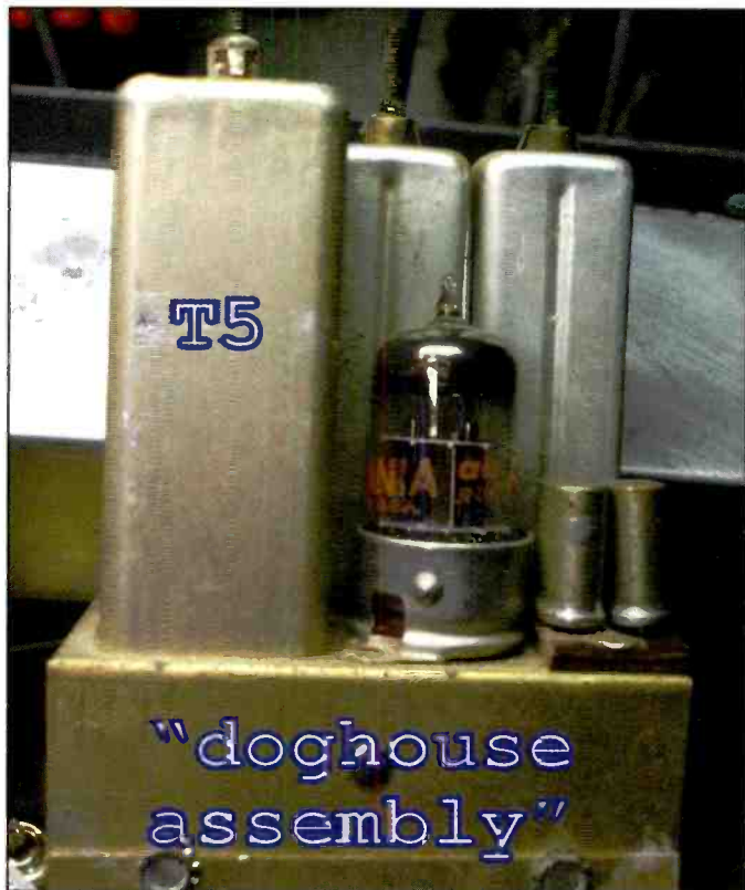
Photo B. Earlier versions of the doghouse used sockets to hold the 1600- and 1700-kHz crystals. Note the tuning slug lead screw for T5 is present on this unit.
