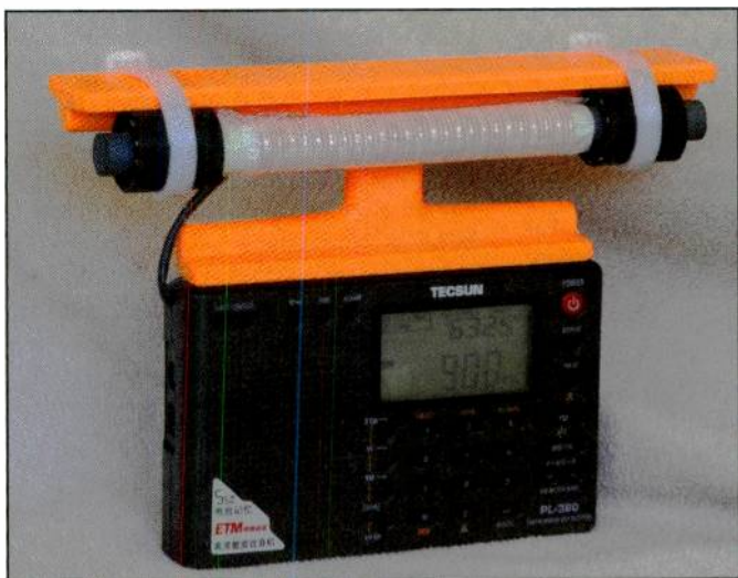
Photo A. The Tecsun PL-380 "hot-rodded" with an external 7-inch ferrite loop antenna by Gary DeBock for optimal performance. (Courtesy of WPC1CAT)
