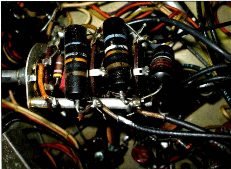
Photo F. The Selectivity switch determines the amount of coupling and the Q of the two 50.75-kHz IF transformers. Switching in different resistors and capacitors for each selectivity position does this. The original bumblebee capacitors should be replaced due to their high failure rates. The original carbon composition resistors were replaced with stable carbon film resistors.
