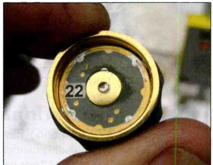
Photo C. A close-up of a ticker-tag shows it's about the size of a quarter. It is seen here with the battery removed.
