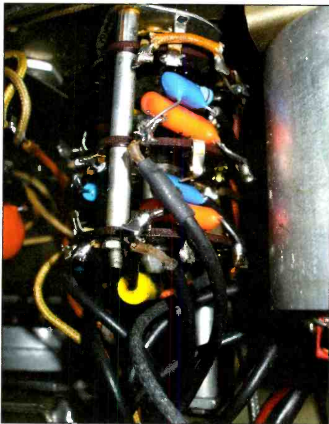
Photos G and H. These pictures show the replacement parts installed on the selectivity switch. Be very careful when de-soldering and removing the old components. The Phenolic wafer sections are easily damaged!
