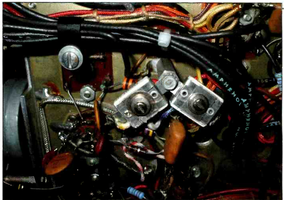
Photo E. Once the correct value for the compression mica was determined; I installed two compression mica capacitors under the chassis. These are used to set the injection level for the 1700- and 1600-kHz oscillators. As previously mentioned, this was supposed to be a temporary fix, but it works well and I may leave it alone.
