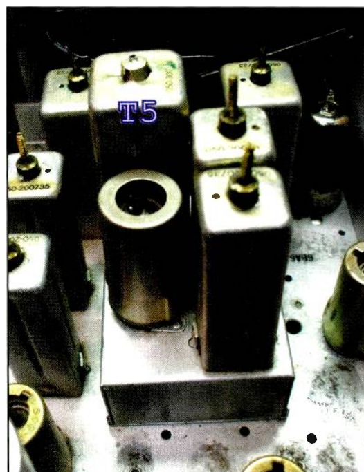
Photo A. The doghouse is the small sub-chassis that houses the second conversion oscillator (12AT7 tube) and the second converter stage (6BA6 tube). Transformer T5, marked on the photo, has two adjustments to set the 1600- and 1700-kHz crystal oscillator injection levels. The upper slug was damaged on this unit. The second slug is accessed through a hole in the main SX-101A chassis. The other two smaller transformers are the 50.75-kHz first IF transformer. (Photography by K1ZJH)
