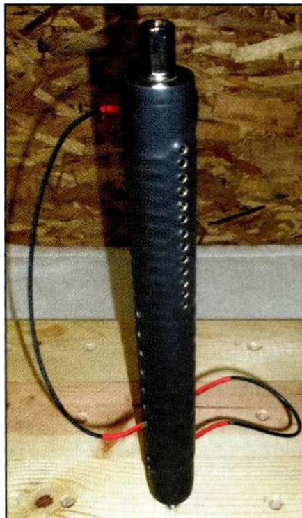
Photo F. More than 390 inductance tap combinations are possible with "The Great Lakes 392HF All-Bander" mobile antenna. (Courtesy of WB6NOA)
