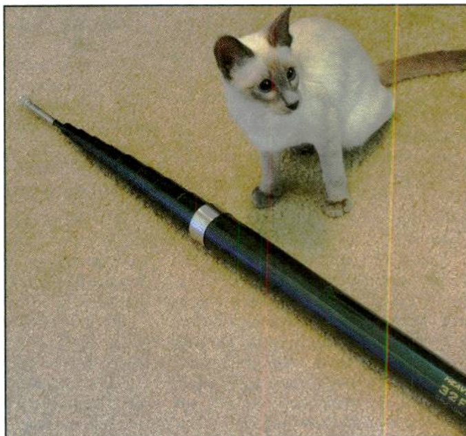
Photo B. The 32-foot, heavy-duty telescopic windsock pole when fully collapsed measures only 46 inches long, receiving the approval of Aurora , the DX Cat. (Courtesy of WPC1CAT)
