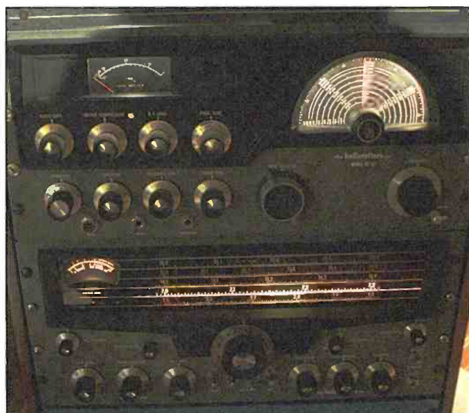
Photo F. Operating at night, by the glow of those vintage dials, is mesmerizing! Note the single-band illumination on the SX-101A dial! The receiver band switch controls the appropriate dial lamps to be lit depending on the band that is selected.
