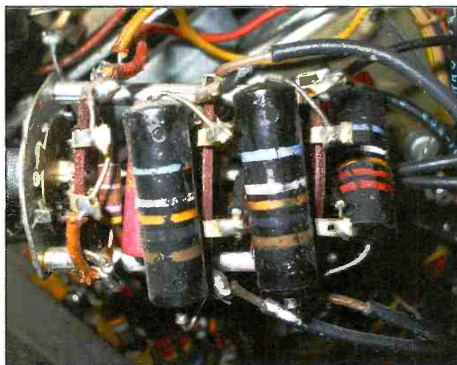
Photo H. These Black Beauty capacitors are part of the selectivity switch assembly and are used to control the degree of coupling between windings in a transformer in the 50.75-Hz IF section. The degree of coupling sets the receiver bandwidth. At the sharper positions, the receiver is capable of single-signal SSB reception, and good single-signal CW reception with decent selectivity.
