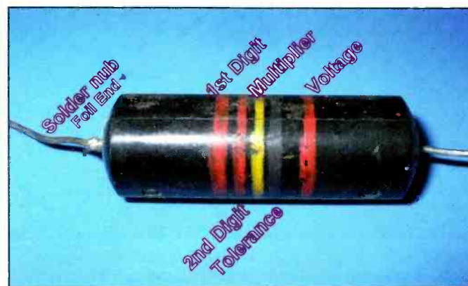
Photo J. This annotated photo of a Black Beauty capacitor shows the method to read its color band coding.
