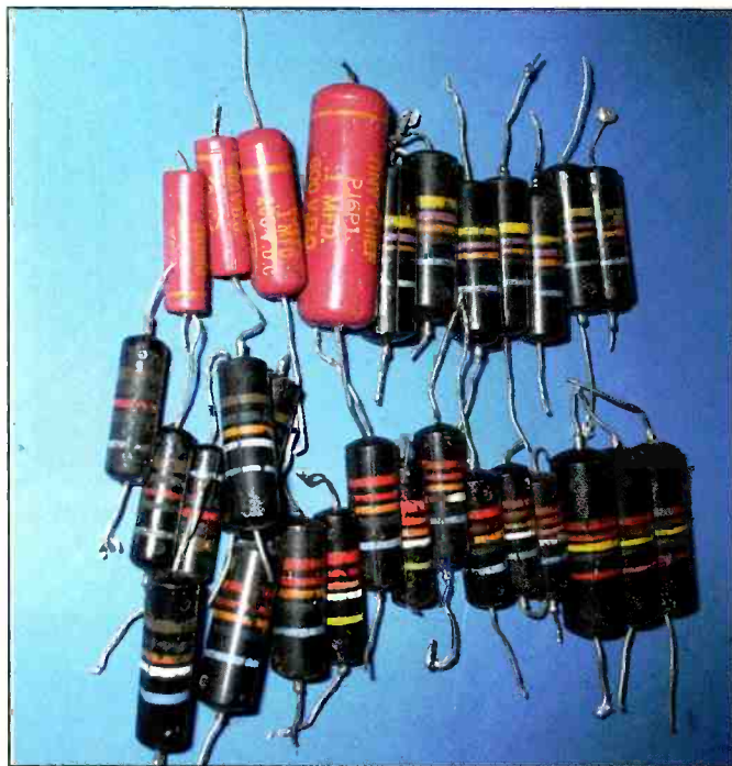
Photo I. These are the Black Beauty and Tiny Chief molded capacitors that were removed from the SX-101A during restoration.
