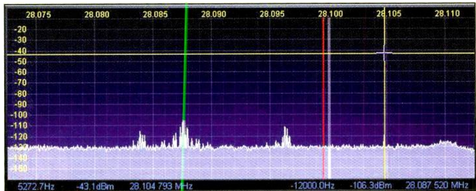
Photo B. Ten meters is open at last! Oops. Every blip on this “middle of the night” spectrum scan is digital crud from nearby PCs, TVs and so on, including the spikes at the left and the less distinct bulge at the right. (Courtesy of NTØZ)
