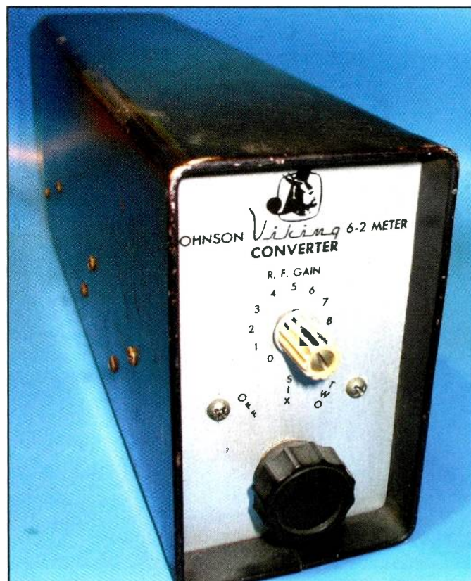
Photo D. A few early ham receivers, such as the National NC-300 and the Hallicrafters SX-101A, provided calibrated bands for the 6- and 2-meter VHF operator. Reception required the use of outboard converters. The Johnson 6N2 converter covers both bands in a single, small enclosure.
