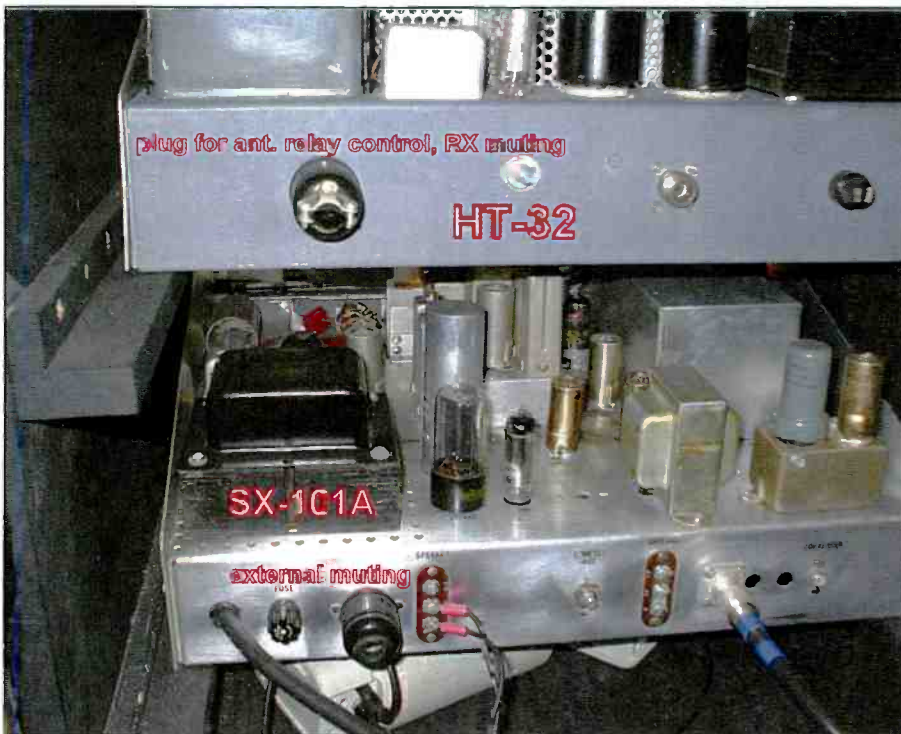
Photo C. Early separates, individual receiver and transmitters, had to be paired to operate properly. Going to transmit required an external antenna relay to transfer the antenna between the receiver and transmitter. Other relay contacts were used to mute the receiver while transmitting. Sockets for interconnecting the two units can be seen on the rear aprons of the receiver and transmitter. Plugs with cable caps are installed in the sockets.
