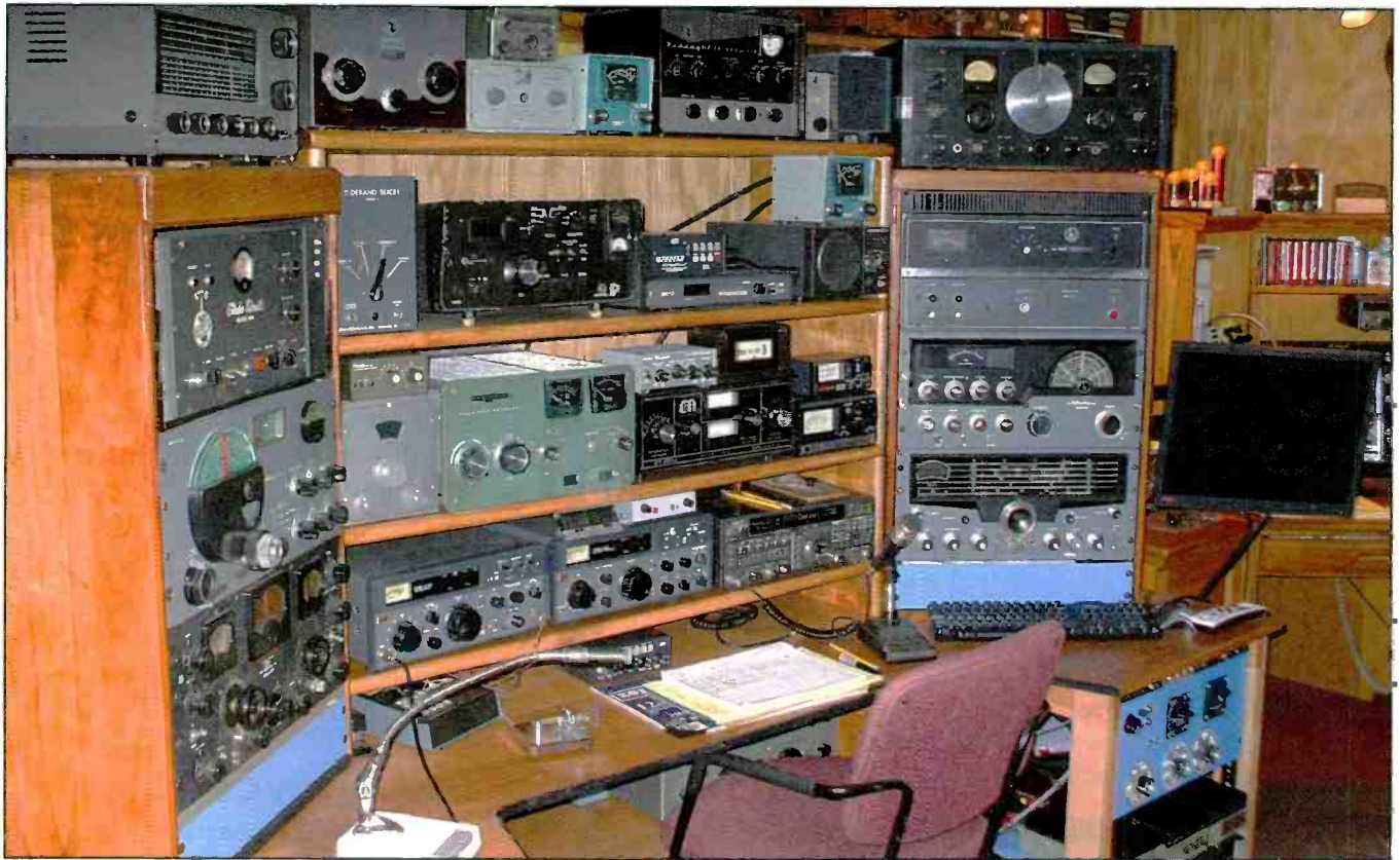
Photo B. My newly-constructed operating table includes two end consoles with 19-inch rack rails for mounting my vintage boat anchor gear.
