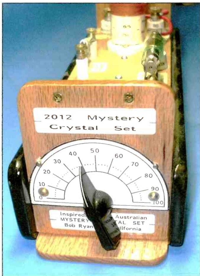
Photo D. Bob Ryan's eclectic version of the Australian Mystery Crystal Set . (Photography courtesy of Bob Ryan)
