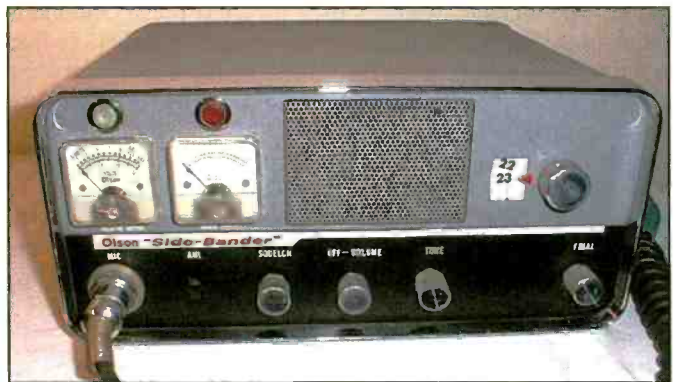
Photo J. The Olson Sidebander, circa early 1960s, was one of the early tube-SSB sets. (Courtesy of RetroCom.com)
