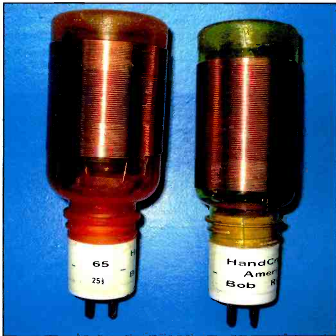
Photo G. Bob opted to use plug-in coils to increase the versatility of his Mystery Crystal Set . These are two fine examples of Bob's handiwork! While the original Mystery Set used cotton-covered wire, Bob used enamel magnet wire from the local RadioShack®.
