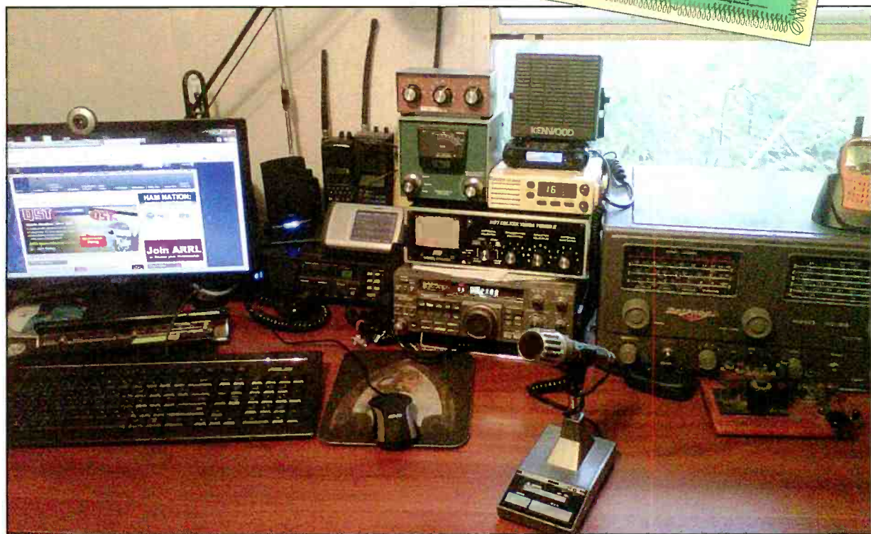
Photo A. The National NC-88 "World Master" general coverage receiver John Murphy, KPCØJPO, got for Christmas in 1967 is visible in the lower right of this picture of his New Town, North Dakota listening post. (Courtesy of KPCØJPO)
