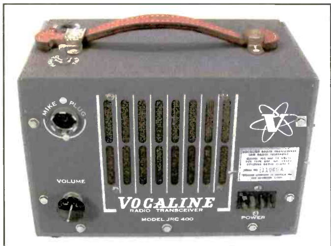
Photo I. The Vocaline JRC-400 was an early Class B 460-MHz CB. (Courtesy of CBTricks.com)
