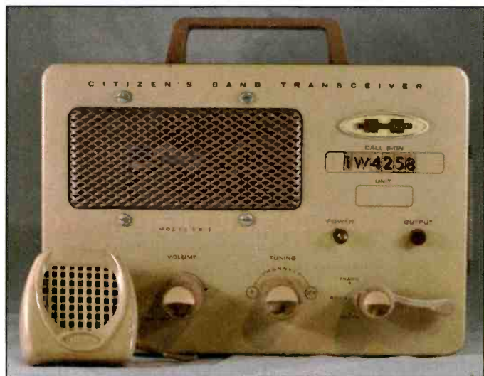
Photo E. The Heathkit CB-1 single-channel Citizens Band transceiver was part of the company's "Benton Harbor Lunchbox" series. Heathkit was based in Benton Harbor, Michigan and the shape of the radio's case certainly looked as though a sandwich, Twinkie® and thermos of milk might be inside. (Courtesy of Mark Haverstock)
