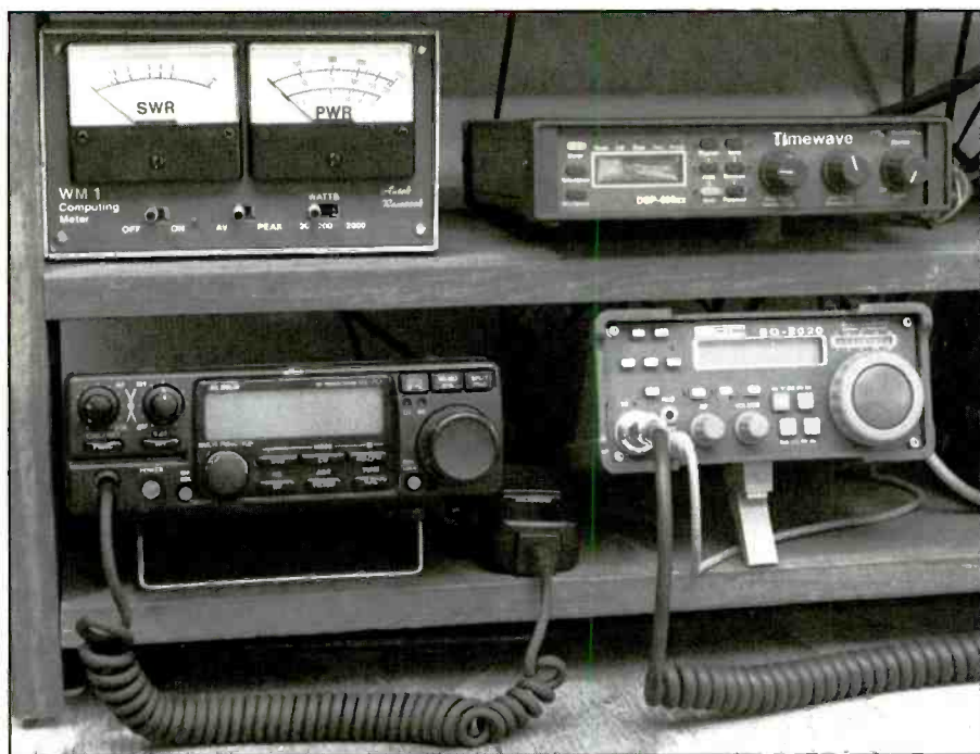
Photo B. My trusty Alinco DX-70, shown at the lower left, made my first "summer of 6-meter fun" — circa 2000 — a practical reality. An early "HF + 6" transceiver, the DX-70 was available in versions that put out 10 or 100 watts on 6 meters. Although not in Alinco's lineup for years now, used DX-70s are available for approximately $450 — which is more than they were selling for a couple of years ago! — NTØZ. (Courtesy of NTØZ)
