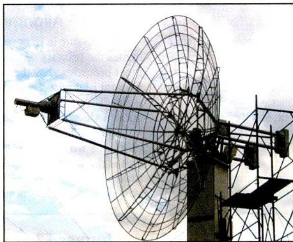
Photo A. Having come a long way since the early days of moonbounce radio communications, many radio amateurs around the world today use EME to communicate regularly. This 6-meter diameter parabolic reflector was built and used by Salvatore Gerloni, I2FZX, of Milano, Italy. (Courtesy of Spamhog via Wikimedia Commons)
