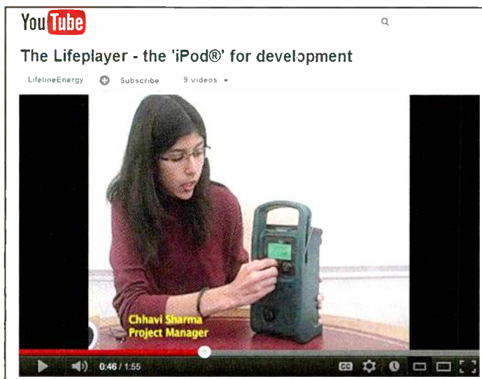
Photo A. The Lifeplayer , developed by Lifeline Energy, is a solar-powered, wind-up device that combines AM/FM/SW radio with an MP3 player. (Internet screen grab, < http://bit.ly/HcJwsY >)
