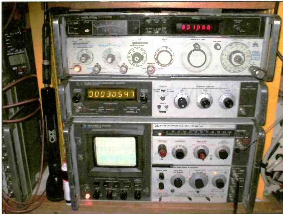
Photo B. Although far from necessary, heavy-duty test gear can save time and eliminate guesswork. In this photo, the author's HP-8640B signal generator, along with a HP-141T spectrum analyzer and companion HP-8443A tracking generator are being used to visually verify that the Mohican local oscillator is correctly tracking on Band E.
