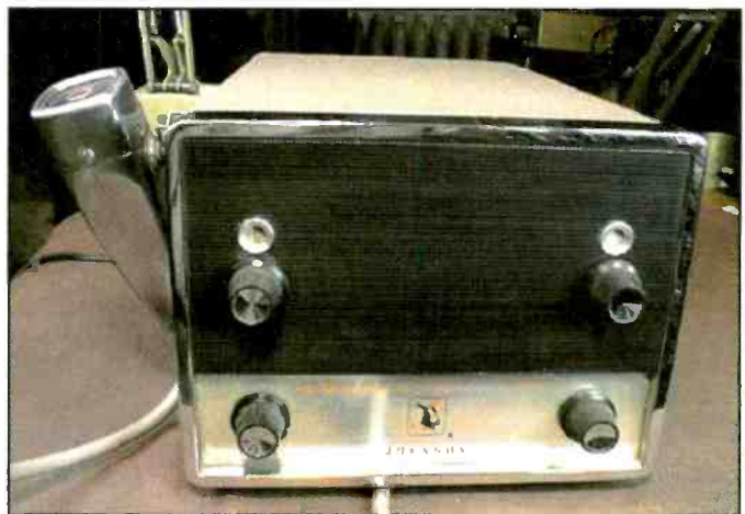
Photo D. Here's the classic Johnson Messenger 2 CB. Take a video tour of the transceiver in action at: < http://bit.ly/ApEO31 >. (Courtesy of RetroCom.com)
