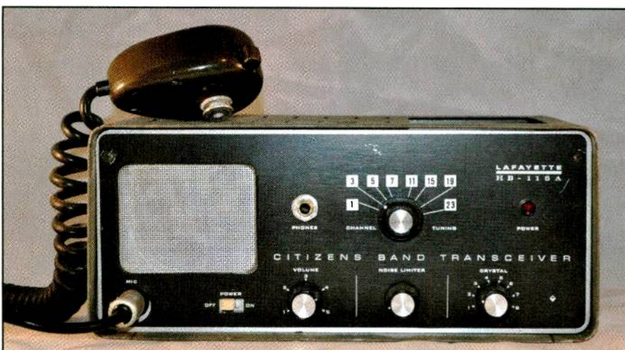
Photo G. The Lafayette HB-115 was writer Mark Haverstock’s first CB rig. It featured eight channels with a tunable receiver. (Courtesy of Mark Haverstock)
