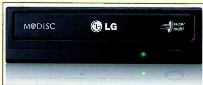
Photo B. LG's GH22NS90 optical recorder can read and write CDs, DVDs and the new M-disc archival DVDs. One of several drives that can handle the new archival discs, this low-cost model is available online for less than $25. (Courtesy of NTOZ)
