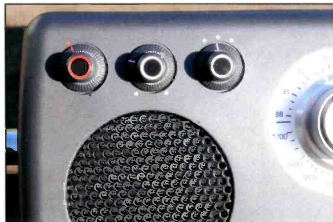
Photo D. These knobs on the CC Gonzo control on/off, volume, bass response, and band selection.
