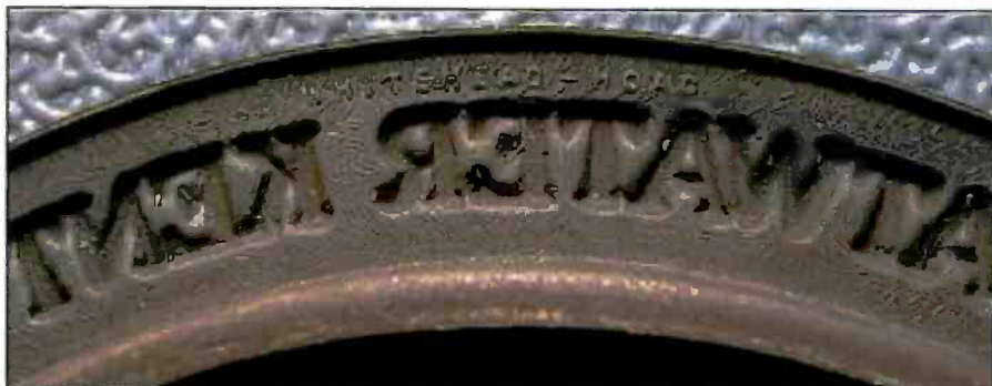
Photo D. A close examination of parts in the 206-X shows the care and quality that went into the manufacture of this radio. "Whitehead-Hoag" — barely visible in this stamped metal piece — "was a major stamper of small metal parts, especially campaign buttons back to the 1890s. So, Atwater Kent indeed outsourced the stamping of these dials, contrary to the urban myth that this brand built every part in house!" writes radio expert Pete Olin.
