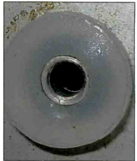
Photo L. A new set of washers was made using silicone caulk. "This material has precisely the right properties to be used in this application," Mornhinweg says. "Using my lathe, I turned some molds from polyethylene, which does not adhere to silicone. Then it was just a matter of pouring silicone, letting it set, take the new washer out of the mold, and pour silicone again. In a matter of some days, I made all the washers I will ever need!"
