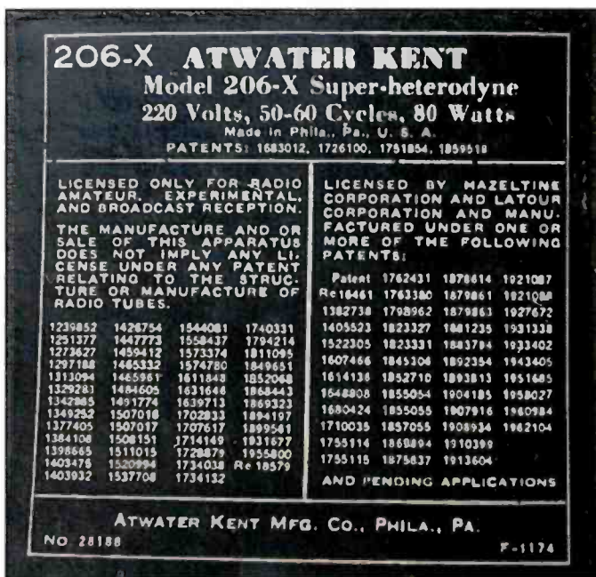
Photo B. An inscribed metal label on the inside of the radio shows it to be Atwater Kent's model 206-X — with the "X" indicating the receiver was an export version, made for 220-volt AC mains power distribution.
