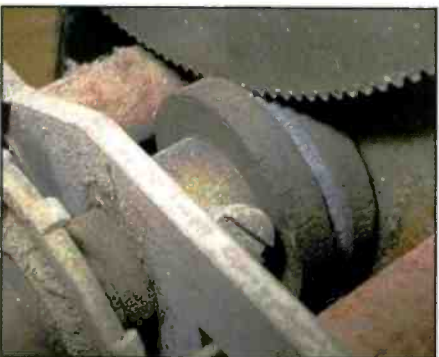
Photo I. The drive mechanism of the variable capacitor was worn and useless. "There is a vernier drive with a rubber roller connecting to a softly dented wheel," Mornhinweg writes. "This roller was dry, brittle and worn — so much so that it slipped without even trying to engage with the teeth."
