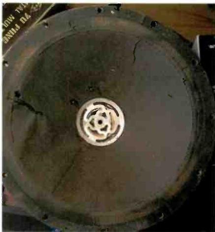
Photo P. "The voice coil was bent, and always scraped at some place, regardless of how I pushed and shifted it," Mornhinweg recalled. "The coil was non-original. The cone had several patched rips, and some unpatched ones. The spider was totally deformed, ending up in a position that left it no motion range. After pondering the possibilities, I decided, with quite some pain in my poor suffering heart, to part with the original Atwater Kent cone, and re-cone this speaker."
