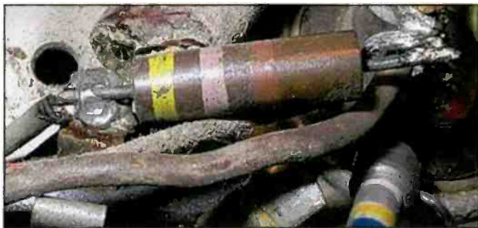
Photo F. Atwater Kent had its own parts coding system, which confused many people attempting to restore its radios. For example, here's a poorly-soldered resistor. It is non-original and 470 ohms. The original was 20K. Nobody who didn't have access to AK literature stood a chance in understanding the company's unconventional resistor color-coding scheme.
