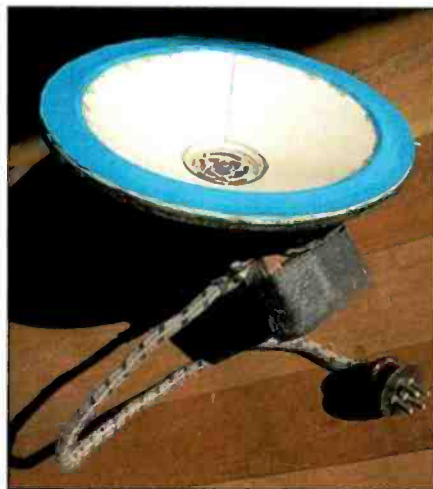
Photo R. Voila — the rebuilt speaker! "Shudder, those colors!" Mornhinweg said. "Originally I had the noble intention of spraying it black, but then I decided against this. The paint might stiffen the cone, making it sound tinny. Anyway, these colors aren't visible when the radio is assembled."
