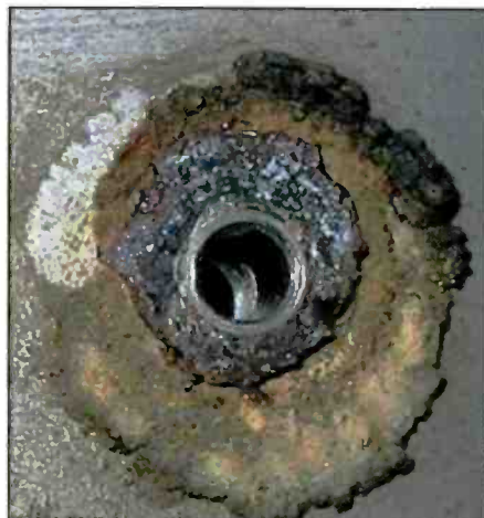
Photo K. Soft, slotted rubber washers that were commonly used in almost all radios of the time "had decomposed into a somewhat-crystallized, rosin-like goo," he says. "I could find no rubber that's soft enough for this purpose." The washers were used to minimize chassis vibration's effect on the variable capacitor.
