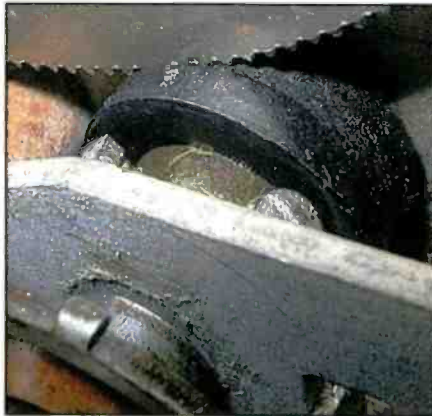
Photo J. A custom-made drive mechanism replacement was crafted from a door stopper — the kind you find at home improvement stores. "Several people who have seen it just don't want to believe that this part isn't an original Atwater Kent spare part!" Mornhinweg says.
