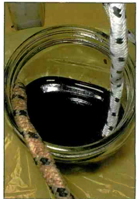
Photo M. The unrestored Atwater Kent 206-X's original power cord had been replaced with one made of plastic from the 1960s. "Ugly," Mornhinweg says. Reverting to a cloth-covered power cord meant buying a length colored white with black dots and dyeing it with walnut extract.
