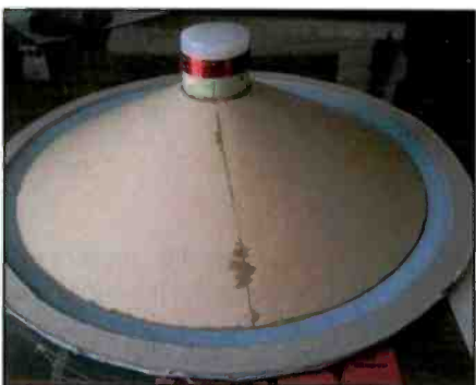
Photo Q. "I made the cone from the same stiff paper I use to print my business cards," he said. "I made a polyethylene former for the voice coil, using the lathe, and made the coil, using an old QSL card as material for the support."
