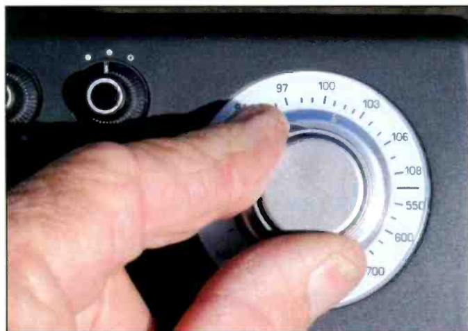
Photo C. The CC Gozo tuning knob is free of backlash, but a little stiff on a cold morning. C. Crane says the stiffness is by design (see text). The dial lights up when adjusted — very clever!
