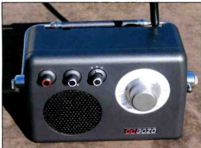
Photo B. The C. Crane CC Gozo is a compact AM/FM portable radio with analog-style turning, plus a jack to patch-in a personal stereo device, such as an iPod.
