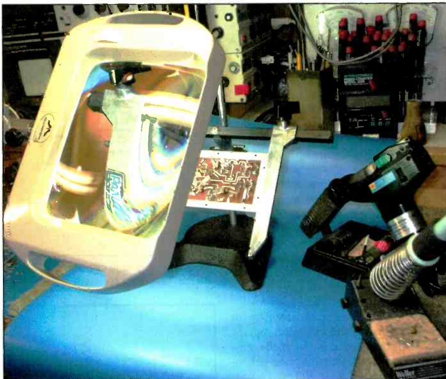
Photo B. A large magnifying lamp and a good soldering iron are essential.
