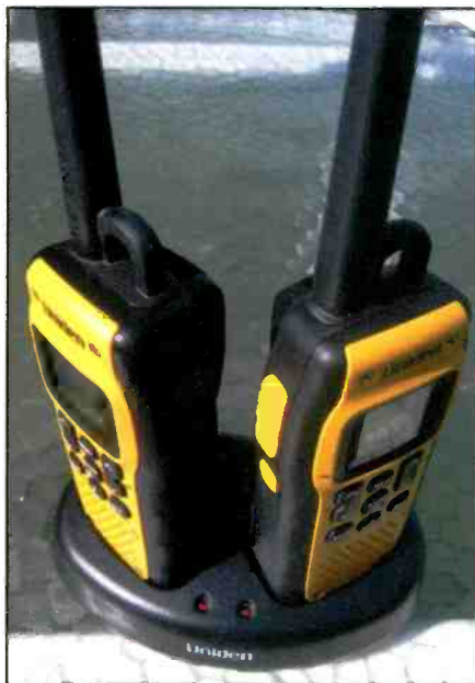
Photo F. These Uniden FRS radios charge in their two cup holders, in about three hours.
