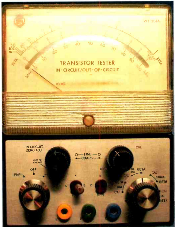
Photo E. The RCA WT-501A transistor tester will test transistors in or out of circuit.
