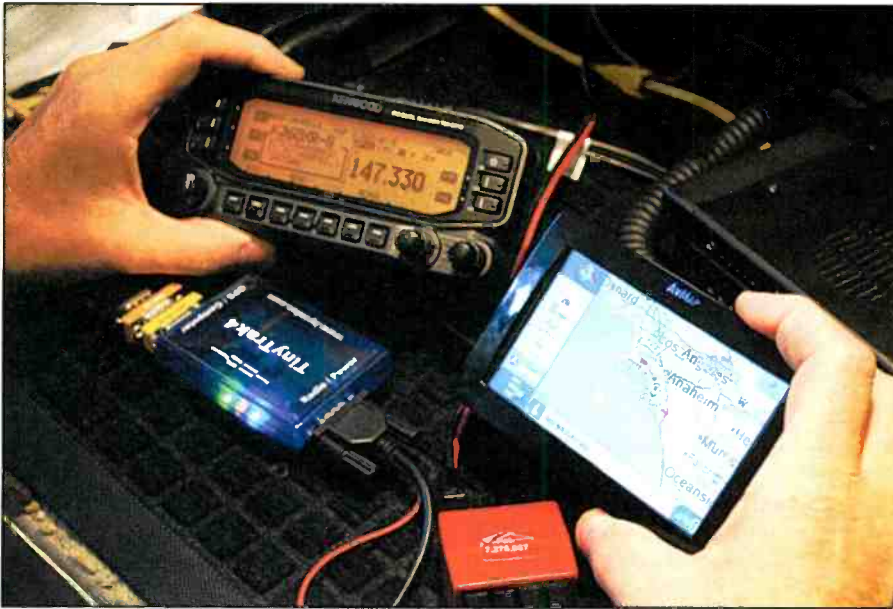
Photo B. The Automatic Position Reporting System (APRS) and a radio amateur location “reader” help FRS operators see the hams around them on the screen.
