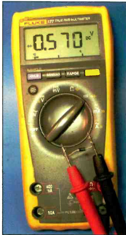
Figure 3. Transistor junctions act like back-to-back diodes, and can be tested on a digital ohmmeter.
