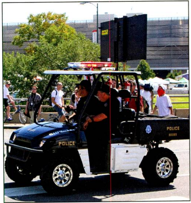
This little cart is used by Denver for public safety events and public relations. Note the traffic sign mounted on the roof that can display moving messages. (Courtesy of Jeffrey Beall)
