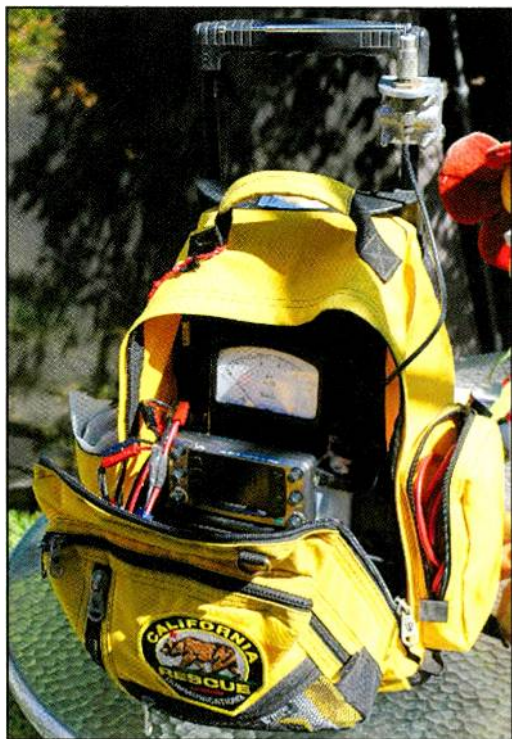
Photo A. Gordon West, WB6NOA, uses a roller bag for toting gear in a remote set up. Monitoring FRS channels is part of his emergency communications plan. On the amateur bands he uses an ICOM dual-bander. (All photographs courtesy of WB6NOA)
