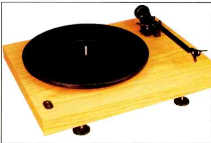
Photo C: The basic Moonbeam model turntable features a 24-pole AC synchronous motor and low-tension belt drive for vibration-free, no-drift, 33- and 45-rpm operation. (Courtesy of SOTA)
