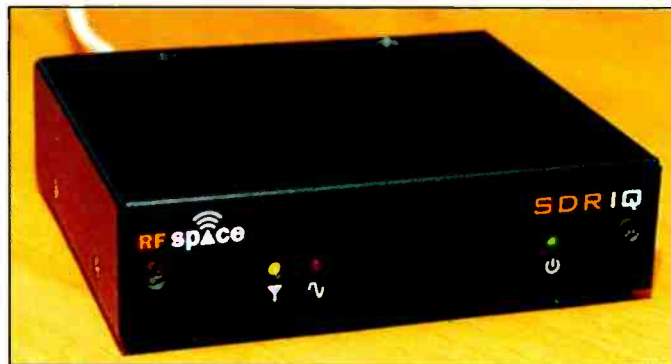
Photo B: The RFSpace SDR-IQ receiver can capture as much as 190 kHz of RF spectrum on your computer's hard drive. (Courtesy of RFSpace)
