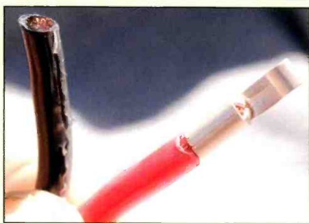
Step 1: Strip the wire and push on the Anderson power connector. (Courtesy of WB6NOA)
