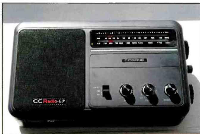
The C.Crane CCRadio-EP AM/FM slide rule radio has a hot front end and is VFO tuned. (Courtesy of WB6NOA)
