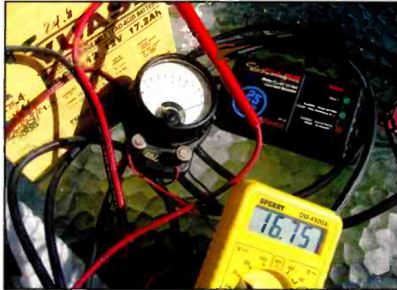
A pulse charger, battery and test gear help tell the story during testing. (Courtesy of WB6NOA)
