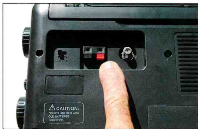
Want to add a long-wire AM antenna to your portable radio? Here's where you'd plug it into the C.Crane CCRadio-EP AM/FM slide rule radio. (Courtesy of WB6NOA)
