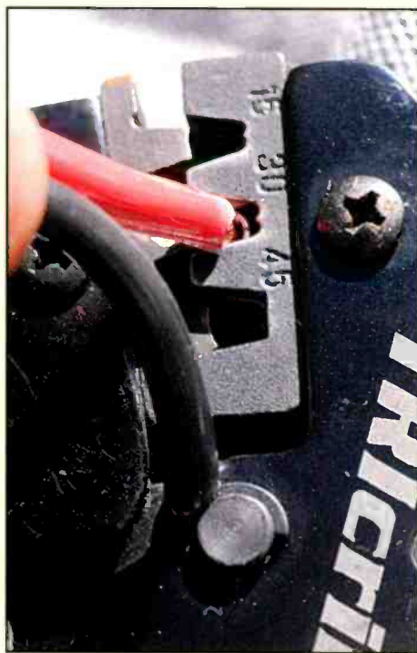
Step 2: Slip the connector into the crimper and squeeze hard. (Courtesy of WB6NOA)
