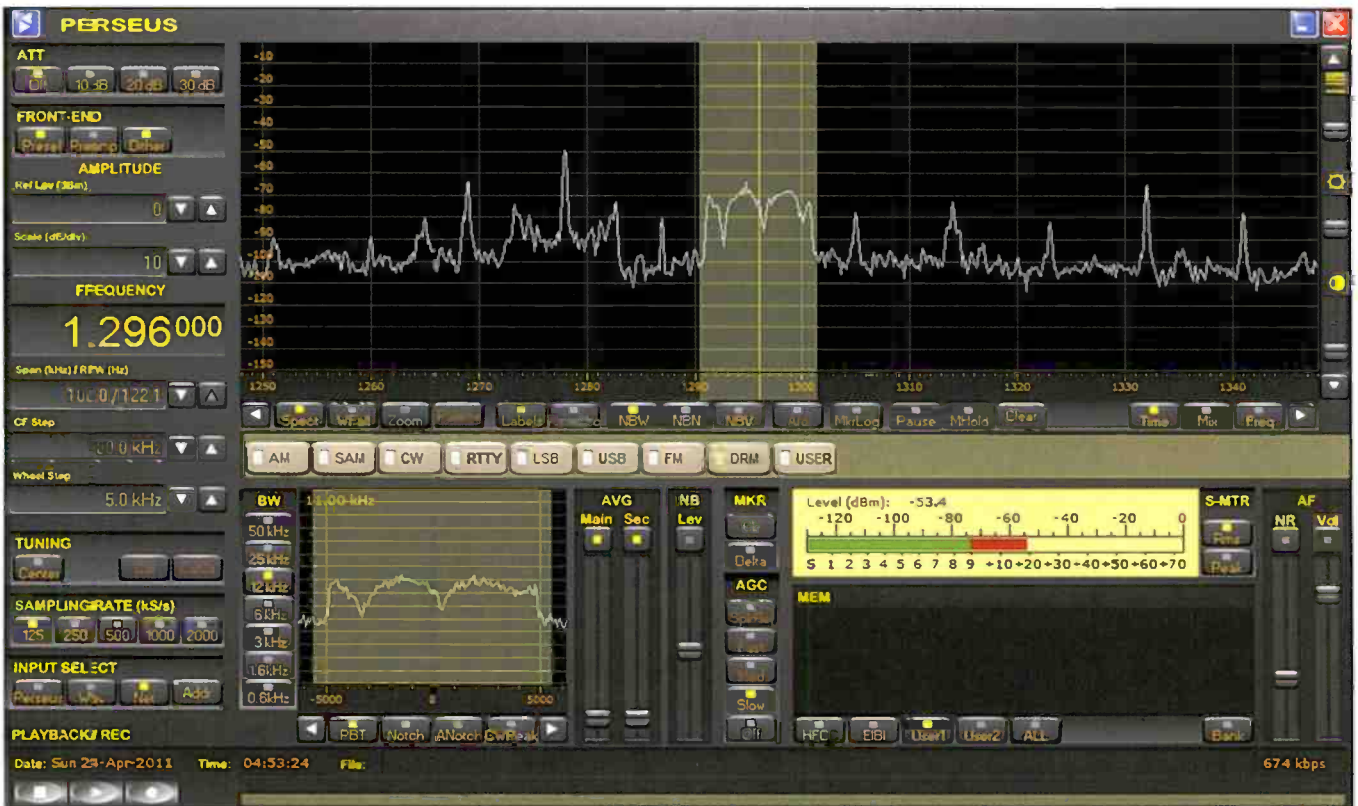
Figure 4: Note the "square" waveform of the DRM digital signal on 1296 kHz as opposed to the more "pointy" analog AM signals that surround it.
