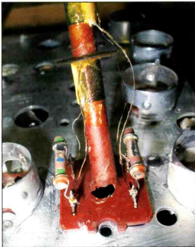
Photo B: Despite careful handling, I did have one “oops” experience when I damaged the 9-MHz IF transformer on the SSB generator. This added another several hours time to the restoration while a replacement was fabricated from junkbox parts.
