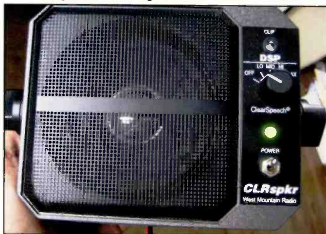
Photo C: The original West Mountain Radio CLRspkr®, above, offered four selectable DSP levels. The upgraded version, shown in Photo A , uses a potentiometer for setting DSP levels — infinitely adjustable for filtering levels.
