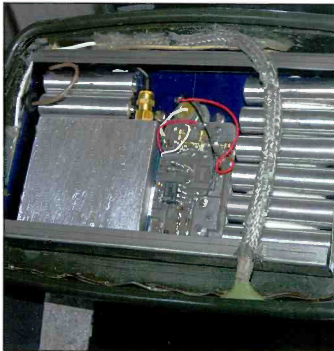
The concealed receiver-transmitter rearview mirror mounted in U.S. Army reconnaissance vehicles was used for emergency distress signals, if attacked.
