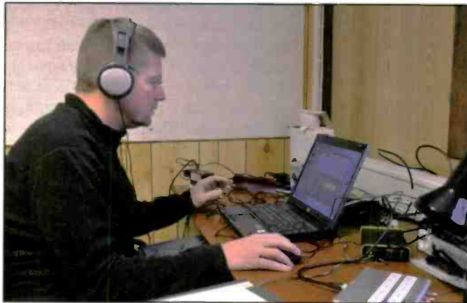
Jim Solatie listens for broadcast DX signals while capturing RF spectrum on a laptop computer connected to a Perseus software defined radio (SDR) receiver.
