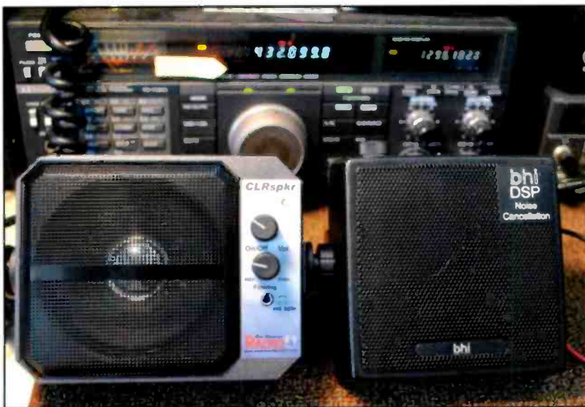
Photo A: The West Mountain Radio DSP CLRSpkr® speaker, left, and bhi DSP Noise Cancellation speaker each feature built-in audio amplification. (Photographs courtesy of WB6NOA)
