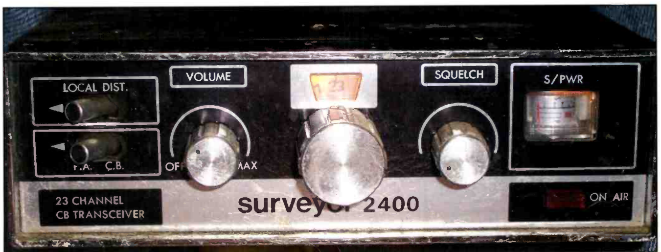
Photo A: A pre-1976 Surveyor 2400 Citizens Band transceiver — complete with 23 channels and lots of knobs and switches — when painstakingly configured serves as our example of a most primitive spread-spectrum communications system. (Courtesy of WA5VJB)
