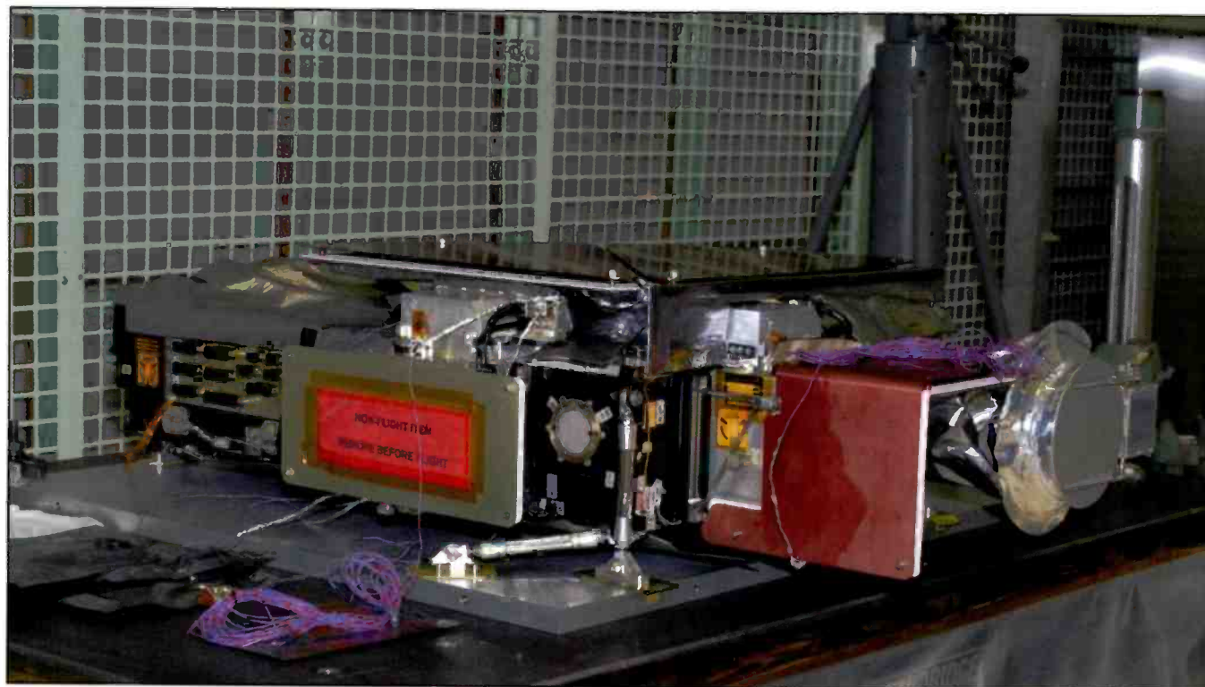
← Figure 1: The Helioseismic and Magnetic Imager (HMI) Instrument aboard the Solar Dynamics Observatory (SDO). HMI allows scientists to “hear” sunspots before they emerge on the visible solar disc. See text. (Courtesy of NASA/SDO)
