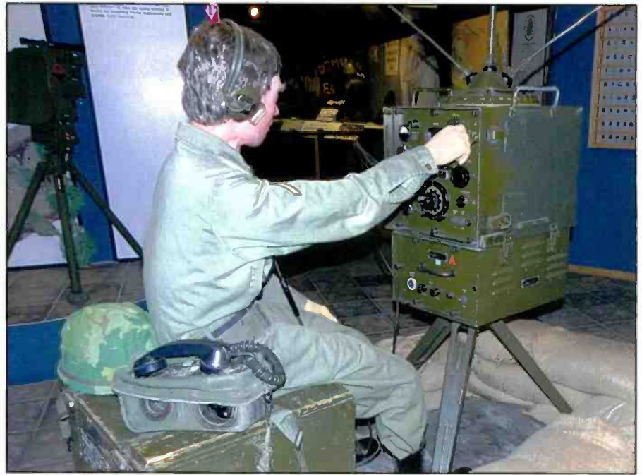
Here's a view of a soldier operating the ANPPS-5 Ground Surveillance Radar.
