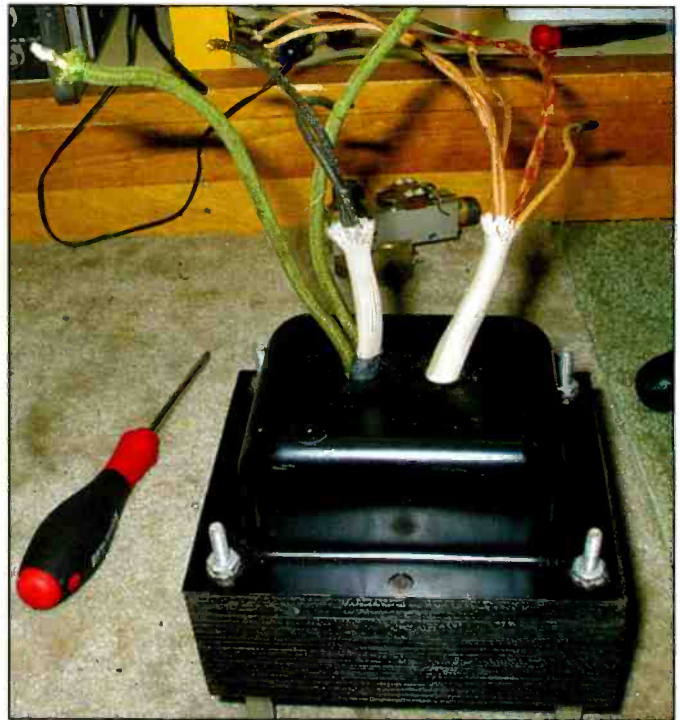
Photo B: Insulation was added to increase the voltage breakdown rating for the high-voltage secondary winding leads.
