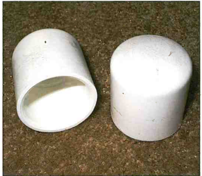
Photo E: The plumbing section of the local hardware yielded two PVC cover caps that were ideal for protective covers over the solid-state replacement rectifiers. They are hot-glued to the old tube base shells.
