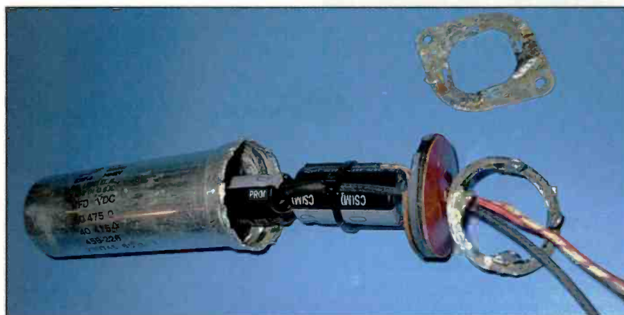
Photo K: The double-section, FP-style mount electrolytic metal can capacitor was gutted and rebuilt using new components.
