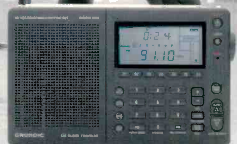
GLOBE TRAVELER G3 AM/FM/Shortwave Digital Radio with Aircraft Band, SSB (Single-Side Band), RDS (Radio Data System) and Synchron- ous Detector
