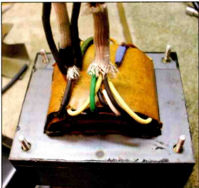
Photo A: The leads for 5-volt rectifier filament windings are insulated and taped off inside the transformer housing.
