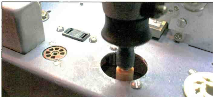
Photo G: A Dremel tool was used to enlarge the tube socket openings on the HT-32 chassis to accommodate higher-quality ceramic tube sockets.
