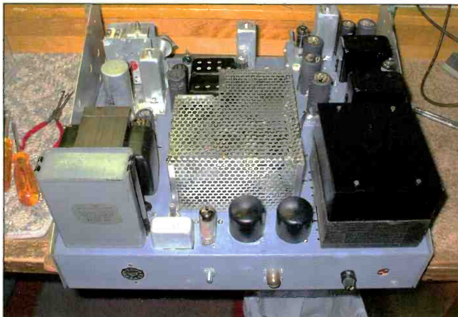
Photo H: Many of the larger power supply components are back in place after being cleaned and painted.
