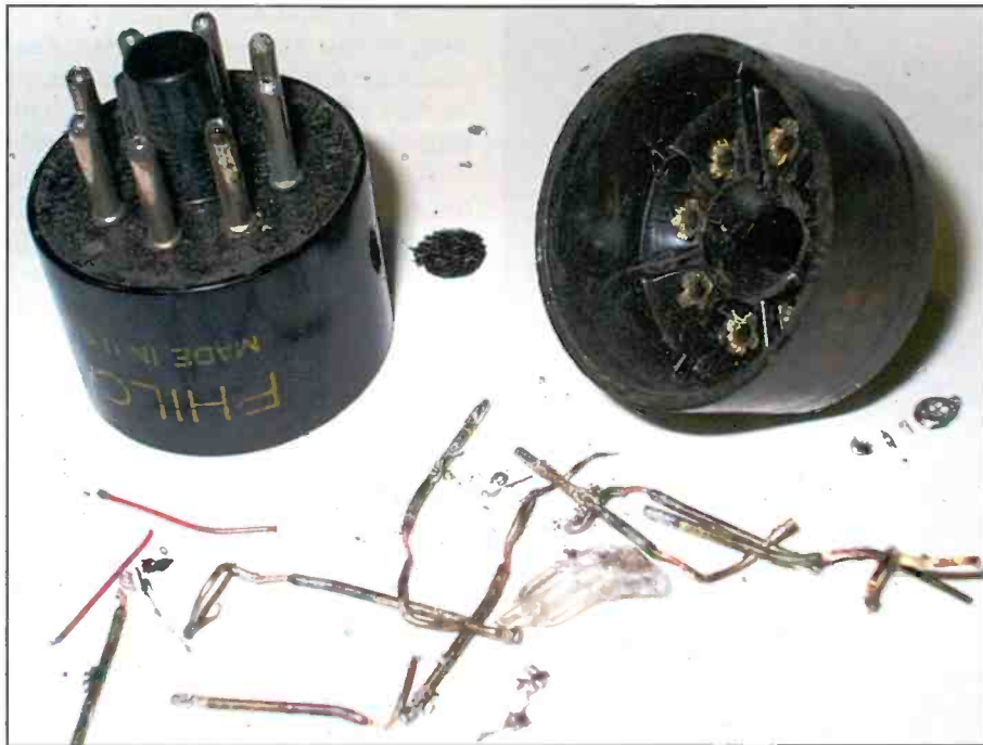
Photo C: The bases from two defective glass octal-based tubes were reclaimed to house the new solid-state rectifier replacements.
