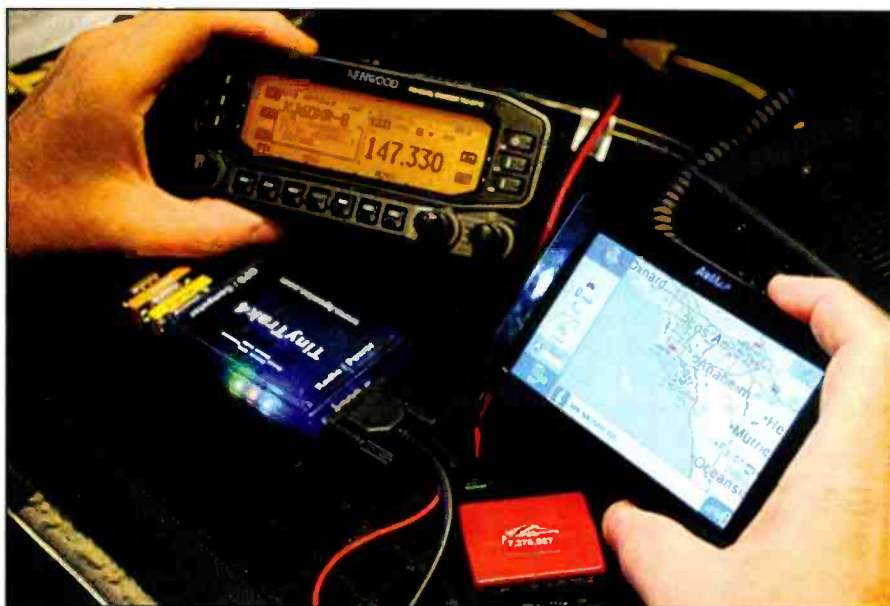
Kenwood mobile TM-D710, Byonics Tiny Trac 4, and AvMap G6, all tied together for APRS and the added texting feature.
