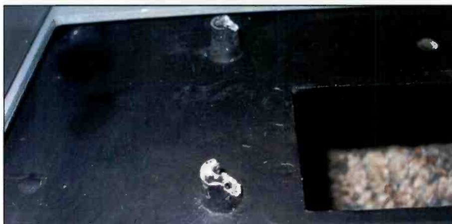
Photo H: These posts were drilled and tapped for 6-32 machine screws, but after five decades the metal has fatigued and fractured leaving few remaining threaded areas.
