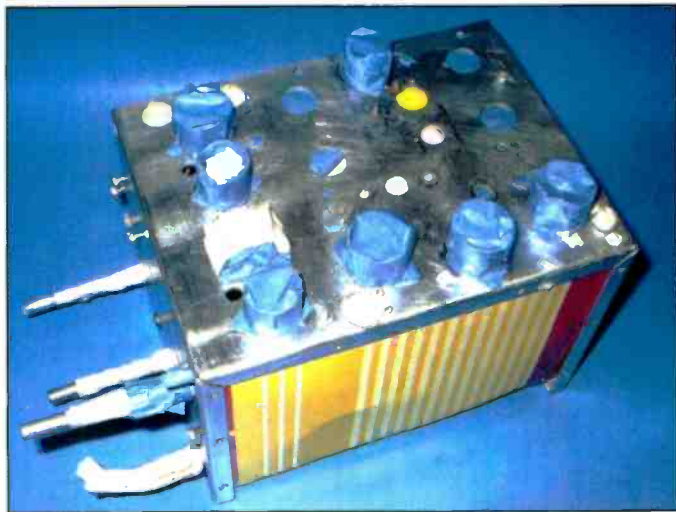
Photo B: The SSB Generator subchassis receives the same protective treatment as the main chassis before painting.
