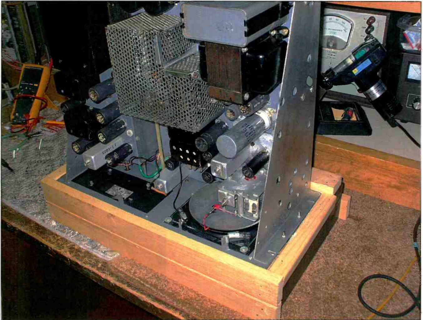
Photo L: Since I have several older Hallicrafters receivers and transmitters in the restoration queue, I came up with a simple chassis support jig. It provides stable support for the front panel and chassis without placing stress on the knobs or shafts.
