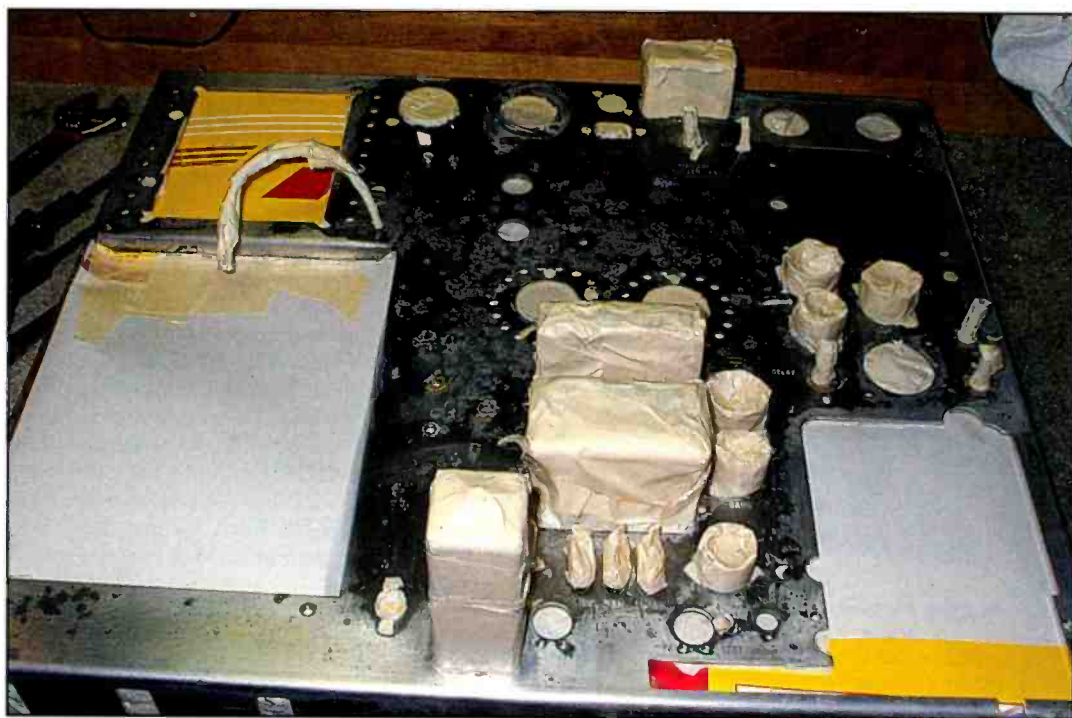
Photo A: Once the main chassis was stripped of the larger, removable assemblies, whatever remained that wasn't to be painted had to be protected. Even the rivet heads were carefully covered with masking tape, which was trimmed using an X-acto hobby knife. (All photographs courtesy of K1ZJH)
