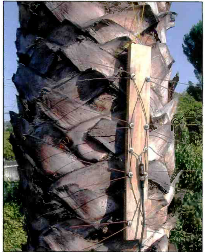
Photo A: This little homebrew DTV antenna's coat-hanger elements have turned rusty red, which helps it blend nicely into the side of a palm tree — and is barely visible from the ground. (Courtesy of K16SN)
