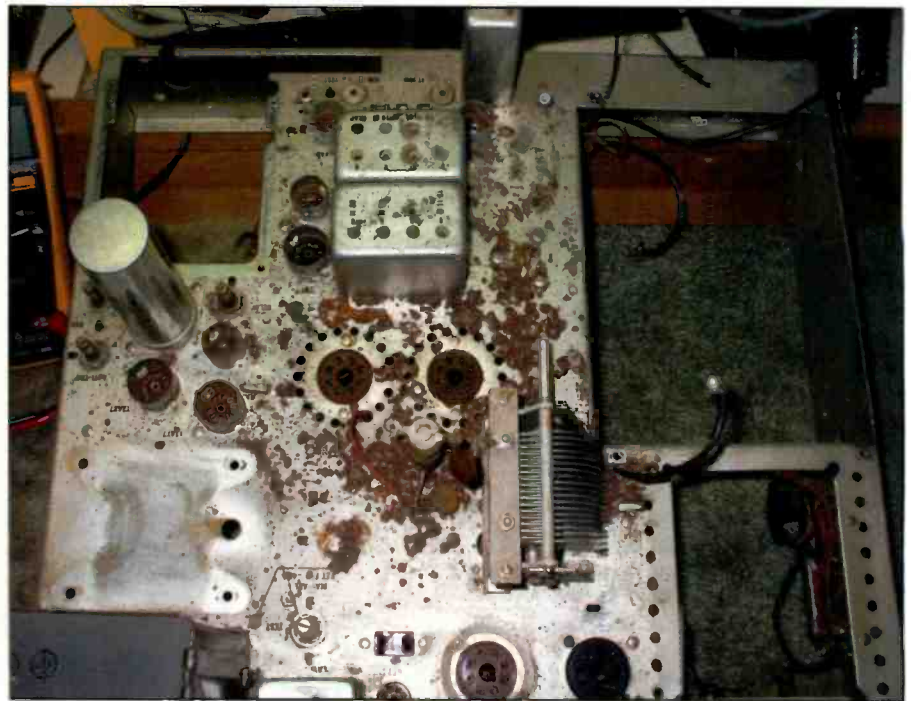
Photo F: Here's where we started! Once the major subassemblies, shields and transformers were removed, the extent of the rust damage was more evident.
