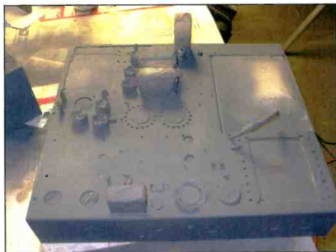
Photo C: Here's the main chassis, after three coats of gray primer. The metal surfaces must be clean to ensure good paint adhesion.
