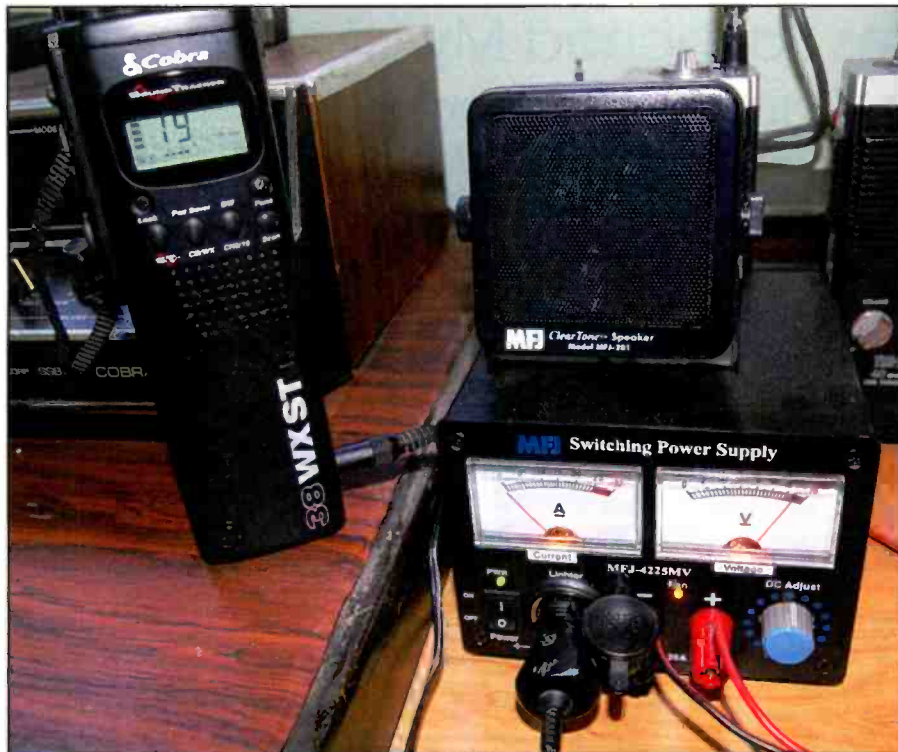
An MFJ-4225MV Voltage Switching Power Supply and MFJ-281 ClearTone Speaker serve as nice accessories to the Cobra 38WXST CB walkie-talkie.
