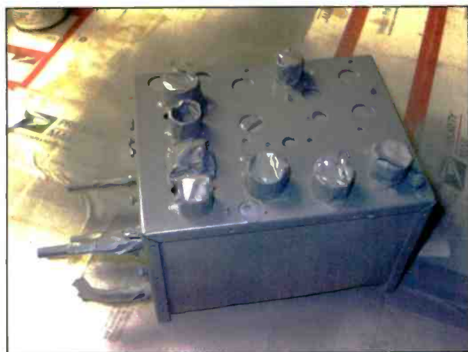
Photo D: After three coats of gray primer spray paint, the SSB Generator takes on a whole new look.
