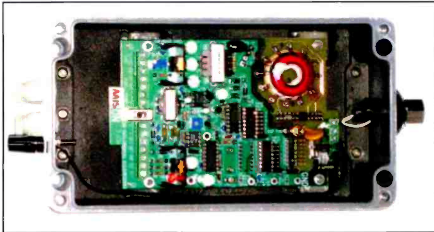
A look inside the Rangemaster AM1000 Part 15 transmitter. (Courtesy of Rangemaster)
