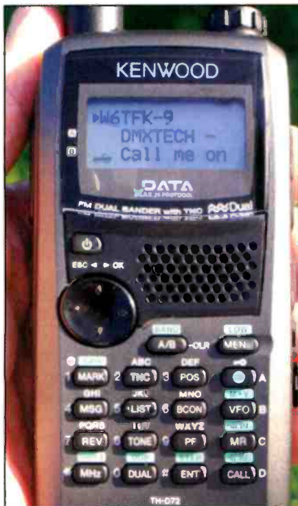
The Kenwood TH-D72 handheld plugs right in to the AvMap. Be sure and turn off the TH-D72’s built-in GPS, though, as the AvMap has GPS output.
