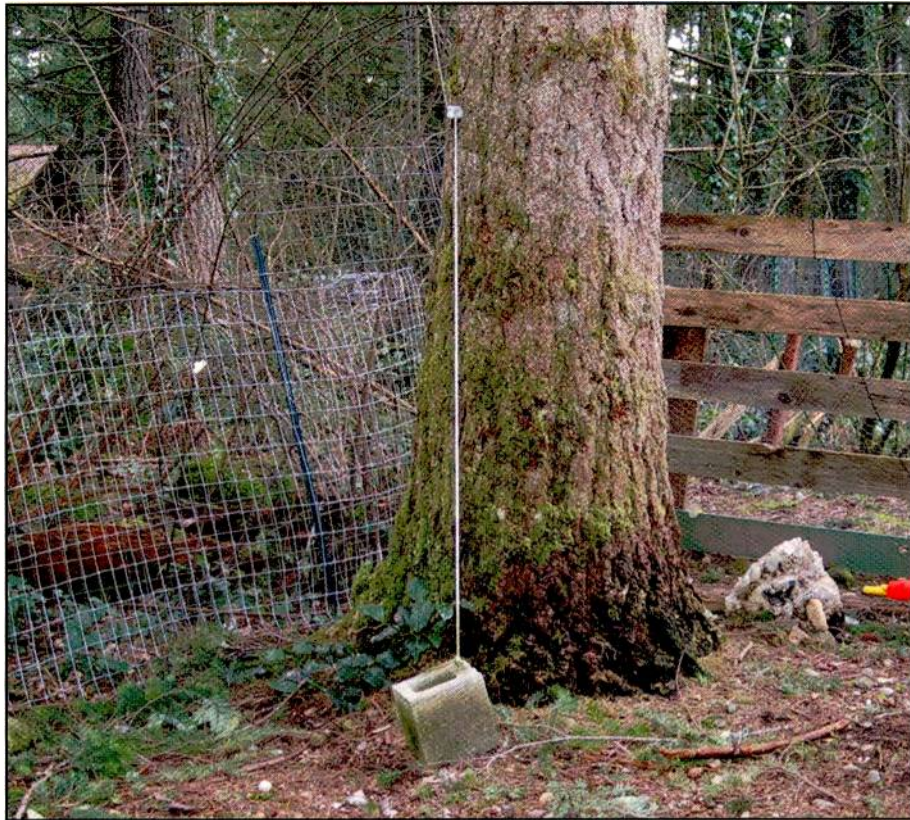
Concrete blocks are used to keep the loop antenna high in the air, while at the same time providing stress relief during high winds — when the trees are swaying.
