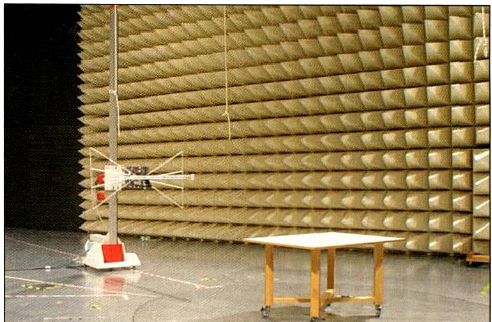
An anechoic chamber — or shielded room — can be used to prescreen a product for emissions that might otherwise be overwhelmed by ambient signals in the air. (Photographs courtesy of Bruce A. Conti)
