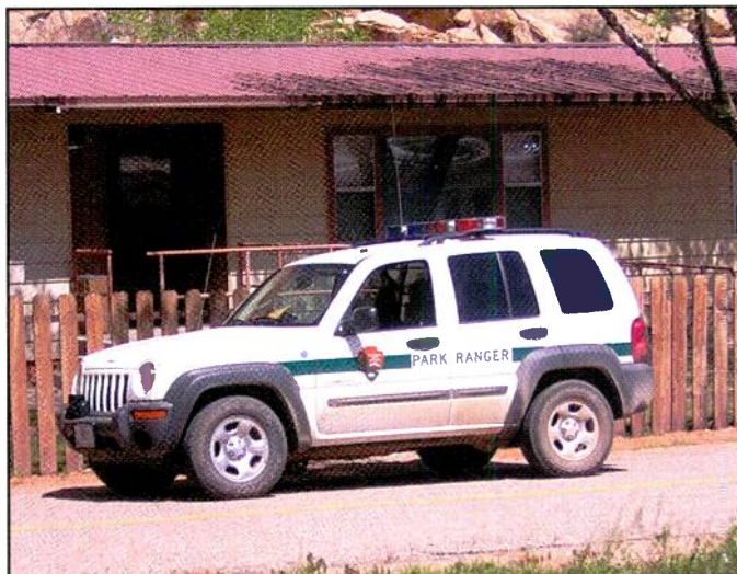
A National Park Service ranger's Jeep is seen parked at Arches National Park in Utah. A long VHF whip antenna offers extended coverage while rangers are out in the park.
