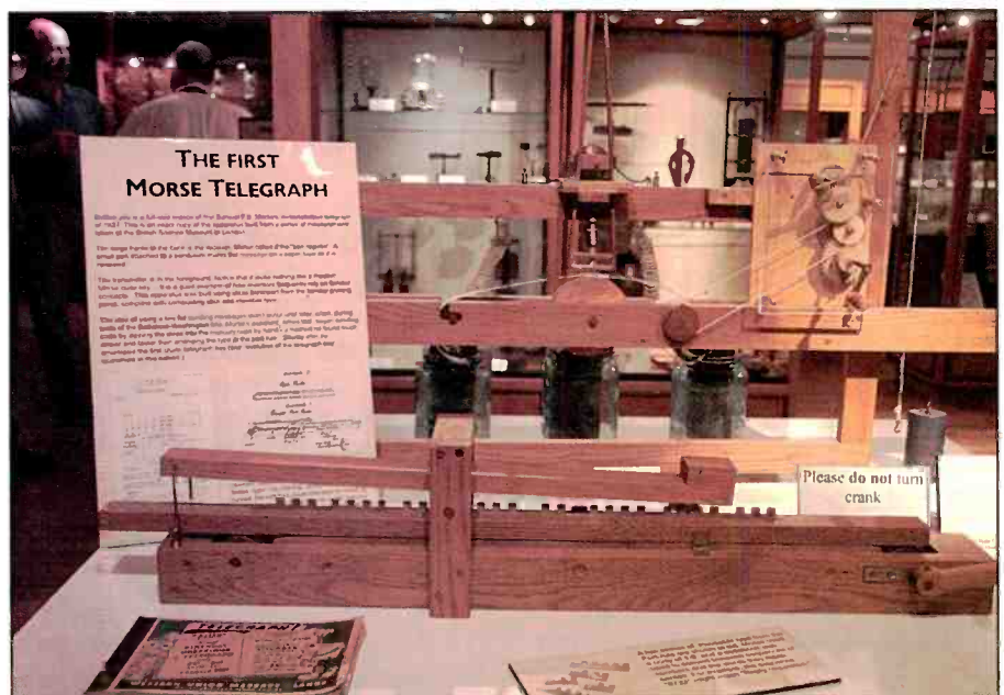
"Before you is a full-size replica," a placard says, of Samuel F.B. Morse's demonstration telegraph, circa 1837. "This is an exact copy of the apparatus built from a series of measurements taken at the British Science Museum in London."
