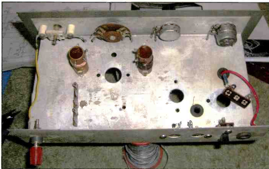
Photo F: Most of the original components couldn't be salvaged and except for a few major pieces, the chassis was stripped bare.
