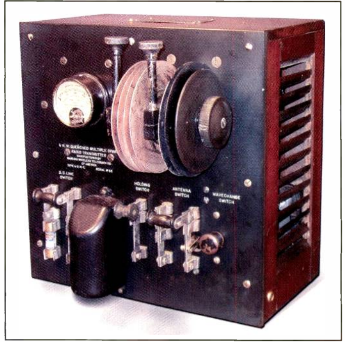
The label on the front panel of this piece of radio gear reads: 1/2 K.W. Quenched Multiple Spark Radio Transmitter – Manufactured by Marconi Wireless Telegraph Co., of America. (From "Where Discovery Sparks Imagination," by John D. Jenkins)
