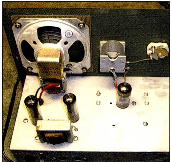
Photo B: The top chassis view shows that the receiver is a rather spartan, three-tube regenerative design.
