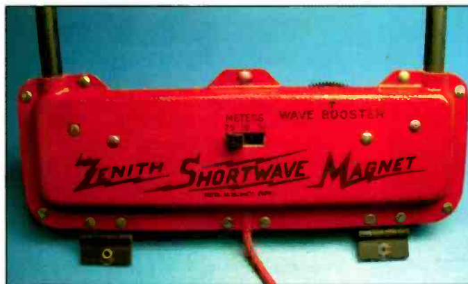
Photo G. The shortwave loop antenna works on three bands. The small slide switch on the antenna manually selects the correct band coverage for the antenna—this extra step is not automatically done by the front-panel band selector pushbuttons.
