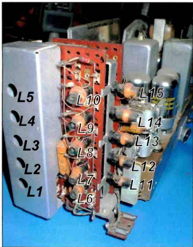
Photo D. The complex tuning-tower is the heart of the Zenith Trans-Oceanic. At the left, the shielded compartment houses the local oscillator band coils. The other coils are for the converter and RF stages. The coil numbers are annotated in the photo to help you identify their locations when doing the alignment.
