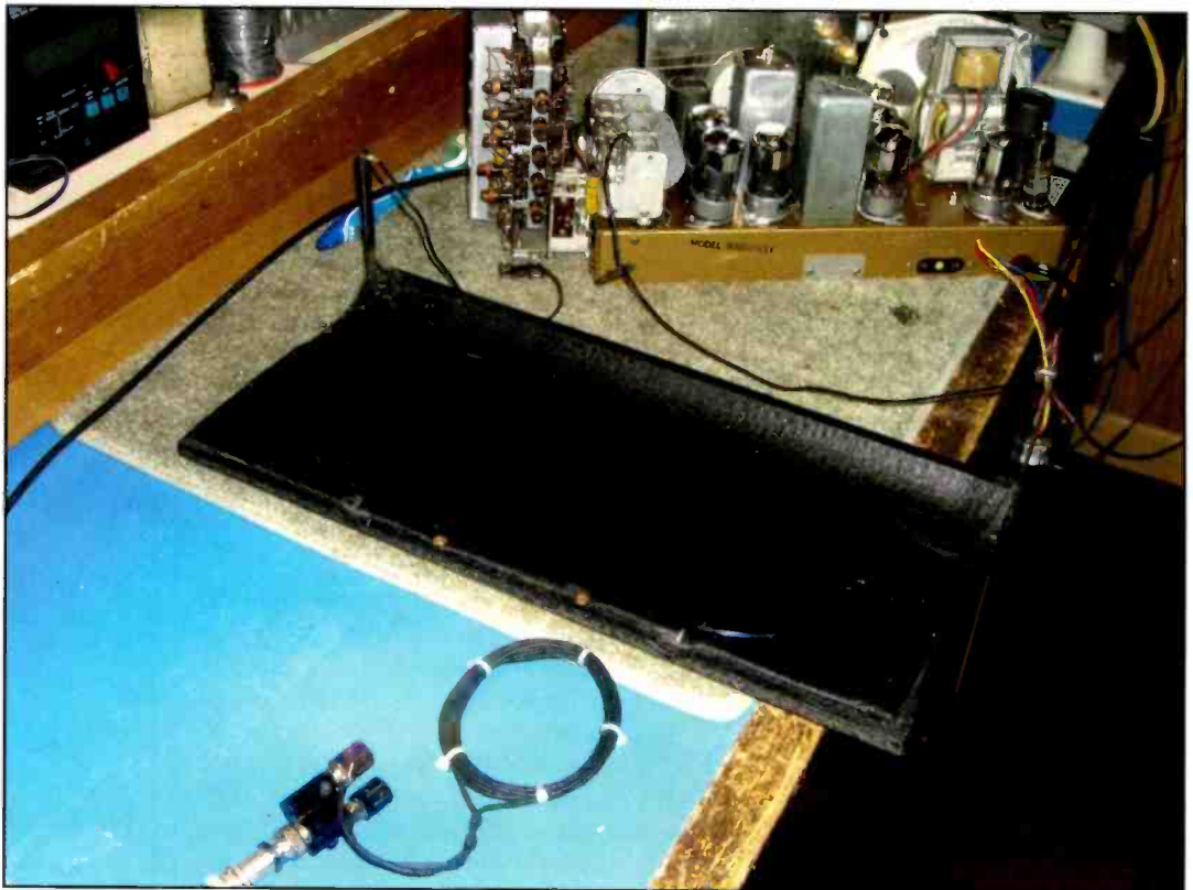
Photo A. Here's a view of the small loop used to inductively couple the signal generator output to the nearby Zenith Wavemagnet antenna. Since the cabinet is torn apart for repairs, you're viewing both the Wavemagnet and the cabinet lid to which it attaches. The Wavemagnet is a high Q tuned loop antenna and is the tuned RF stage for the radio. It should be kept clear of nearby metal objects or clutter.
