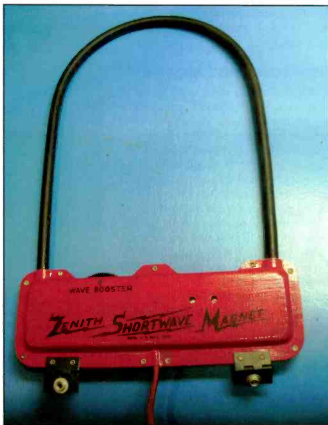
Photo E. This special shortwave Wavemagnet loop antenna can enhance reception on the 19-, 25-, and 31-meter shortwave bands when the radio is used in areas that shield the whip antenna. It is normally stowed with other accessories on the inside of the rear cabinet cover.
