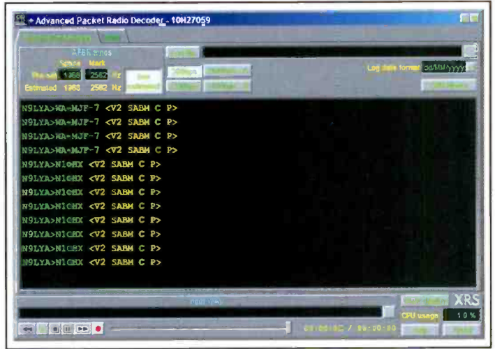
Figure 7. ADS decoding 300-baud HF packet on 30 meters.
