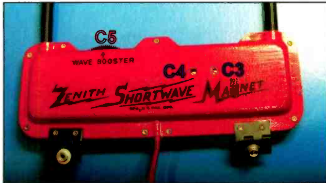
Photo F. The “wave booster” control is used on 19 meters to peak a weak signal. C3 and C4 are alignment points.
