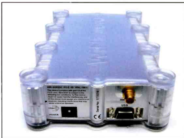
Figure 1. The Excalibur is attractive and modern in appearance. On the rear panel is the power connector, SMA antenna connector, and USB computer connection.
