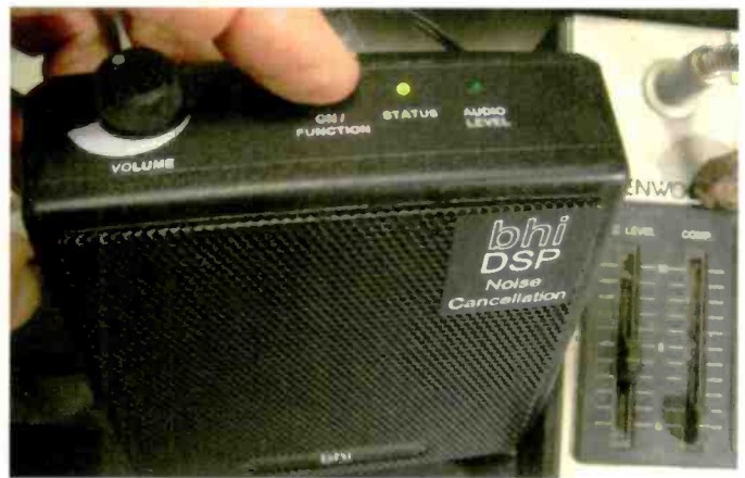
The bhi DSPKR amplified speaker blasts out 10 watts and offers seven levels of digital signal processing.
