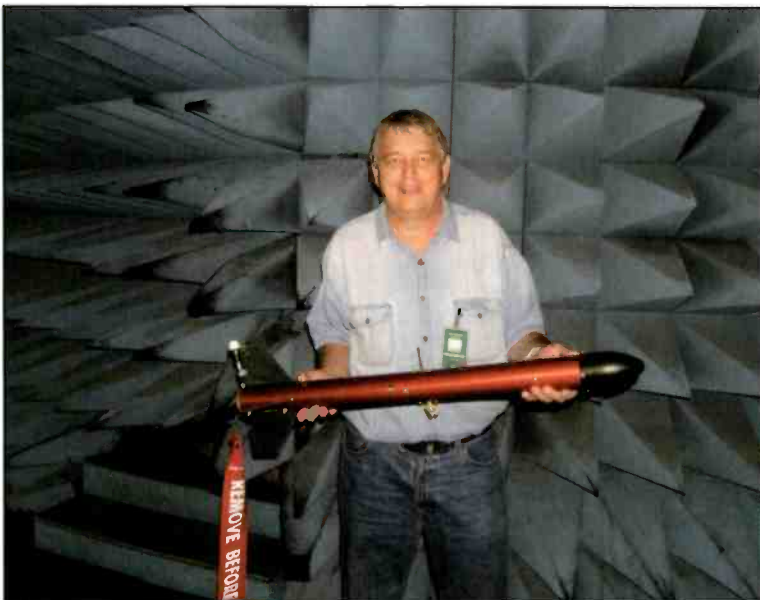
Photo A. Your columnist and a Monopulse Radar Decoy in Radar Cross Section chamber.
