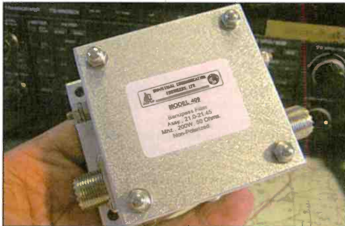
Industrial Communication Engineers' band filter worked great to eliminate another-band's QRM.
