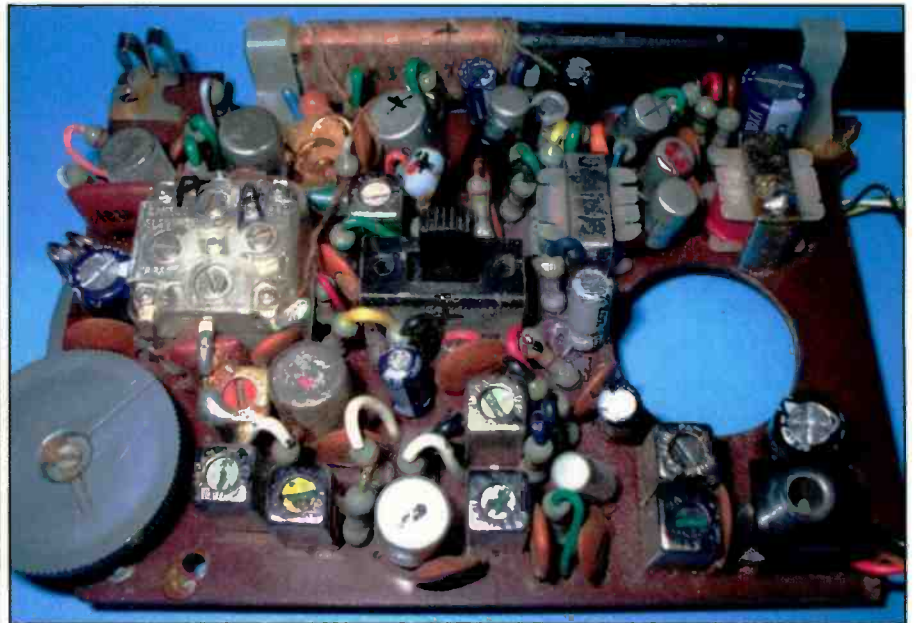
Photo B. A top view of the Jetstream printed circuit board shows the extremely tight component density. It's quite a contrast from the wide-open spaces we've encountered in early tube sets!
