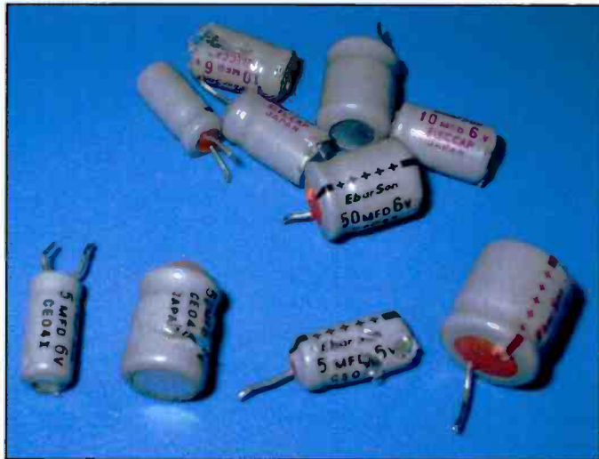
Photo D. As a proactive restoration measure, I replaced all 10 of the original electrolytic capacitors. They exhibited high ESR measurements when the radio was first turned on after decades of non-use.
