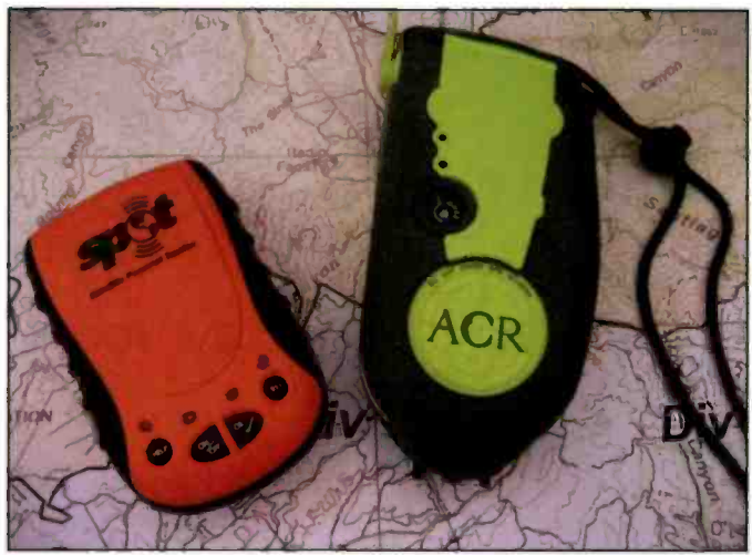
The SPOT satellite transponder (left) is not the same as a Personal Locator Beacon (right). The public needs to know the difference.
