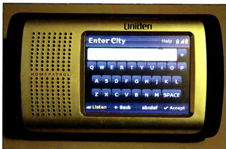
The City entry screen of the HomePatrol. Zip Code entry is similar but uses a numeric keypad instead of the alpha keypad. (All photos by the author, © 2010 Tom Swisher)
