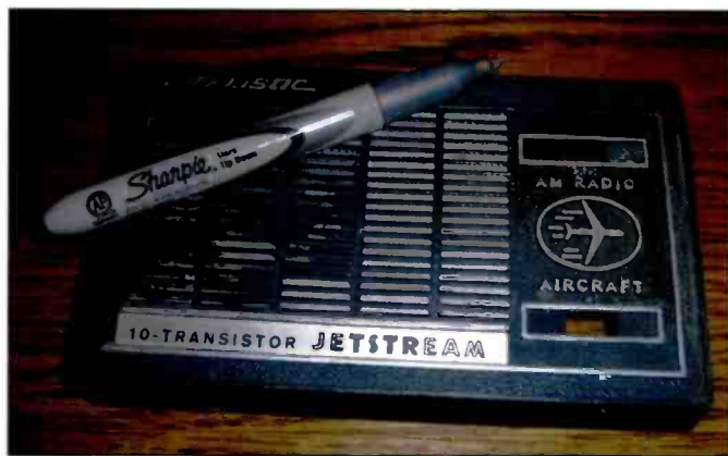
Photo E. The Jetstream originally sported handsome silver detailing on the raised areas of the front panel. Years of use had worn the original finish away, but it was easily restored using silver Sharpie marking pens.
