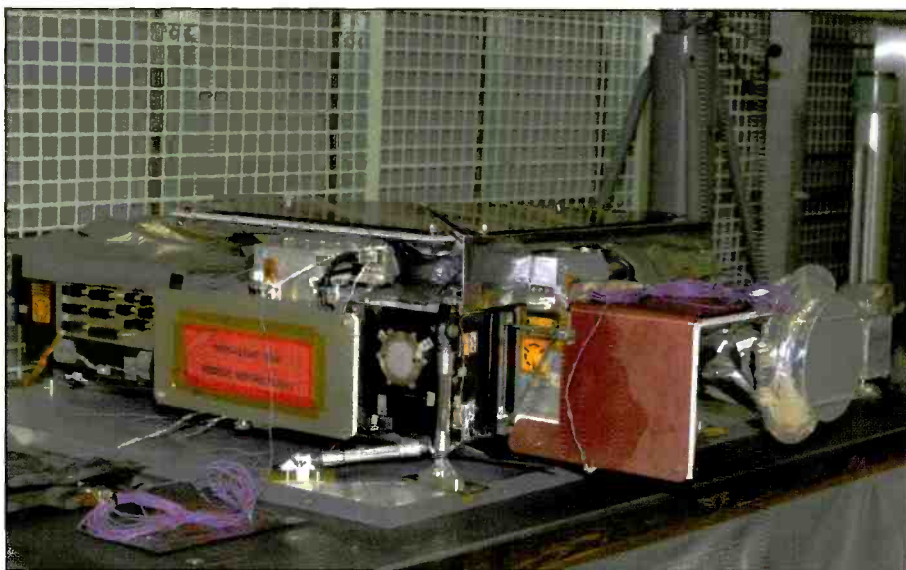
Figure 6. The Solar Dynamics Observatory Helioseismic and Magnetic Imager (HMI) instrument arrives at Goddard. HMI will extend the capabilities of the SOHO/MDI instrument with continual full-disk coverage at higher spatial resolution. (Source: NASA)
