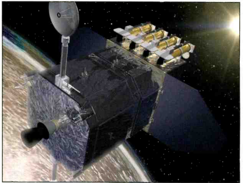
Figure 3. The Solar Dynamics Observatory spacecraft. The SDO satellite is the most advanced spacecraft yet deployed to study space weather and our nearest star. (Source: NASA)
