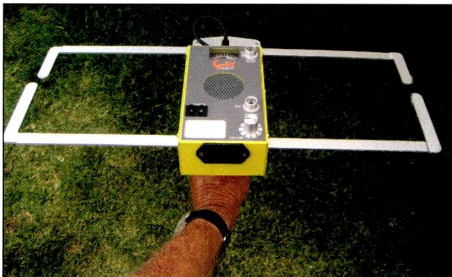
This fold-up Moxon antenna and receiver zeros in on a T-hunt tag.
