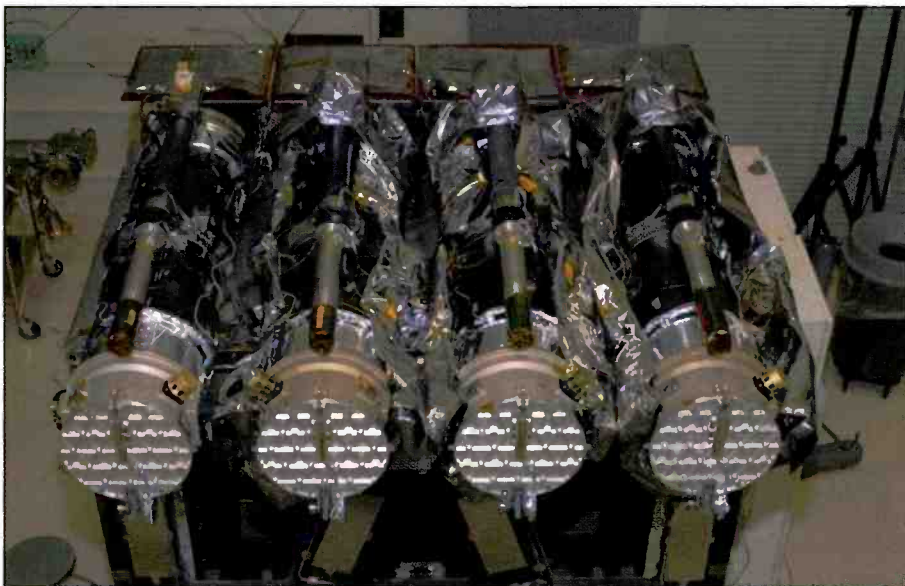
Figure 7. The four Atmospheric Imaging Assembly (AIA) telescopes installed on the Instrument Module in the Space Checkout Area cleanroom at Goddard Space Center. AIA will image the solar atmosphere in multiple wavelengths to link changes in the surface to interior changes. Data will include images of the sun in 10 wavelengths every 10 seconds. (Source: NASA)
