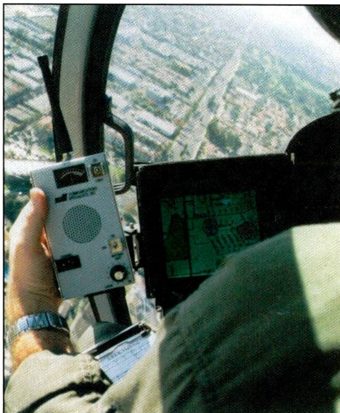
From the air, we detected a 5-milliwatt medical tag three miles away, and ended up hovering over a lost elderly rest home patient until help arrived from the ground.
