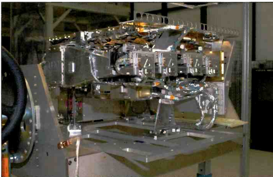
Figure 8. The Extreme Ultraviolet Variability Experiment (EVE) instrument in the clean tent. The EVE experiment measures the solar extreme-ultraviolet (EUV) irradiance with unprecedented spectral resolution, temporal cadence, and precision. It will help scientists understand variations on the timescales that influence Earth's climate and near-Earth space. (Source: NASA)
