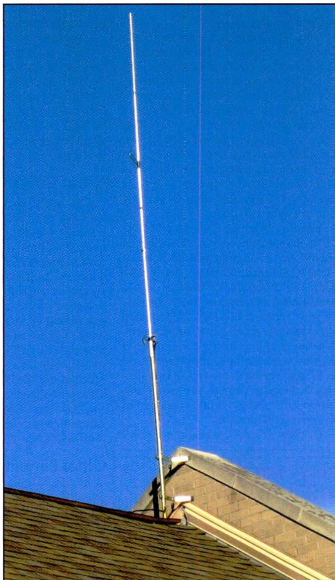
The 2-meter Ringo Ranger antenna mounted on the peak of the building gives great coverage.
