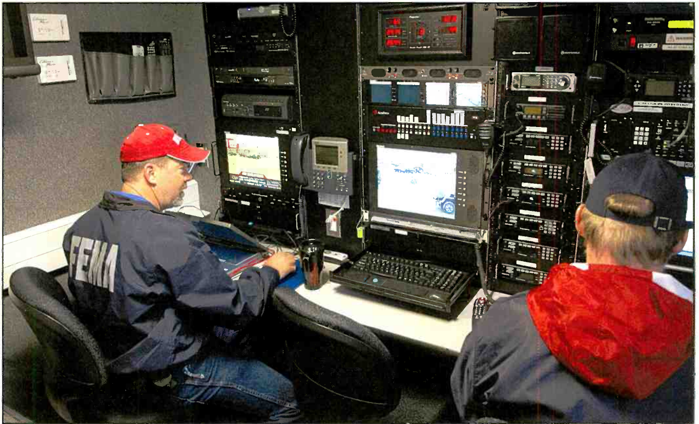
FEMA personnel work inside a Mobile Emergency Response Support (MERS) vehicle. These vehicles are equipped with satellite communications systems to enable communications wherever they are needed. (Photo courtesy FEMA/Mark Wolfe)
