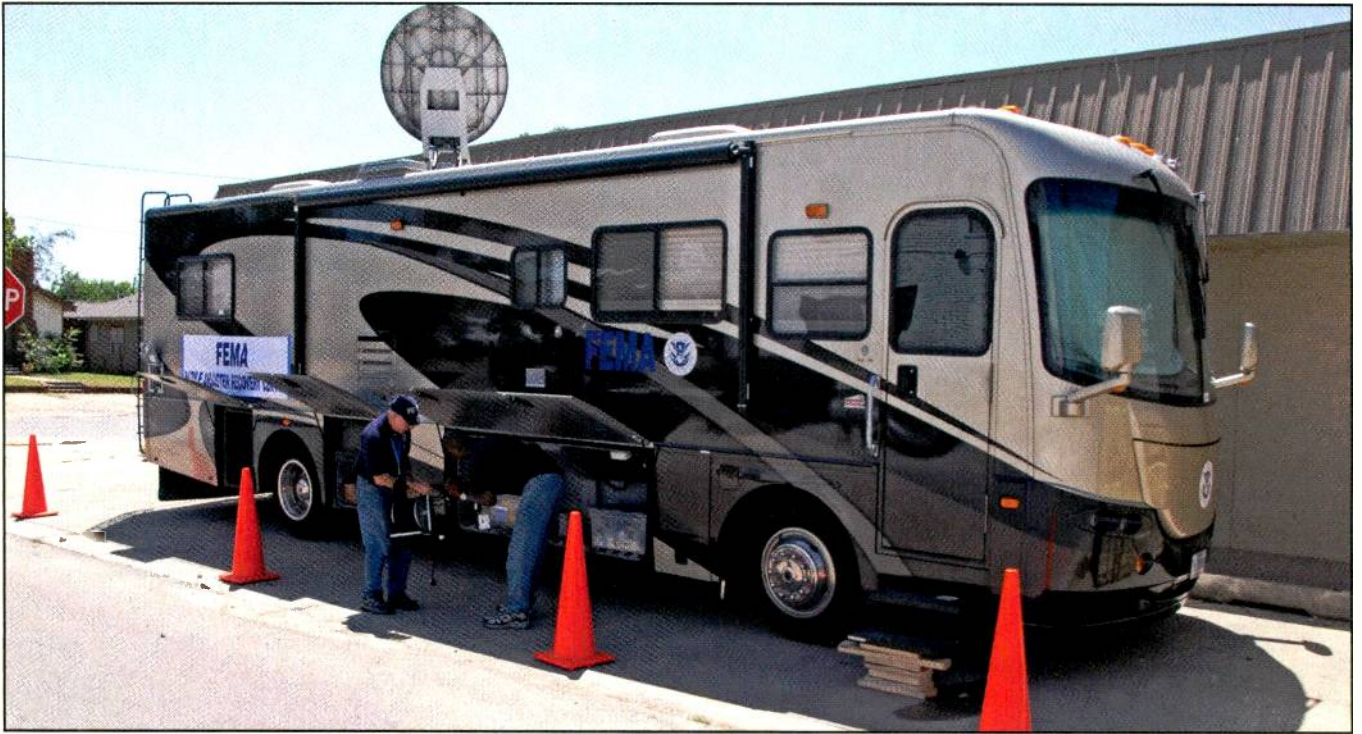
FEMA workers setting up a Mobile Disaster Recovery Center. These campers are self contained and include satellite uplinks and other forms of mobile communications. (Photo courtesy FEMA/Marvin Nauman)
