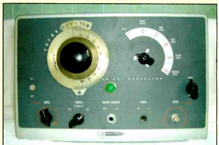
Photo A. This Heathkit IG-62 color bar generator, an inexpensive flea market find, yielded the tubes, sockets, enclosure, and many parts that were reworked into Richard’s ham version of the Night Hawk regenerative receiver.
