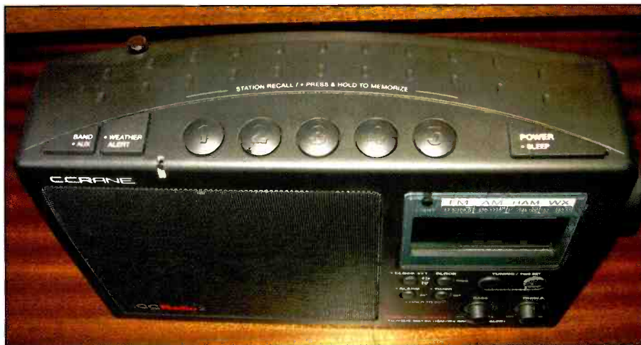
The top panel of the CCRadio-2 includes five memory stations, a band selector, weather alert plus a sleep mode option.
