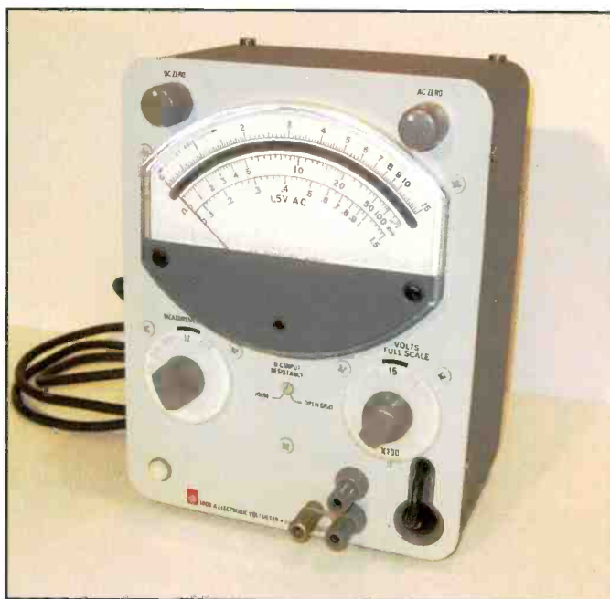
Photo E. The General Radio model GR 1806A is a real sleeper! The meter design is elegant simplicity and is surprisingly modern for a General Radio product. The meter has only three scales, making it one of the most user-friendly VTVMs out there. Unfortunately, they also seem to be very rare. (Photo courtesy Mike Harrison, KEØZU)
