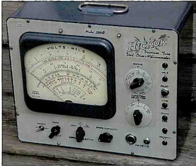
Photo J. Here's another of my favorite VTVMs, an earlier example of the Hickok model 209A. The huge meter can be easily read across a small room! These meters are fairly common, but unfortunately many display rust and other damage from years of neglect and poor storage conditions. (Photo courtesy historian Alan Douglas)
