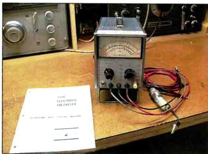
Photo D. Dating from the early 1960s, Mike Harrison, KEØZU's example of a HP 410C marked Hewlett Packard's transition from the all-tube HP 410A and 410B VTVM model lines to a solid-state version. However, the AC probe on the 410C continued using a tube diode detector.
