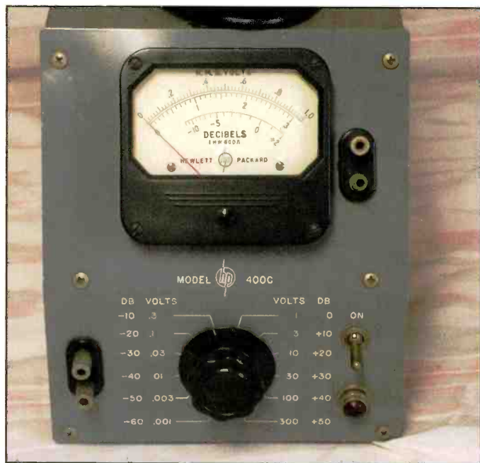
Photo C. The Hewlett Packard model 400C, circa 1950. It's an AC-only VTVM, with a frequency response from 20 Hz to 2 MHz, and covers from 100 \mu V to 300 volts in 12 ranges. (Photo courtesy Tom Kelly)
