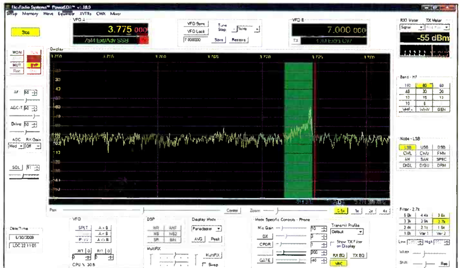
Figure 2. PowerSDR 1.18.1 main screen with receiver tuned to 3.775 MHz LSB, 2.7k bandwidth. The graphical display in the center of the screen is the panadapter.
