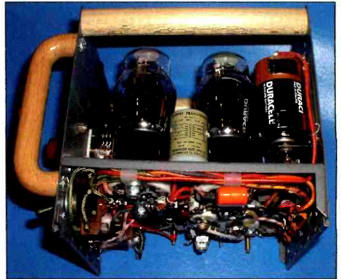
Photo D. The A battery, a single D cell is visible on the back wall. The UTC Subouncer transformer is visible between the two #49 tubes.
