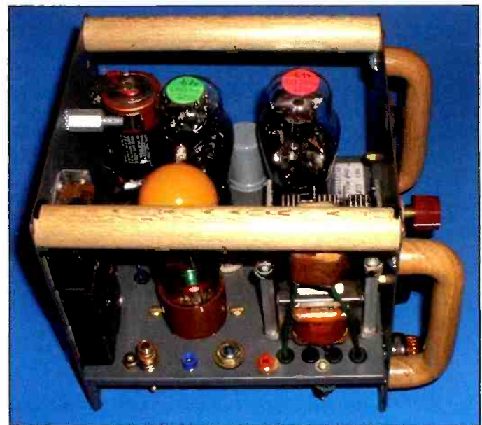
Photo E. This oblique view shows overall top of chassis layout. Note the stacked set of three transistor batteries on the rear apron panel that the supply the B+ voltages for the receiver. The rotor plates for the tuning capacitor are just visible at front and center.
