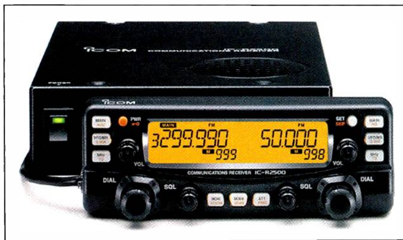
The ICOM IC-R2500's control head attaches to the main unit by a cable that looks a lot like a telephone cable.
