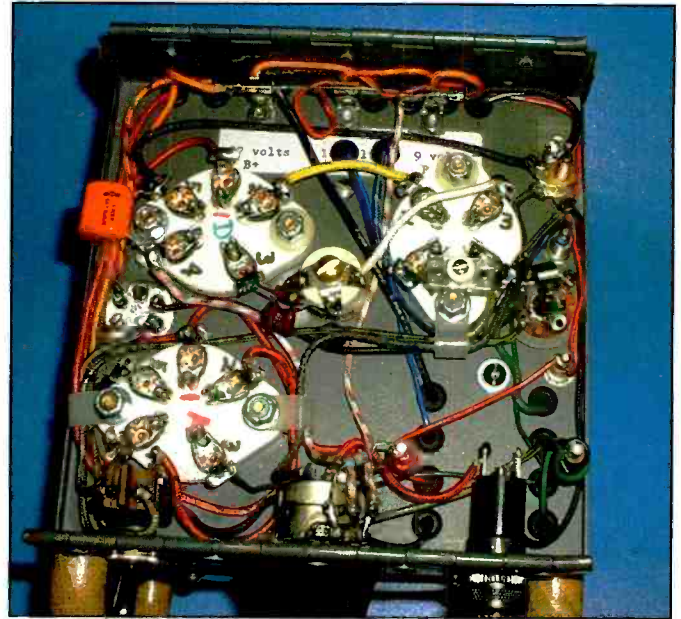
Photo B. Bottom view of the receiver chassis. High-quality ceramic sockets are used throughout!
