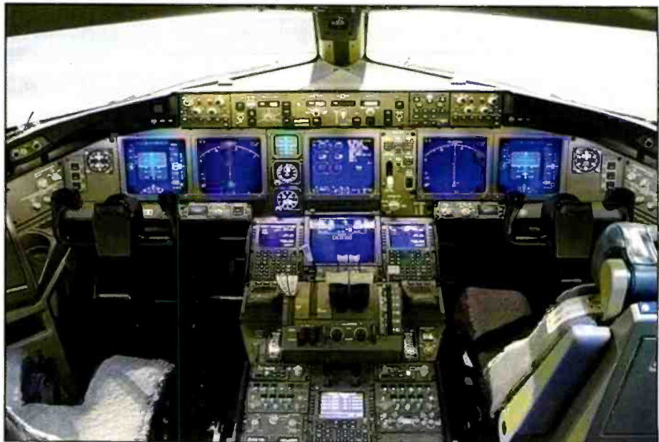
The cockpit of a Boeing 777. The integrated displays use information from various sources, such as ADS-B, to provide situational awareness for the pilots. (Photo courtesy of AviationEarth)
