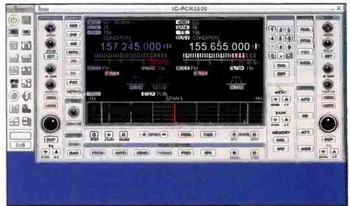
Photo B. The included software from ICOM gives you a choice of three main receiver presentations. This simple screen is perfect for basic operations and casual listening while using the computer for other tasks.
