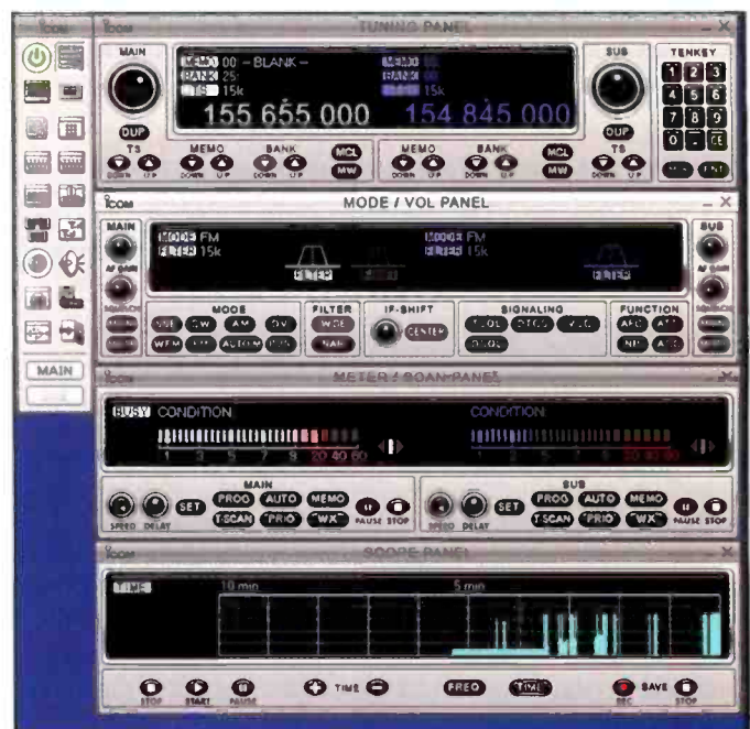
Photo C. For a more full-featured operation, the receiver screen looks and feels like a dual VFO communications receiver. A bandscan function is also available at the bottom of the display.
