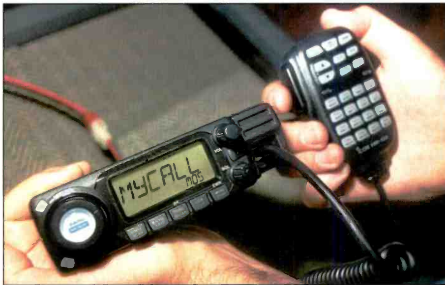
By design, the digital stream transmitted by D-STAR-equipped radios includes the user’s callsign, which is programmed into the “MYCALL” field. ICOM America is the only manufacturer selling D-STAR-capable radios in the United States; the company’s ID-800H is shown here. (KB3CNM photo)
