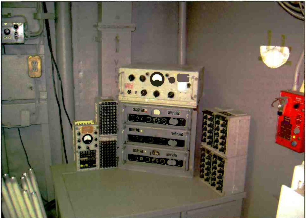
Photo A. The red box at right is a KY-8 voice cryptographic unit. (KC2HMZ photo)
