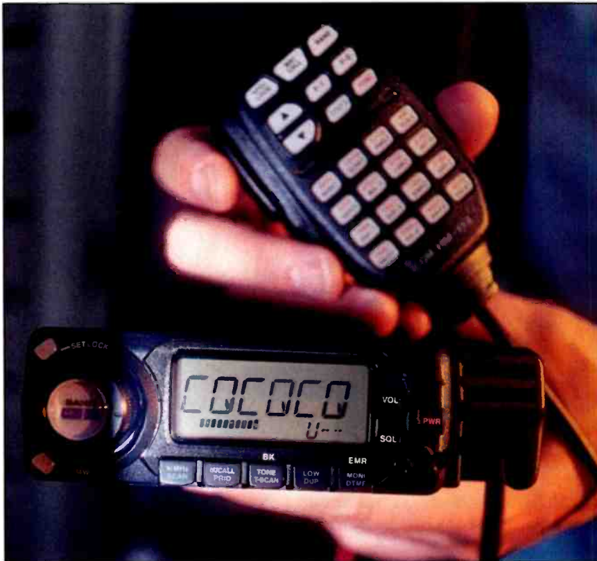
After registering for access to the Internet at their nearest D-STAR gateway, users are able to call CQ through any D-STAR-equipped repeater anywhere in the world. (KB3CNM photo)
