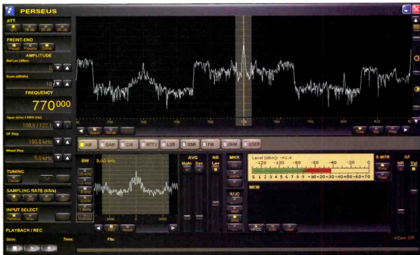
Figure 2. Here you can clearly see the 30-kHz digital IBOC sidebands of WABC 770 kHz in New York. BCB DXers have been complaining about the QRM of the IBOC sidebands for some time now. The Perseus spectrum display is set to 100 kHz in this instance.
