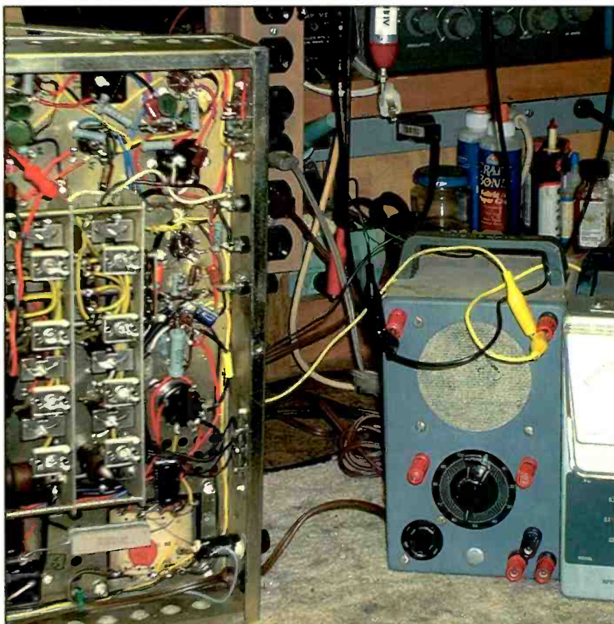
Photo A. Our speaker test jig project is teamed with a Heath IM-21 AC VTVM to monitor the recovered signal generator audio on the HE-10 speaker terminals.
