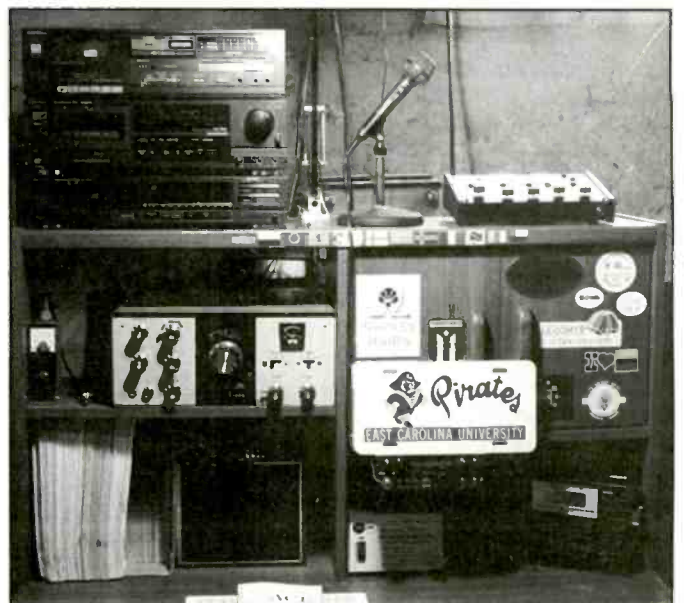
Photo B. The Omega Radio setup from the early 1990s, showing the Heathkit HW-101 transceiver, at the center left of the shelves.
