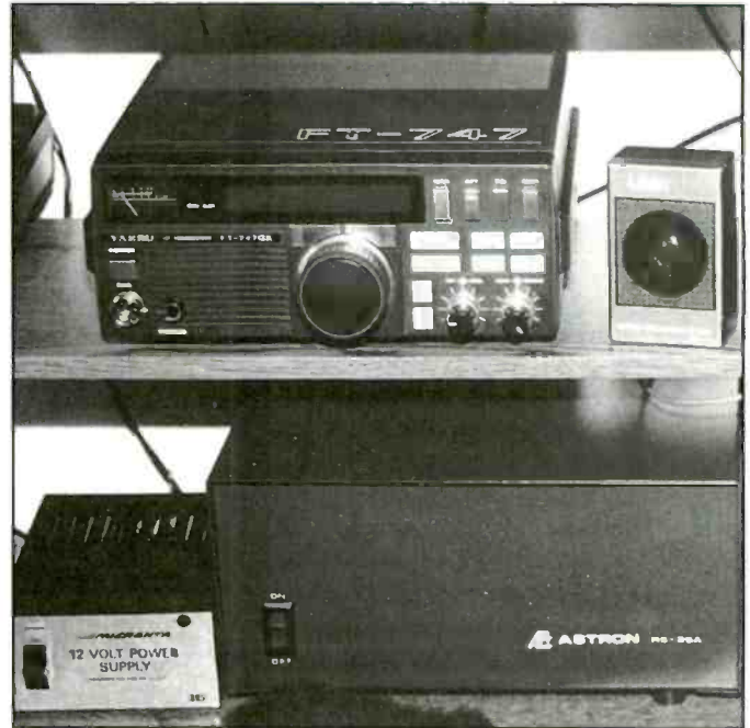
Photo A. WCYC's equipment from the early 1990s, showing the Yaesu FT-747 transceiver at the center of the top shelf and the AC power supply underneath.
