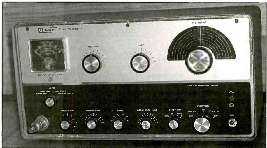
Photo D. A Knight T-150 transmitter from the early 1960s. Although used by a number of pirates over the years, the grid-modulated AM with carrier control doesn't provide broadcast-quality audio.
