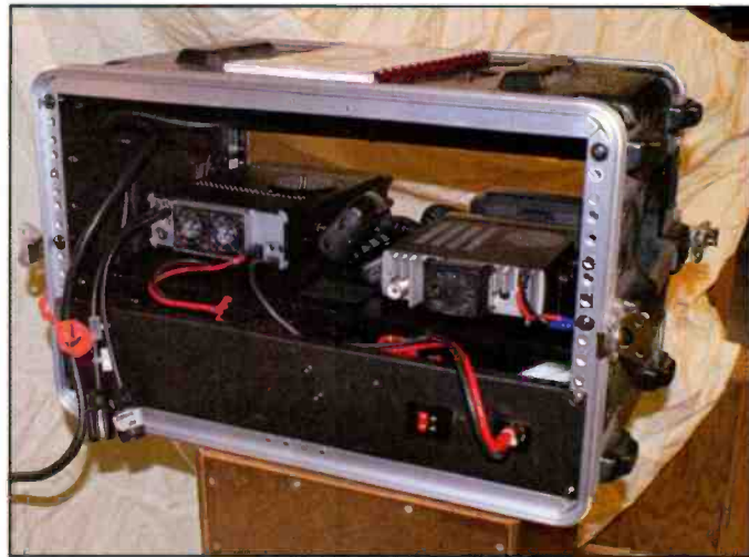
John Gianotti, W9WY, of Munster, Indiana, has done a terrific job assembling his EmComm Go-Box in a musician's equipment case. This case features standard 19-inch rack panel spacing and is extremely versatile. John covers HF with a Yaesu FT-100D transceiver and VHF/UHF with a Kenwood dual-bander. He excluded internal batteries in favor of a small switching power supply since all his ARES/RACES callouts to date have had 120 VAC available. John provided front and back views of his EmComm Go-Box.
