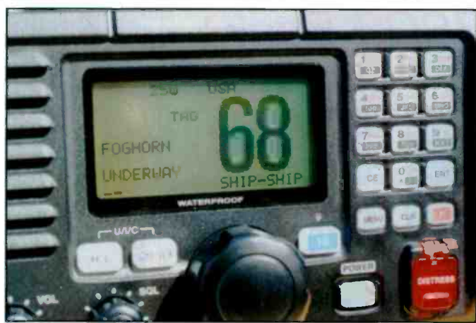
Digital Selective Calling (DSC) marine radios dual-watch VHF Channel 70 for distress calls.
