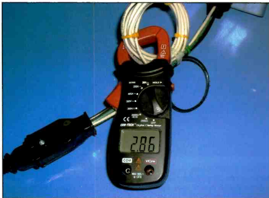
Photo D. The Cen-Tech meter is clamped over the 10-turn winding in this test setup. The meter is indicating the current being drawn by a small pencil soldering iron. While the meter is showing 2.86 amps, remember that this reading is actually 10 times more than the actual current being drawn. The iron is drawing 1/10th that current: 286 mA.
