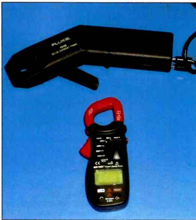
Photo A. The Cen-Tech clamp-on ammeter is shown in the lower portion of the photo. Above it is a Fluke clamp-on probe that will measure both AC and DC currents when used with a companion digital meter.
