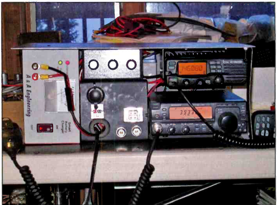
Frank Henrikson, KLØSW, from Alaska has constructed his Go-Box using a modified GI ammo can that houses a simple “rack” system that can be dismantled and re-deployed quickly. His radio setup consists of a Kenwood TS-50 for HF and an ICOM IC-V8000 for VHF FM. There’s a deep cycle gel-cell battery housed in the base of the rack and an A&A Engineering “smart charger” that will not overcharge the battery if left on full time. HF antenna matching is handled by a small MFJ 160-10 manual tuner and the SWR bridge on the TS-50. Many thanks to Frank for the photo.
