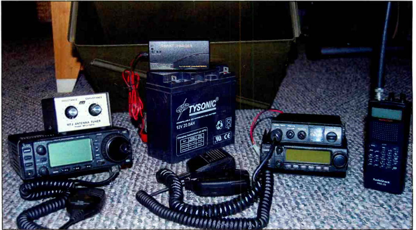
Here's my EmComm Go-Box project in the works, showing what the ammo box will eventually contain (from left to right): an ICOM IC-706 with MFJ 160-10 ATU, Tysonic 20A/hr gel-cell battery with "smart charger," ICOM IC-2100 2-meter FM transceiver (below) along with a RadioShack 40-channel CB set (top), and a RadioShack PRO-79 scanner (which will be updated later to a digital/analog trunk tracker). I was going to include a second 20A/hr gel-cell battery inside the ammo box, but that would bring the total weight to 30 pounds in batteries alone! Eventually the ICOM IC-2100 will be replaced with another Kenwood TM-D700A dual-band FM rig. The really nice thing about this Go-Box is that both the HF and VHF/UHF units can be removed if table/workbench space is at a premium. It's all about the versatility!
