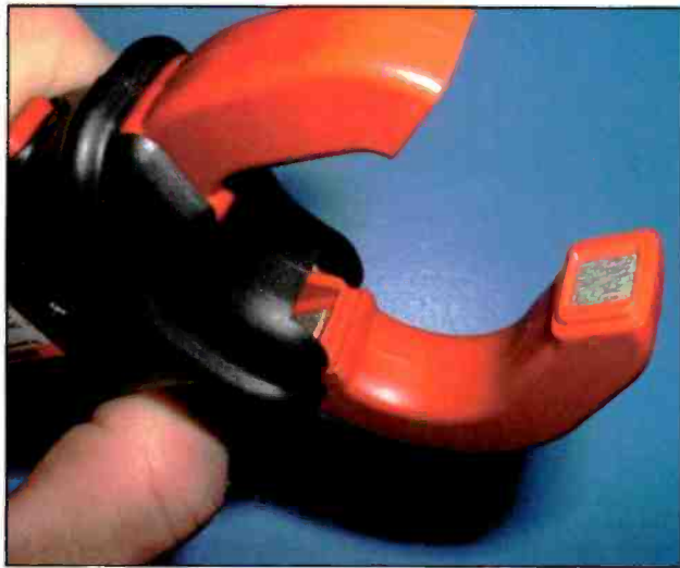
Photo B. Clamp-on meters measure the magnetic field generated by the conductor the probe is clamped over. The conductor acts like a single-turn primary winding in a transformer. In this photo the core laminations in the moveable portion of the clamp probe are visible.
