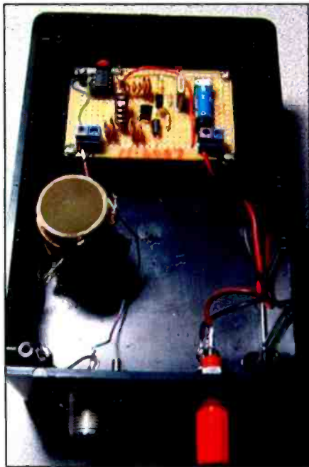
Photo B. The transmitter for an often-heard “dasher” beacon located in Colorado; see article text. (Courtesy of High Frequency Beacon Society)
