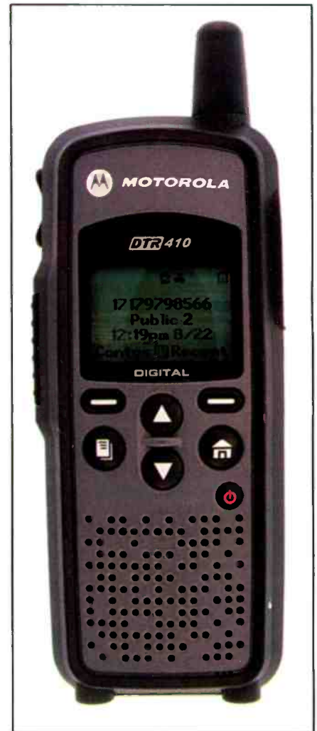
The Motorola DTR410 digital FHSS license-free transceiver represents a technological trend in two-way radio. This advanced technology is becoming increasingly affordable to non-government users.
