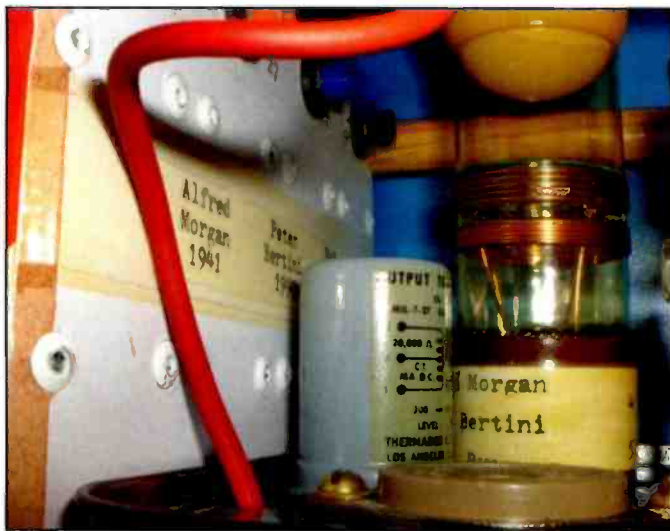
Photo 1. The Doerle Twinplex used a vintage audio interstage between the detector and audio stages to provide voltage gain. Bob's chassis provided a 20,000-ohm center-tapped audio transformer. I was able to wire up the CT primary autotransformer in similar fashion to provide the same gain for the recovered detector audio.
