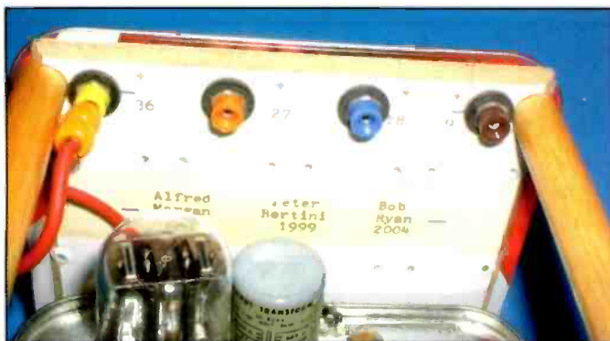
Photo C. The bank of 9-volt batteries was wired in series, and each of the tie points included a pin jack to select the optimum detector voltage. This scheme would work well with sets based on Alfred Morgan designs, which often worked well with 9 or 18 volts on the detector plate.
