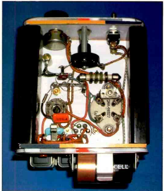
Photo F. Here's the under chassis wiring. I used vintage cloth insulated wire salvaged from old TV service test cables. I'm sure Bob will approve! Bob included a pilot lamp on prototype. This isn't mentioned in the text since I felt it shortened the D cell life.
