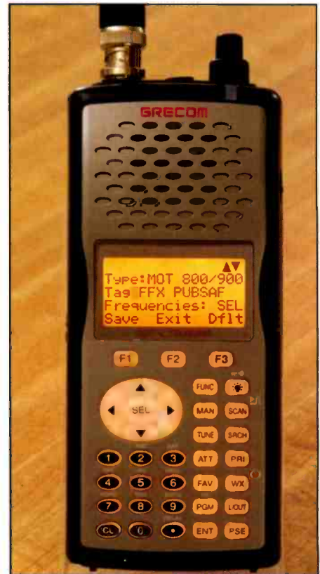
Here we're editing an object, as discussed in the text. The screen shows the trunking system (TSYS) menu with trunking Type, Tag, and Freq selections.
