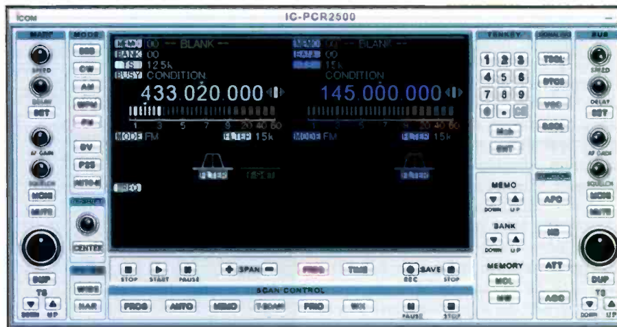
The ICOM IC-PCR2500 user interface featuring simultaneous reception of two frequencies.
