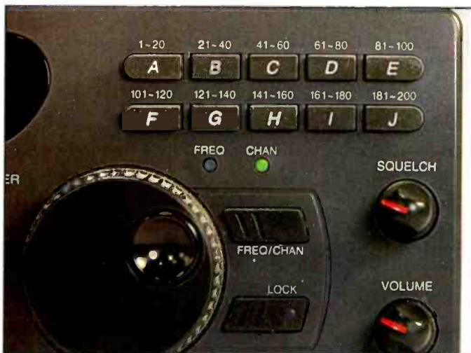
This unique arrangement from Uniden and RadioShack separated the bank switches and labeled them with alphabetic characters. Later versions of this radio had 20 banks: 10 numeric and 10 alphabetic. Nice feature, and more banks!
