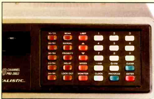
Just about the time Pop'Comm first came along, so did this 50-channel radio from RadioShack. It was one of the first with actual banks of 10 channels, each of which could be switched on and off easily with the numbered keys at the far left on the keypad.
