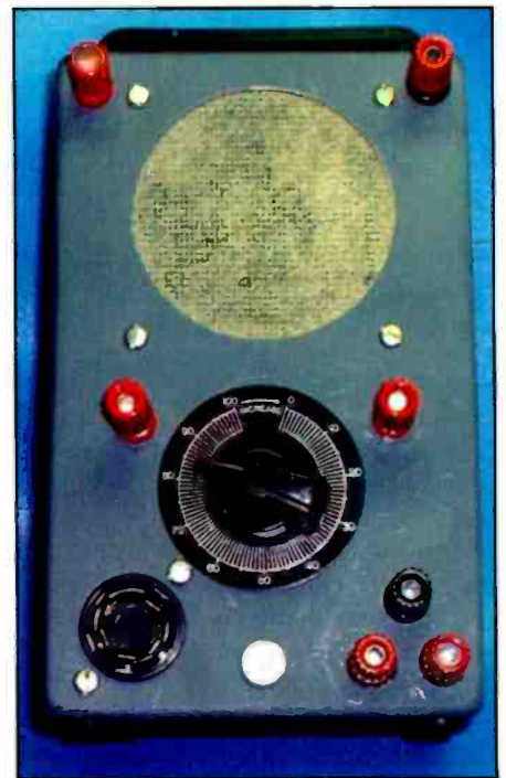
Photo B. The completed speaker test jig is housed in a salvaged Heath T4 signal tracer enclosure. I painted the front panel to hide the old control markings. I added extra binding posts to bring out the rheostat, speaker, and audio transformer connections for flying lead hookups. A five-pin socket permits the use of custom extension jumper cables made up for the more common sets.
