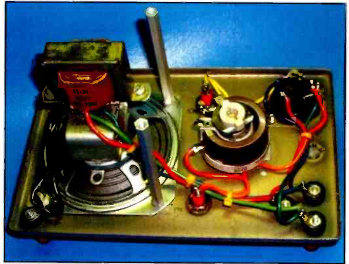
Photo A. Here's an inside view of my speaker test jig. The speaker, audio transformer, and many of the other smaller parts were salvaged from a non-repairable junk Heath T4 signal tracer. Note the long threaded spacers that provide a means to attach the front panel to the enclosure. All wiring and parts must be able to withstand voltages in excess of 500 VDC.
