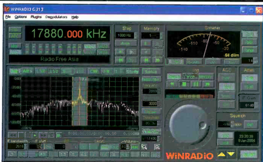
The WiNRADiO WR-313e/i user interface featuring an integrated spectrum analyzer display.
