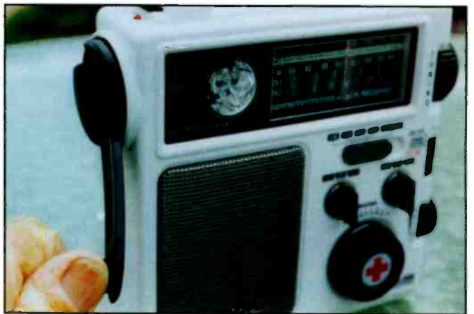
Here’s the dynamo crank to recharge the encased battery pack.
