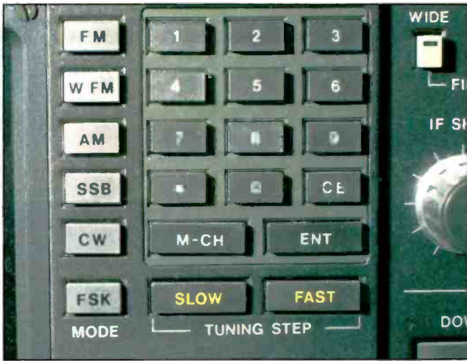
Another feature of the true communications receiver is the ability to choose the operating mode. Shown here are the mode switches from an ICOM R-9000.
