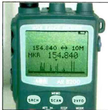
One feature that's becoming common on newer communications receivers is the spectrum display, a graphical view of signals that are near your current frequency. This AOR AR-8200 features this somewhat useful version, but it's no substitute for a true spectrum display unit.
