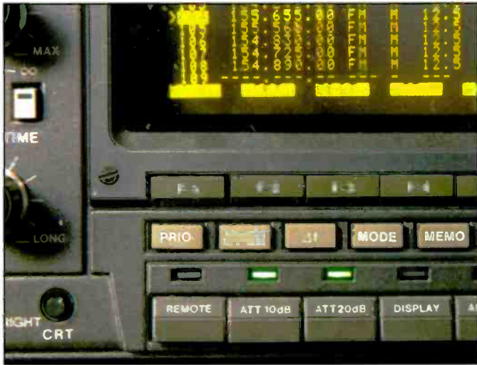
The types of scan available are varied, but none of them approaches the convenience of your garden-variety scanner. This R-9000 has a Priority Scan, Program Scan, Triangle F (Delta F) Scan, a Mode Scan, and Memo Scan. Memo is the closest to what a normal scanner does, but its top speed is about 10 or 15 channels per second.
