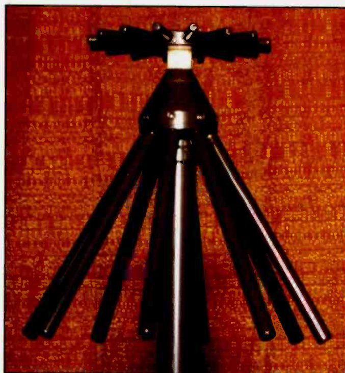
Discones come in all shapes and sizes (this is a DA5000 from AOR). Smaller versions like this are designed for higher frequencies, but larger ones can easily cover 4 or 500 MHz of spectrum—all with equal mediocrity. But at least some coverage is better than none.
