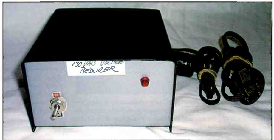
Photo A. Here's a front view of Ted's voltage reducing accessory. Alas, I suspect most of the components used were once readily available at RadioShack outlets. Note that Ted installed a pilot lamp and power switch on the front panel.
