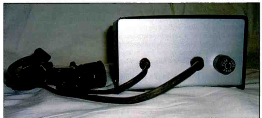
Photo B. Here's a view of the rear apron. The power cords and fuse holder are visible. The AC socket could be mounted on the project box if a female-socket-type power cable assembly isn't readily available.
