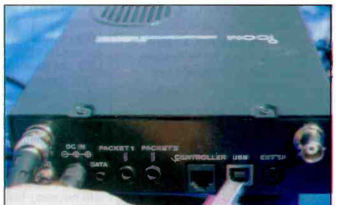
The "business end" of the PCR2500 receiver, hooked into the computer with the pink USB cable.
