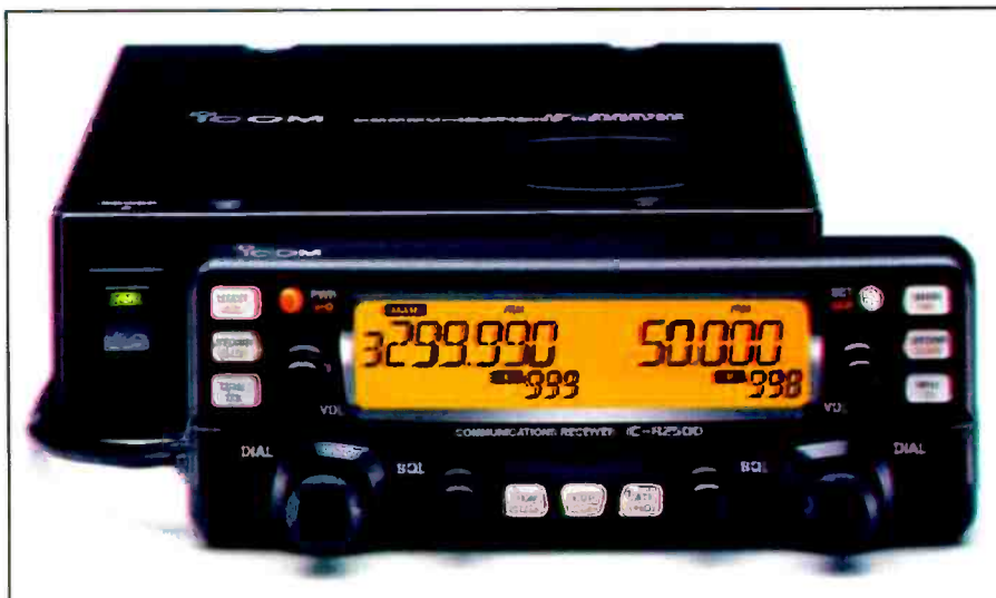
ICOM's IC-PCR2500 is a full-blown PC-controlled black box receiver that will accept a P-25 Public Safety digital board for unencrypted APCO-25 transmissions.
