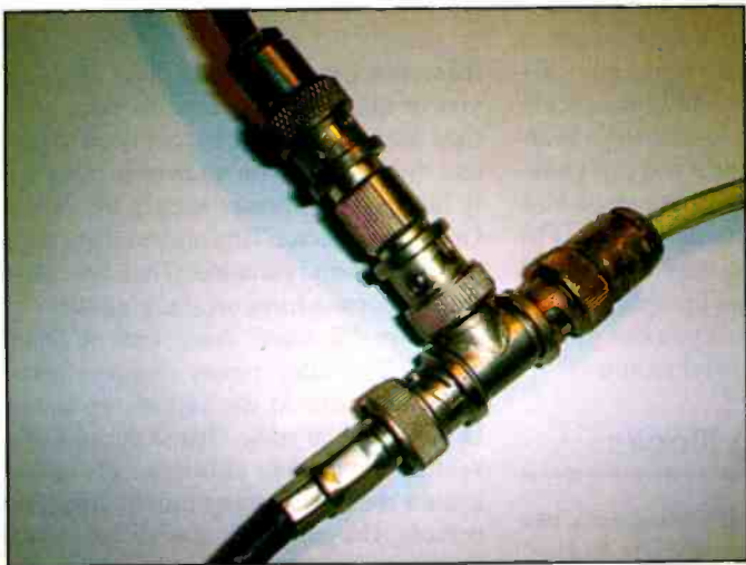
Photo C. How not to connect an antenna to two radios!
