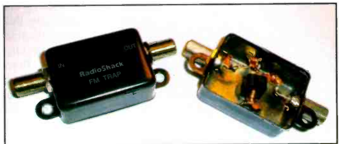
Photo E. FM band notch filters that can reduce intermod.
