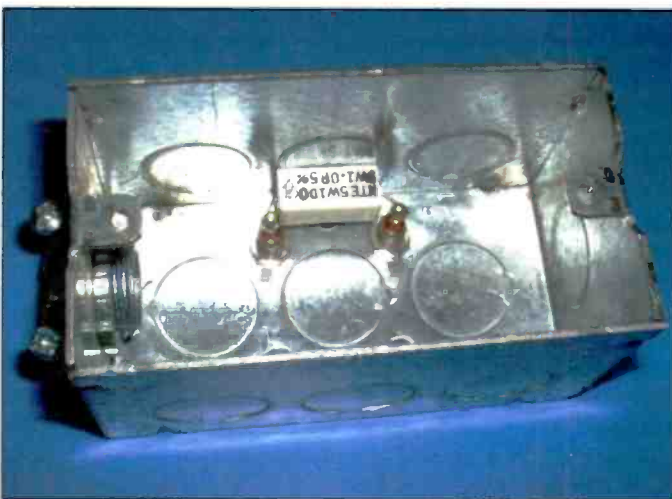
Photo B. The electrical box had four holes in the bottom that were ideally located for mounting the four pin jacks! Two of the pin jacks are used to mount the power resistor.
