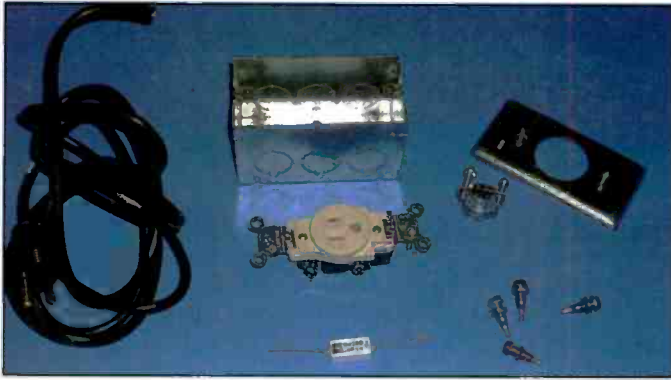
Photo A. Only a handful of components is needed. Many items can be found on the electrical supply shelves at the local hardware store. The four pin jacks and the resistor are available from most electronic supply houses.
