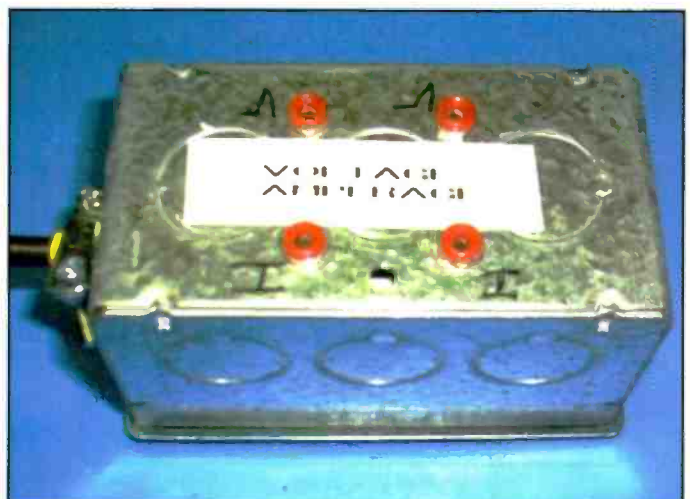
Photo D. Keep the wire leads short and neat. When everything is assembled, the wiring should be routed away from the resistor (which can become hot in operation) to avoid damaging the insulation.
