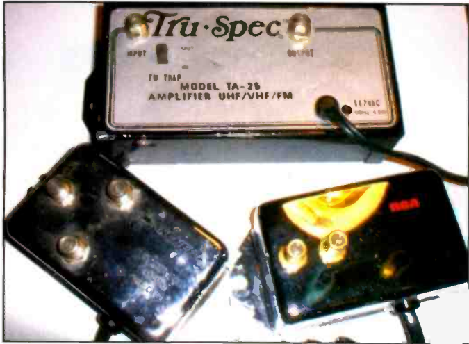
Photo F. Wideband preamps, most of which have 10 to 20 dB of gain.
