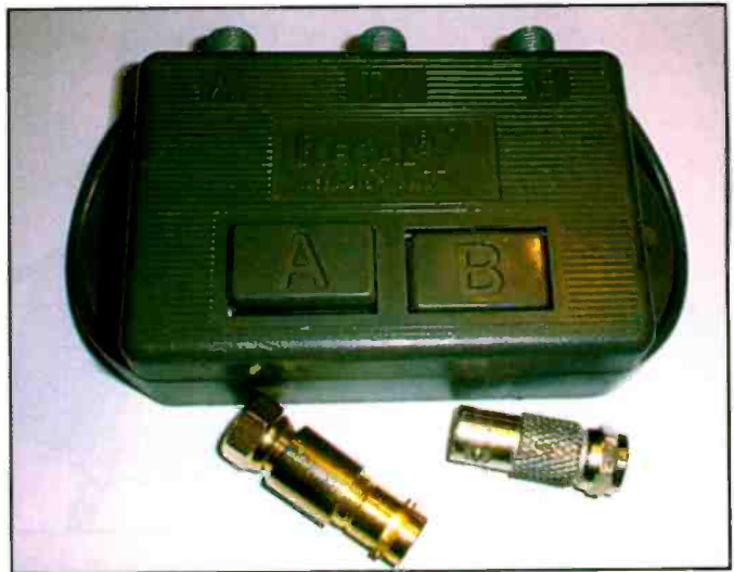
Photo D. A-B antenna switch and F-BNC adapters.
