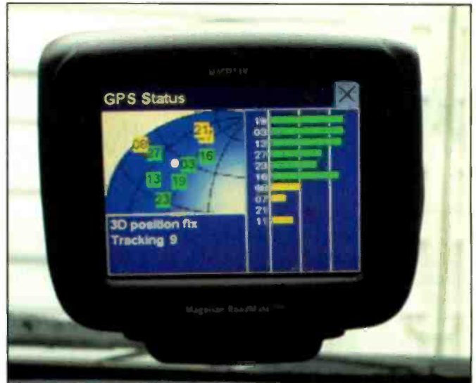
The tracking screen showing the unit locked onto nine GPS satellites in the 3D mode.
