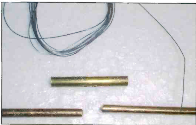
Photo F. Splicing a brass or copper element.
