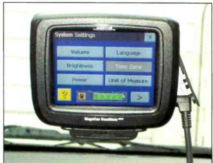
The five green bars at the bottom center of the screen show the charging status and that the 2000 is plugged into 12 VDC.
