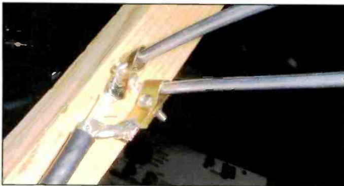
Photo E. Soldering clips for an aluminum rod driven element.
