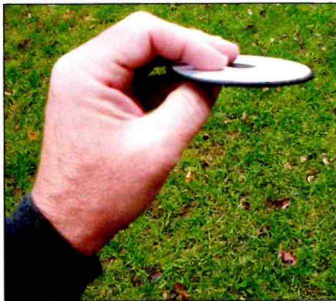
The Magellan RoadMate™'s adhesive mounting pad is included with the 2000. Clean a very flat surface on your dashboard, ensuring it's free of any commercial vinyl cleaner/coating, and press the disc in place. Wait at least an hour or two before mounting the 2000's suction cup mount to the disc.
