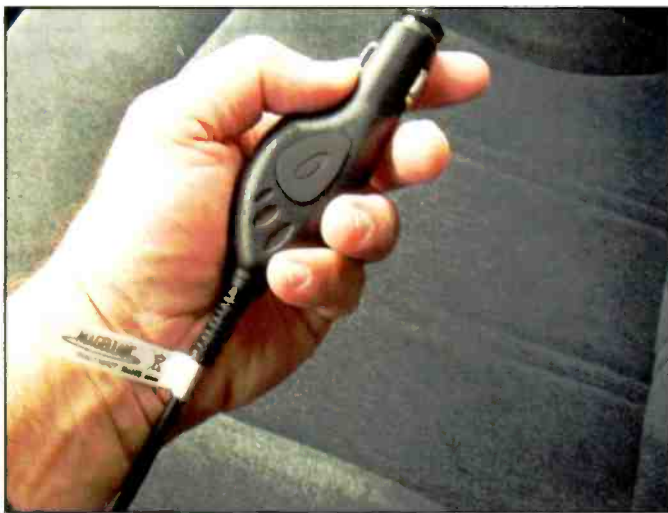
The larger-than-normal cigarette lighter adapter/charger plugs into your vehicle's 12-VDC power supply receptacle. It takes four to five hours to completely charge the unit.
