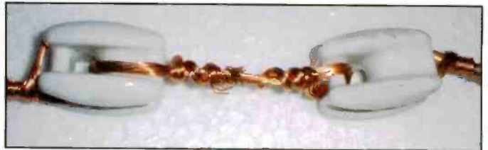
Photo G. Wires and antenna egg insulators.
