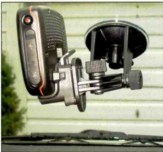
Here's a view of the RoadMate 2000 turned sideways to show the two small thumbwheels for adjusting the left/right and up/down angle of the unit for best viewing. The small pushbutton on the top of the unit turns it on and off. It truly is a power-up-and-go GPS.
