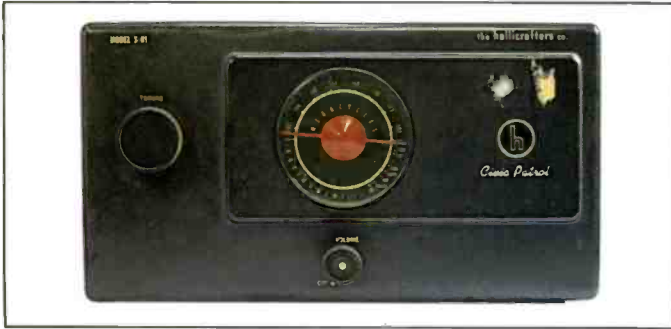
Here’s an early VHF receiver. All tubes, of course, and no squelch! No scanning either. Pick a frequency and listen. This one is probably 1950s vintage, but the “scanner” didn’t come along until the late 1960s. It was really the CB radio craze as much as anything else that drove scanning and shortwave listening forward in the 1970s.
