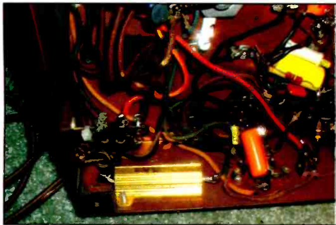
Photo E. Once you're sure that the selected resistor will do the job, find an open location, preferably on the rear chassis apron, where it can be mounted. Heat conducted to the chassis will be eventually dissipated to the room by air currents and radiation.
