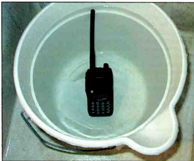
You can't do this with your cell phone or most other radios. The DJ-V17T survived The Dunk. Okay, I didn't leave it in the water for the full 30 minutes—even my insanity has its limits!
