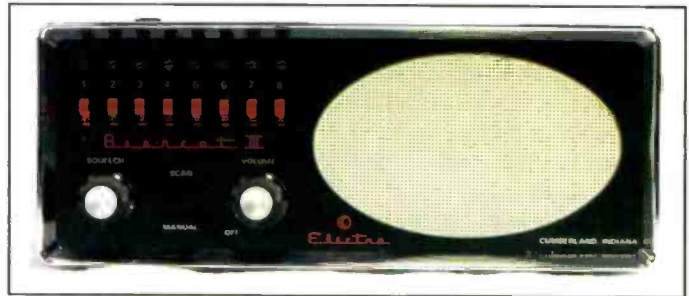
There were scanners. This is actually a Bearcat III, the UHF variant of a very early model by Electra. Electra was later bought by Uniden, which has kept the Bearcat name. This one featured individual channel lockouts, a luxury many scanners didn’t have for quite some time. But it would scan! No more single channel listening!
