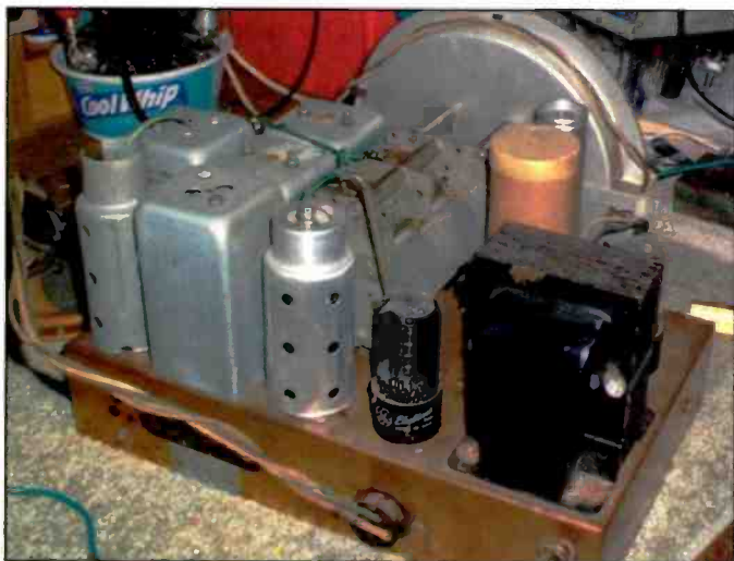
Photo A. This small Zenith chassis will be the guinea pig for our tests. It's a five-tube chassis from a Zenith 5S127 tombstone radio. Many restorers opine that the transformers used in these chassis were underrated by the factory and failure prone, making the Zenith an ideal example for this column.
