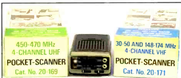
This early RadioShack Pocketscan was a popular handheld in its day. It had four channels and was crystal controlled, so you were pretty much stuck with your choice once you loaded up the crystals and left the house. Later models could do VHF-Hi and Lo in one scanner, but UHF was a separate radio for sure. The radio shown here is VHF-Hi only, and the pin plug (similar to what's used for earphones) that connected the antenna meant that the antenna fell out and got lost quite often.
