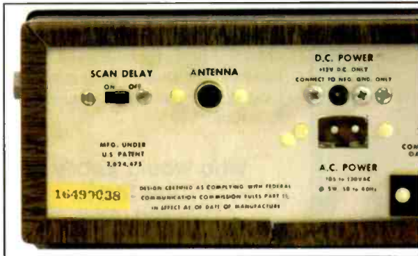
It may seem like a small thing, but having a scan delay on the front panel was quite a feature. Having it on the back panel was equally common, as was not having a choice.
