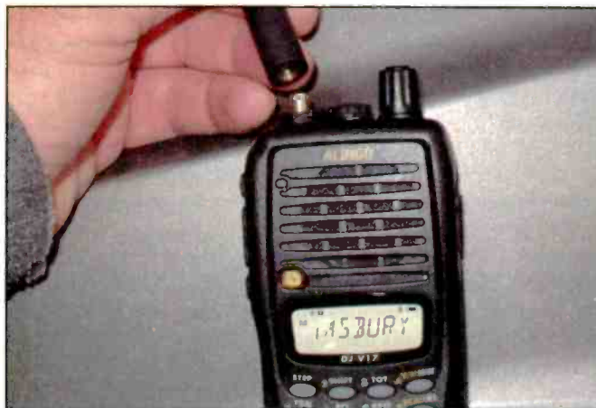
Supplied with an SMA flexible rubber duck antenna, the DJ-V17T is waterproof for up to 30 minutes in three feet of water.
