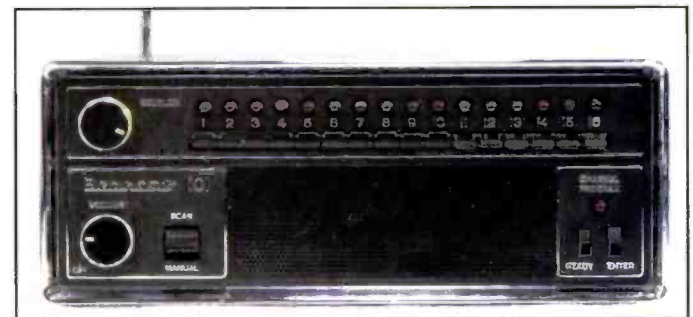
This was the scanner enthusiast's ultimate scanner. No crystals required! Programming the very early processor was done by entering the program mode and then setting the channel switches to up and down positions as dictated in the frequency guide. Once set, you pressed the "enter" button on the right and the frequency was "programmed." It took about an hour to program all 16 channels, but at $5 to $7 a crystal, it was a lot cheaper! It wasn't the first device to allow this, but it was the most popular because it was made by Bearcat. Not too long after, keyboard entry made its debut, but we'll save that for another column!
