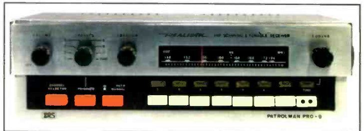
Here was an attempt at the best—or worst—of both worlds. The early scanners required a crystal that had to be purchased separately for each channel you wanted to receive. I remember them at about $5 each, so there’s an additional $40 to load up an eight-channel scanner (not so bad until you consider today’s 400-channel units!). This one had seven crystal positions and a tuner for the eighth. If you found something worth hanging onto, you had to then figure out what frequency it was to get the right crystal.
