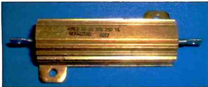
Photo C. This power resistor was made by Dale and is enclosed in an aluminum metal case with mounting tabs. The aluminum case ensures good heat transfer, and the tabs are ideal for mounting the resistor to the metal chassis.
