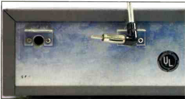
The early scanners and tunables seem to prefer the Motorola pin plug antenna connection. This rear view of the tunable receiver shows the separate antenna jacks for UHF and VHF (behind the antenna showing the plug).
