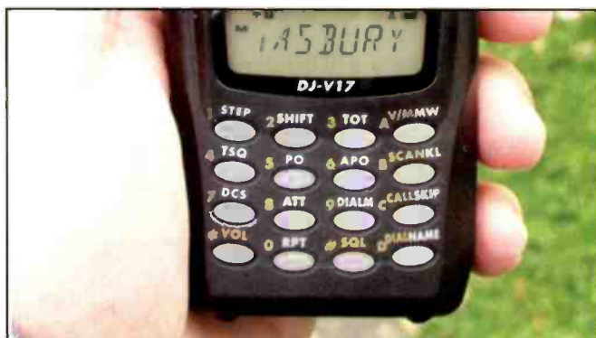
This close-up of the very visible (and lighted constantly if you want to drain those batteries quickly!) display window clearly shows "Asbury." It took all of a minute to label the No. 1 memory slot with easy keypresses. You can give all 200 memories an alphanumeric name (up to seven characters). It sure helps when you're looking at numerous frequencies; I don't have to remember that 154.430 is the fire/EMS frequency for Asbury Park (and other nearby New Jersey towns).
