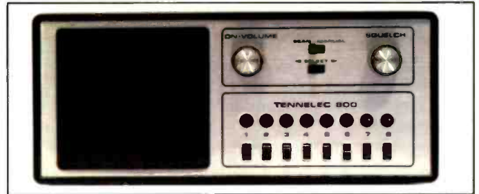
Another little known scanner company was Tennelec. This crystal-controlled unit was one of their early models.
