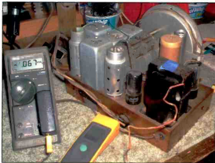
Photo B. Here's how I took the temperature measurements. The first instrument converts temperature to a 1 mV-per-degree output for use on a sensitive DVM. It uses a thermistor pickup, which must be placed in direct contact with the part being measured to take a reading. The other instrument is an infrared thermometer made by Fluke. It's marketed for locating hot circuit breakers in electrical boxes. It doesn't require physical contact to take readings, but the most accurate readings are made on dark and non-shiny surfaces.
