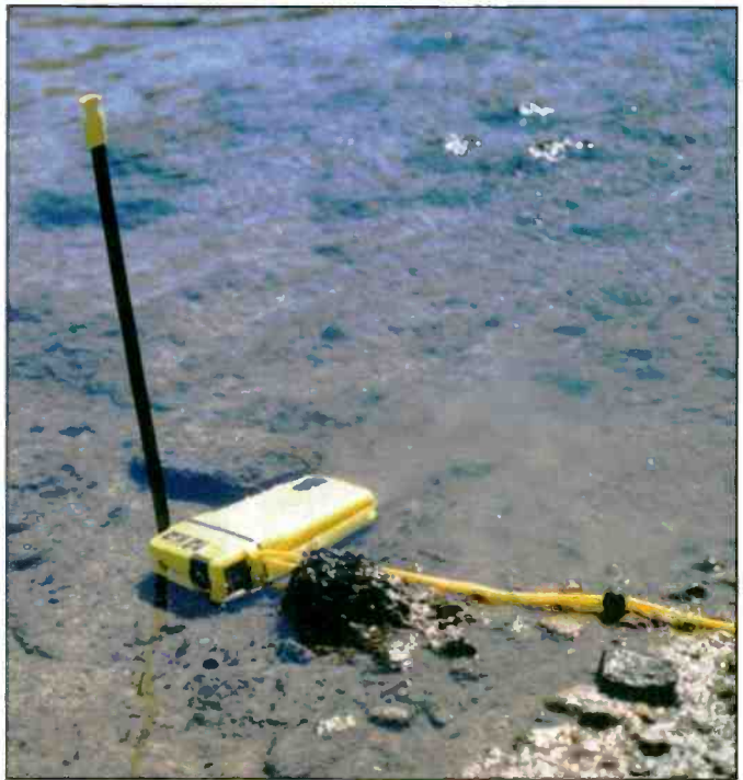
The test signal on 121.775 was increased by 3 dB by placing the test PLB on a water groundplane.
