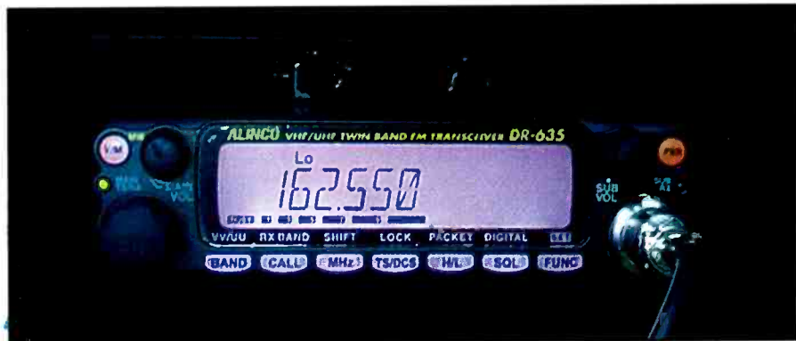
The 635T's front panel mounted to the plastic bracket, which tilts for just the right viewing angle. The modular cable is routed to the left and under the door floor panels.
