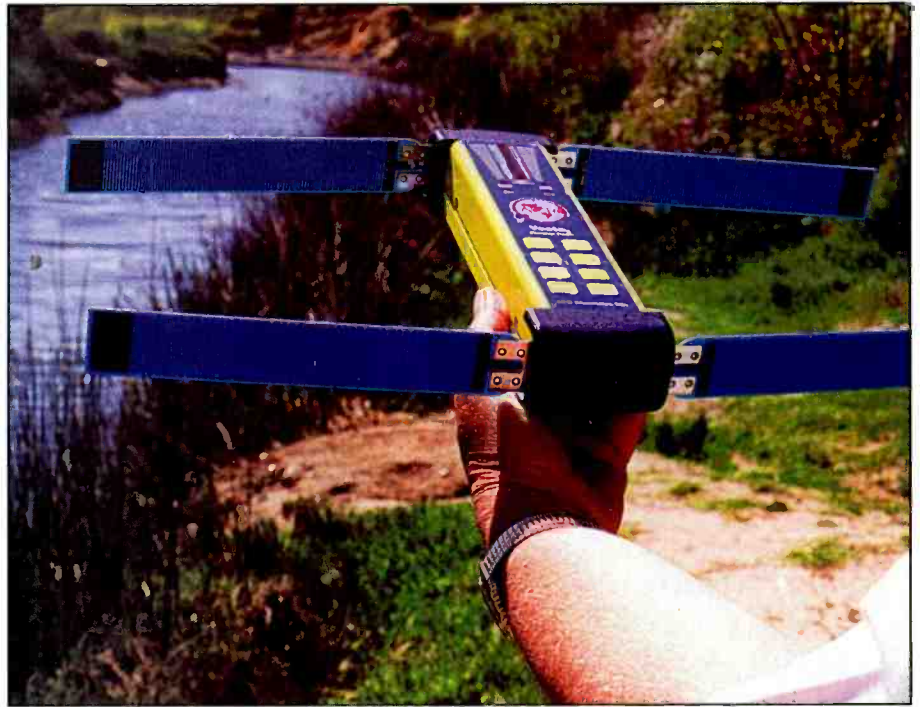
The ACR Direction Finder in a real 121.5-MHz track-down along a popular river rafting route in a remote area.
