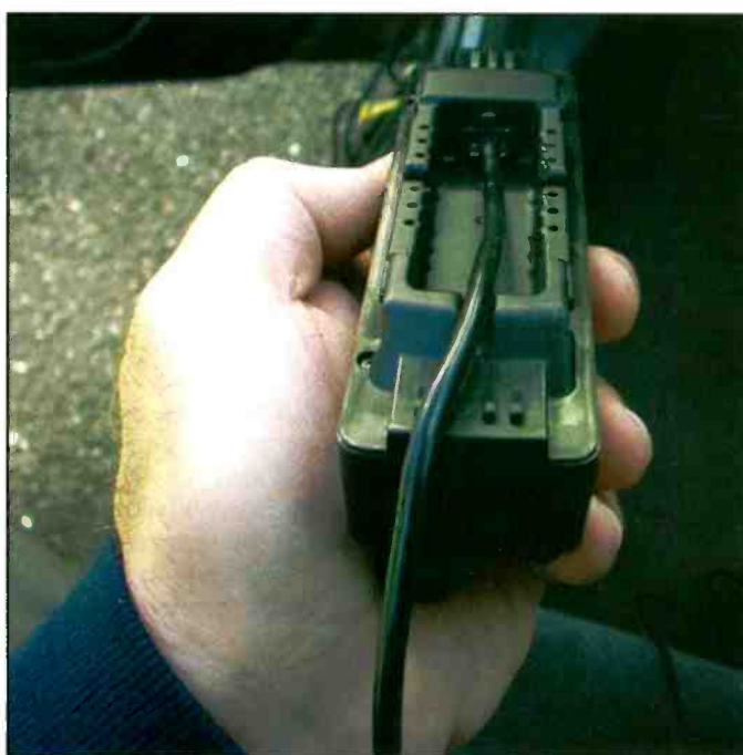
One end of the 16-foot modular cable plugs into the 635T's front panel; the other end routes to the 635T's main body. Ours is in the trunk.
