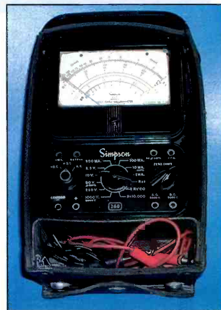
Photo D. The Simpson 260 series VOM meters remain in daily use in the electronic industry. While the increasingly popular, and low-cost, modern digital meters have lessened their popularity, the 260s are still in production.
