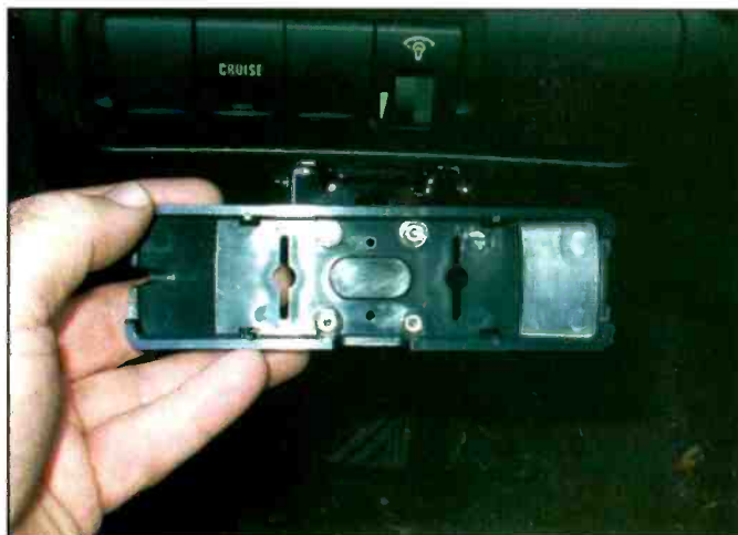
The best mounting location in our vehicle required using both the plastic and angled metal bracket.
