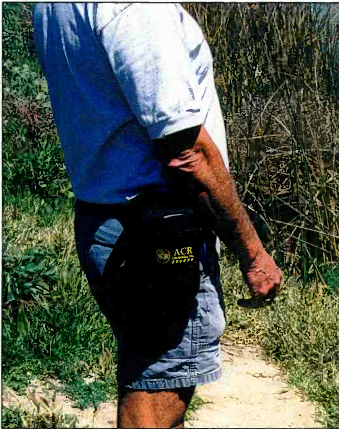
PLBs are small enough to wear, but they must be placed out in the open to signal satellites.
