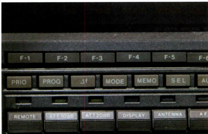
Higher-end receivers have built-in attenuators. On newer receivers, attenuation can be set by channel, while older ones have an on/off switch (frequently on the back) and it's either on for everything or off for everything. This receiver has two stages of attenuation.
