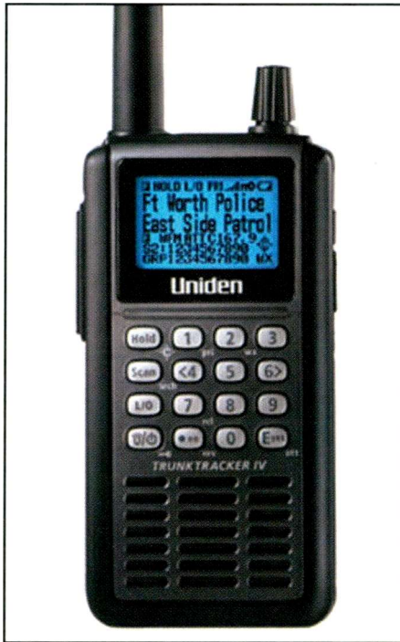
The Uniden 396T is a full-featured handheld scanner that receives 25 MHz to 1.3 GHz.
