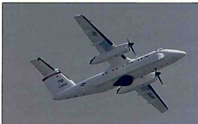
Widget 48, the second of the two existing E-9A aircraft, is seen here with its belly-mounted sensor pod clearly visible.
