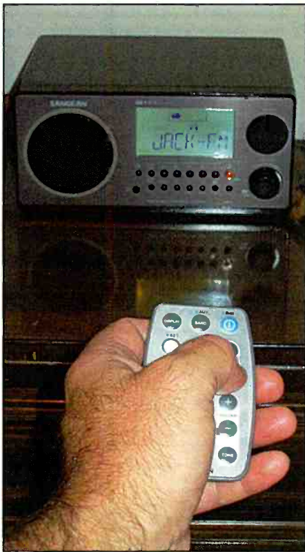
The remote operates on a single CR-2025 battery (included) and controls a multitude of functions.
