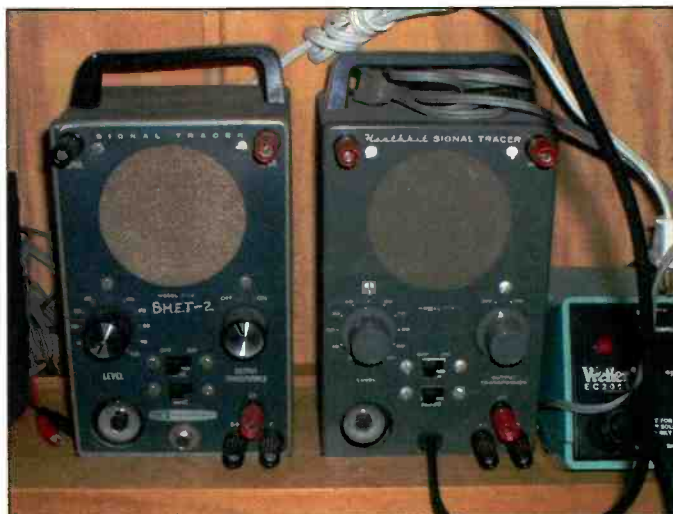
Photo C. These two Heathkit signal tracers have the "noise" feature to isolate parts that might be breaking down under operating voltage. I'll be doing a piece on troubleshooting by signal tracing in a future column, and I'll show you how to restore these nifty instruments as well!
