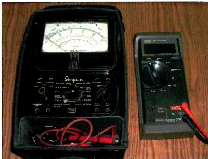
Photo D. These simple meters are all you need to measure and test resistors.
