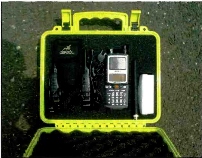
The only items not packed in the case are the small manuals for the scanner and (only one, of course) for the Midland GMRS/FRS handhelds, and the PC control cable for the BC-296D. It's a snug, perfect fit!
