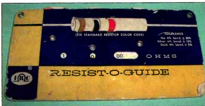
Photo B. Most resistor manufacturers provided a complimentary decoder to help decipher resistor values. This is an example IRC's Resist-O-Guide. Contemporary equivalents are computer programs, available as free downloads for Windows operating systems! They're more trouble than they're worth, however, in my opinion!
