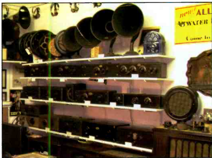
These shelves display Atwater Kent radios dating from 1925 to 1929. The odd boat-funnel shaped objects on the top shelf are in reality early horn speakers and are representative of what would have been used with those early Atwater Kent battery sets.
