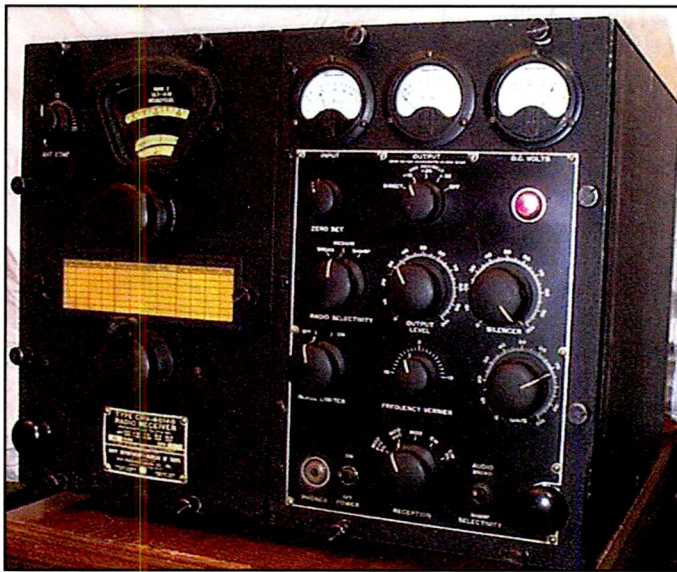
Here's an example of a WWII vintage U.S. Navy receiver that represents the analog way of doing things. It was big, heavy, and powerful, but it received only one frequency at a time. It worked in its day, but only with a lot of human intervention and interpretation.
