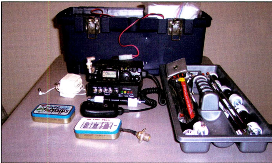
David R. Hassall, WA5DJJ, of Las Cruces, New Mexico, furnished the following photos of his FT-817 portable EmComm Jump-Kit. Dave uses a plastic tool box from a major home improvement center. Notice how things just "fit together" to make a nice rugged, portable Jump-Kit. Dave, like me, favors the Yaesu FT-817 QRP transceiver as the prime mover for his EmComm gear. The toolbox shows all the "stuff" that goes inside to complete his RF gear for emergency communications work.
