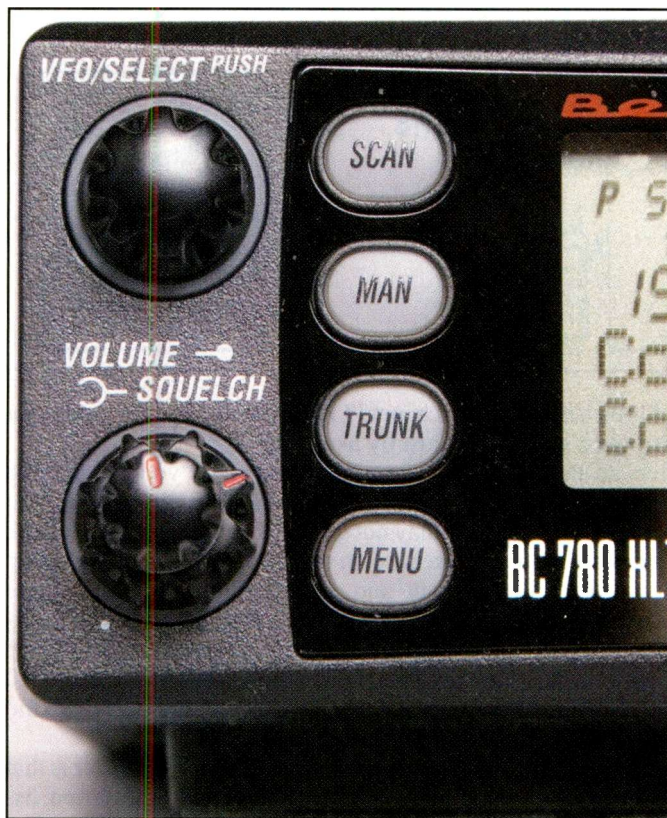
Putting the scanner in MAN mode allows you to follow the action very closely on just one channel. You'll learn a lot in a short time this way.
