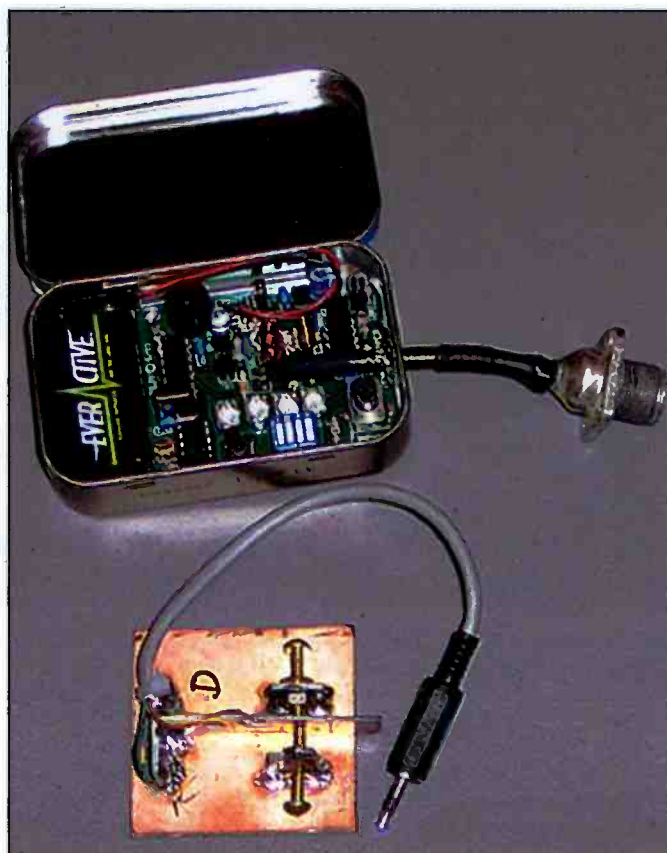
This picture shows the KD1JV Antenna Analyzer in an Altoids tin along with a homebrew CW keyer and the paddle set made from a pc board. To keep weight and mass down, Dave went to extremes building these two devices into one Altoids mint tin.
