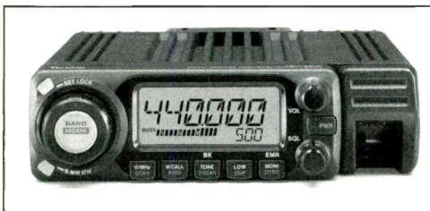
The new ICOM ID-800 is a full-featured 2-meter/70-cm voice and data comms mobile transceiver.
