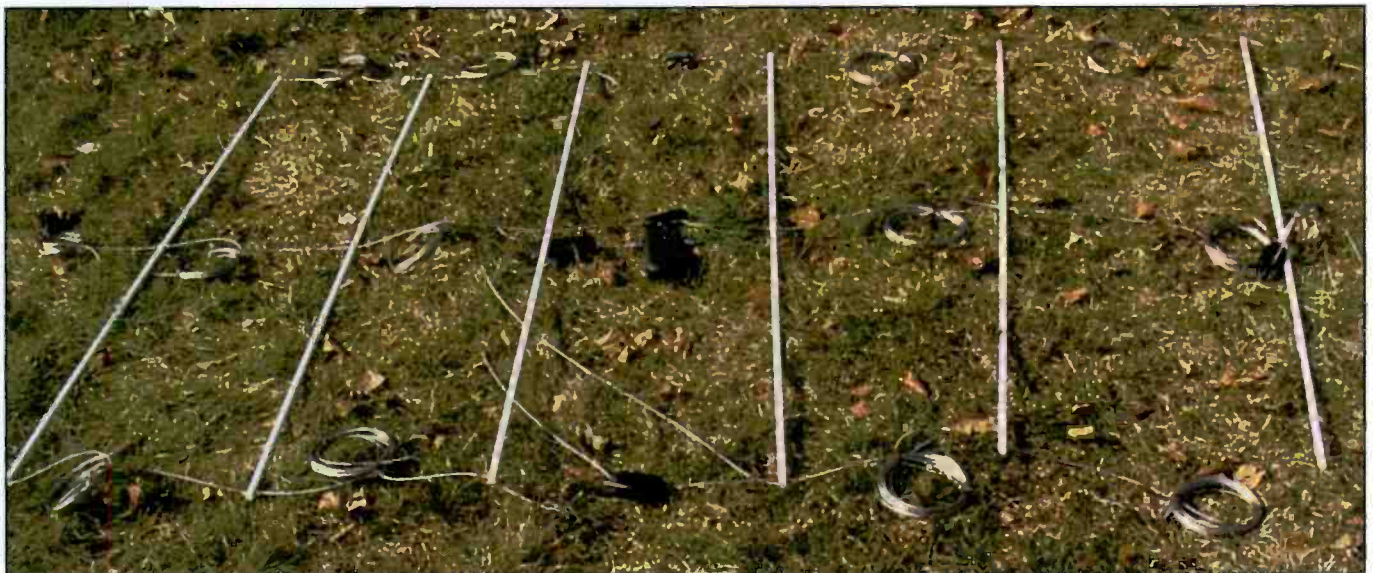
Here you see the antenna unfolded with the six fiberglass spacers and eight taped coils.
