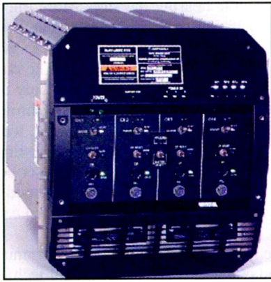
The AN/USC-61 Digital Modular Radio (DMR). The new radio communications standard for the U.S. Navy for the 21st Century. Able to transmit on any frequency between 2 and 2000 MHz, this unit is no bigger than a mini-fridge and can be programmed into any configuration needed "in the field" using the appropriate software program. (Photo courtesy Joint Tactical Radio System Program Office)
