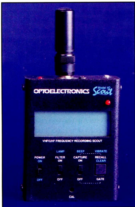
If you're close to the action, a near field receiver like the Scout or Xplorer from Optoelectronics might be a handy device. Further away, you'll need some frequencies programmed into your scanner in a hurry.
