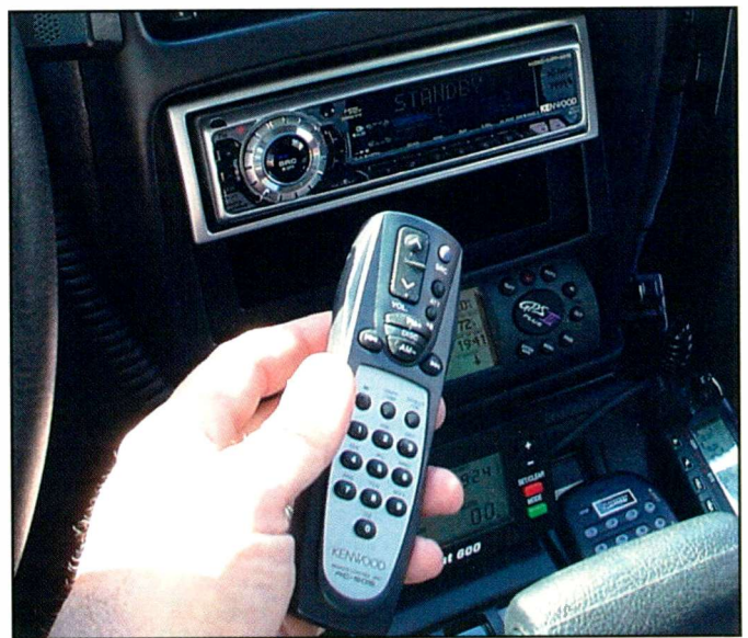
The Kenwood KDC-MP425 receiver control head unit comes with an infrared wireless remote control. While at first this may seem like overkill for use in an automobile, it is a necessary accessory. This is because there is no room for a digital numeric keypad on the control head itself, hence the keypad on the remote.
