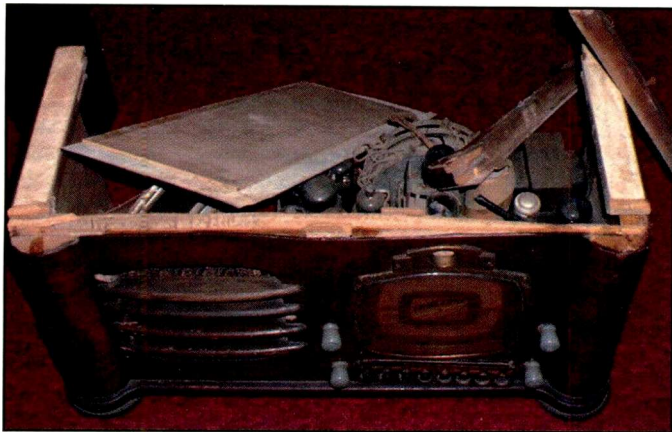
Photo D. This large Detrola model 175-E table radio, circa 1937, features 10 tubes and push-pull audio, motor-driven station presets, a tuning eye, and a gorgeous tuning dial and front panel presentation. What should have been a $100 to $300 radio was transformed into a $25 junker (parts set) by years of careless storage. Poor shipping concluded the damage.
