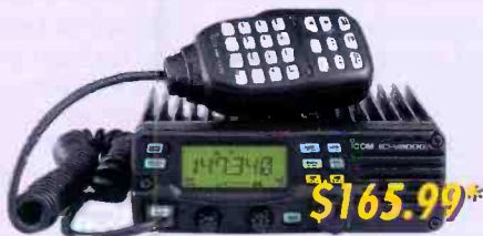
IC-V8000 Offers 75/25/10/5W output. With clear, operator-facing speaker, the 2M features CTCSS/DTCS, DTMF encode and 207 memories. 5.9" w x 1.97" h x 5.9" d, 2.22 lbs.
