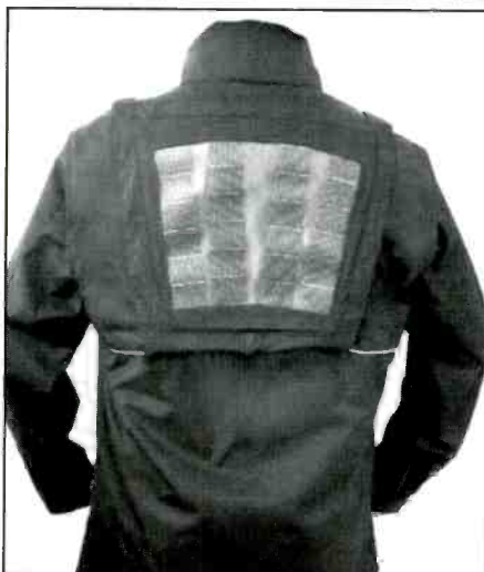
The Solar SCOTTeVEST includes solar panels that charge a small battery.
