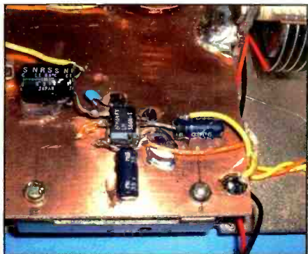
Photo D. The audio amp IC is mounted using "dead bug" construction techniques. The larger parts are glued to the pc board to alleviate stress on the IC leads.
