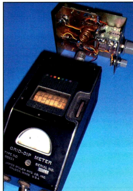
Photo B. Here's the Millen Grid Dip Meter in action! When tuned to the resonant frequency of the capacitor and coil, the meter on the Millen will dip to a lower value. Fifty or 60 years ago, every ham owned one of these useful pieces of test equipment. That was a time when hams built their own gear. Now using one has become an archaic art.
