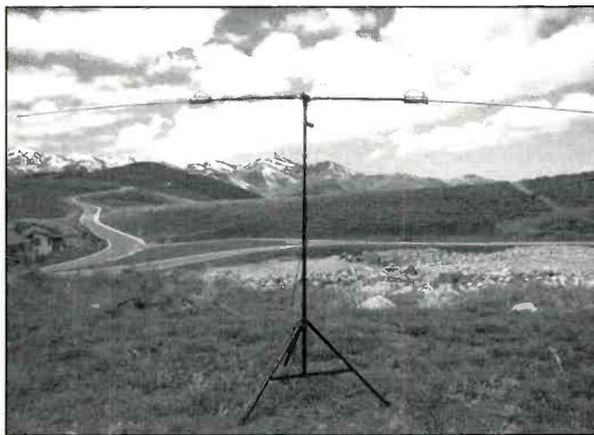
The W3FF Buddipole is a versatile antenna system that costs $199 direct from sales@buddipole.com . The company also offers a 35 optional rotating arm kit that allows you to change the antenna's configuration in the field. →
