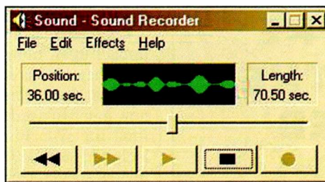
Photo E. A glimpse of the Sound Recorder software in operation recording sound off the air. Note that the "Oscilloscope" is showing the volume level of the sound being recorded. The length of time that the recording has been made is shown, as well as the "position" of the slider. The slider can be used for editing the sound recording later on. You stop the recording by clicking on the square, and then saving the file by clicking on the "File" pull down menu and giving the sound recording a file name.
