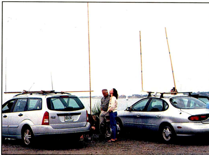
Patriot DXers admire the phased arrays perched atop these cars in Rockport, MA to catch transatlantic mediumwave signals during the DX Clams expedition.
