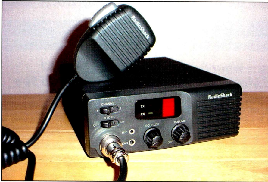
The RadioShack model 19-1210 mobile transceiver for MURS and licensed business itinerant use. (All photos courtesy of N3HOE.)
