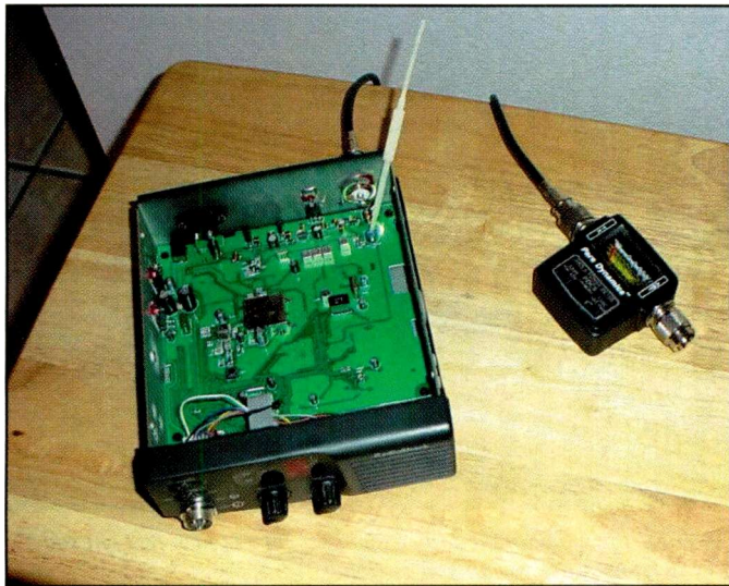
Transmit power adjustment setup conceptual illustration. A single coax jumper runs from the 19-1210's antenna connection to an RF power meter's TX connector. A small dummy load (5 watts) is screwed onto the meter's ANT connector.
