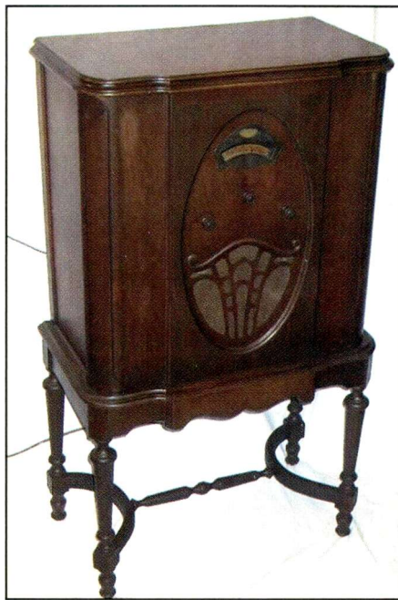
Photo G. John brings the radio back to displayable condition by applying a new finish coat of Minwax. The Minwax, applied with a white Scotch-Brite, acts to soften and reamalgamate the damaged lacquer, much in the same manner as the toluene in BriWax. (Photo courtesy: John Hagman)
