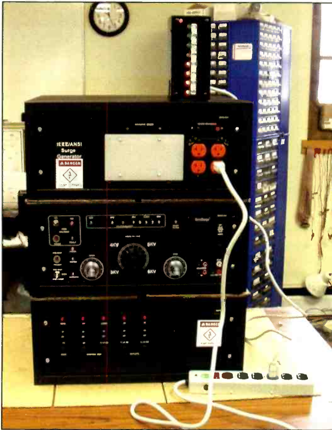
ZeroSurge's 6000-volt, 3000-amp generator getting ready to—literally fire up a consumer-grade suppressor.
