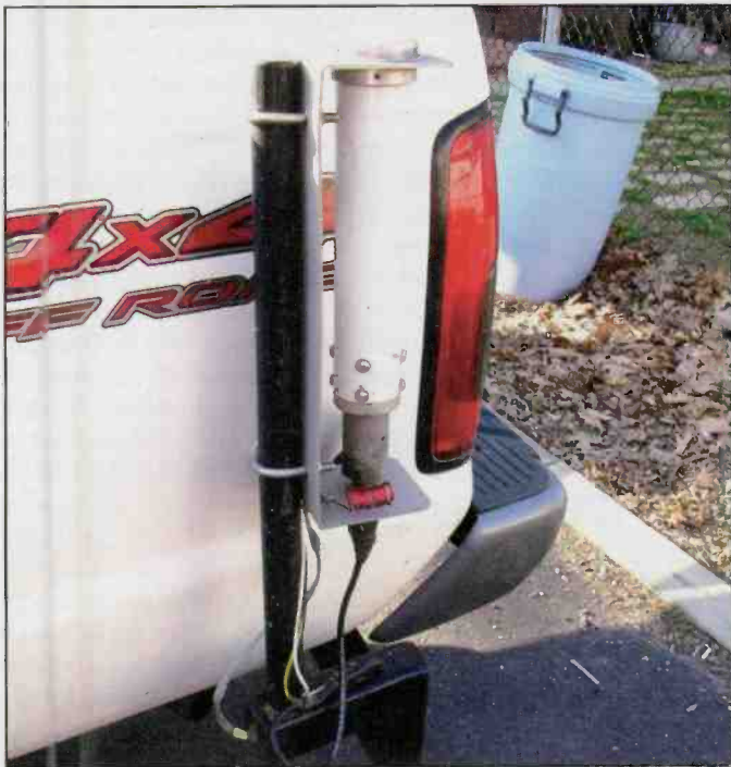
Here is a close up of the Tarheel model 200 antenna mount. This is a quick-disconnect mount to allow the cylindrical lower portion of the antenna to be quickly removed for storage in the bed of the truck. The actual steel portion of the mount that connects to the truck frame is extremely rugged, as can be seen in this photo.
