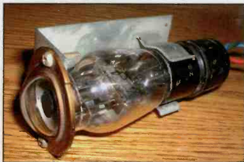
Photo C. Companies offered Magic Eye kits, usually consisting of a socket, bracket, and eye tube bezel. They permitted quick one-hole mounting to add Magic Eye tuning to existing radios and provided an incentive for amateurs to use the eye tubes in their projects.
