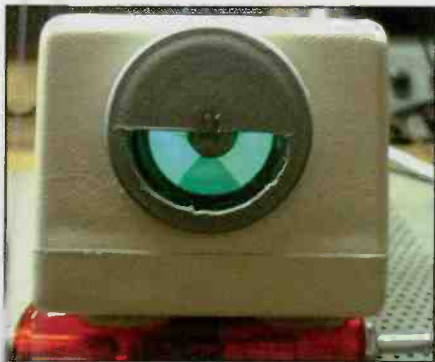
Photo K. Unfortunately, the proper metal bezels are hard to come by, but a passable bezel was made by cutting an opening in a lid from a 35-mm film canister.
