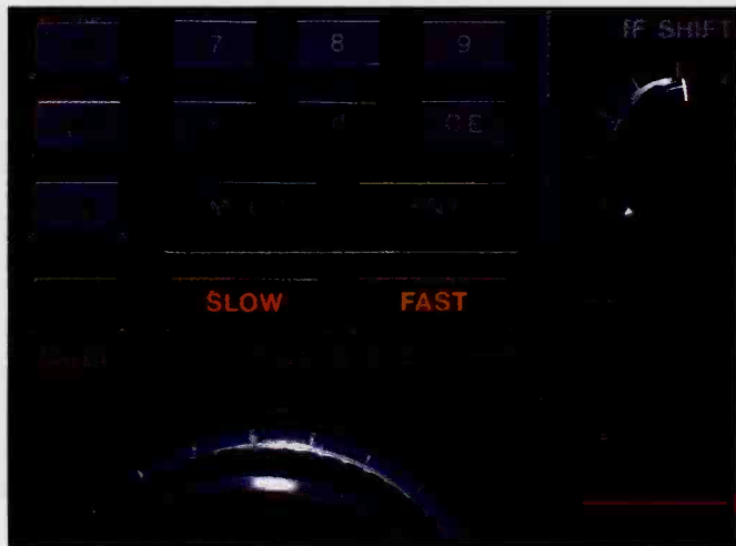
This receiver adjusts the step using SLOW and FAST keys to step through a wide range of available step sizes.
