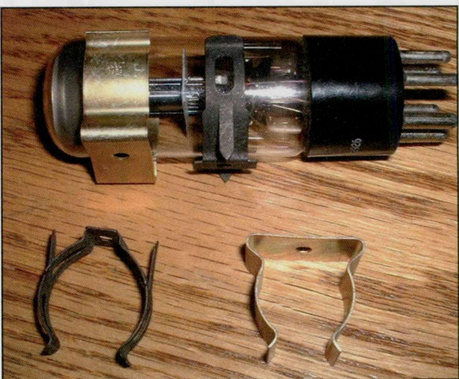
Photo J. Another way to mount the eye tube is to support it with spring clips as shown here and similar to the technique shown in Photo C. These clips are normally used to chassis mount components and support parts such as large tubular capacitors.
