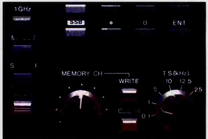
This receiver has a dial in the lower right corner that determines the step size. Any of the methods works just fine, as long as you can get to the frequencies that are in use!
