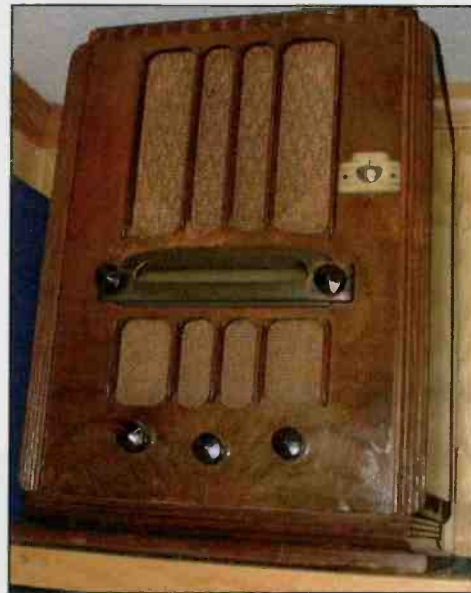
Photo D. GE sets get no respect! Their "Plain-Jane" styling, ugly fish-mouth bezels, and slide rule tuning is disdained by many collectors. Yet these are powerful and strong-playing radios, really RCA designs in disguise! The eye tube was an after-market add-on made shortly after the radio was sold.
