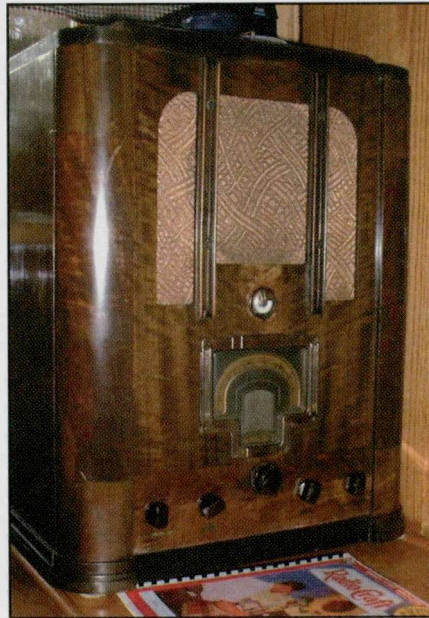
Photo A. This large RCA 10T tombstone was the RCA flagship tabletop model and featured the newly developed magic tuning eye. Despite its high cost, the RCA radio wasn't particularly attractive, and the eye tube looks like an afterthought.
