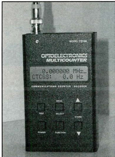
A few counters like this CD100 from Optoelectronics can actually grab the tone information off the air for you — if you can get close enough to the signal to get a reading!
