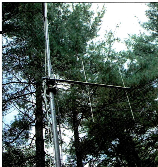
Shaped-response antenna keeps a vigilant ear on news events as they unfold in Strafford County while rejecting unwanted squelch bursts from out-of-area signals.
