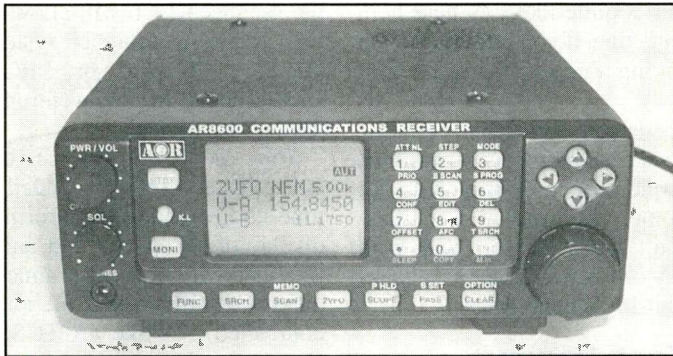
This top-of-the-line receiver from AOR has a tone squelch module that is optional. This also applies to the popular AR-8200 handheld scanner. The 8600 has mul-tiple card slots so that tone squelch can be used with other features.
