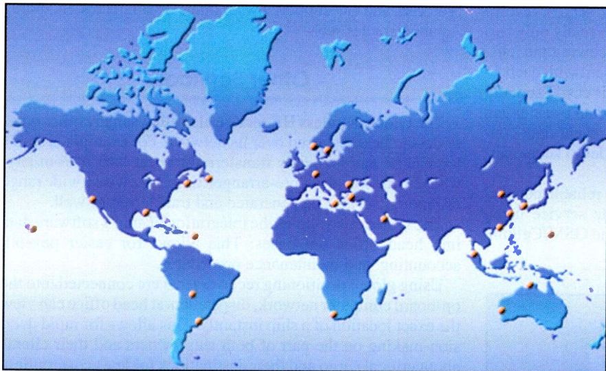
Each of the dots on the map represent a Globe Wireless Digital Maritime Data Network "Node". Each of these Nodes is connected to an HF transceiver that allows an on-board computer network to connect to Globe Wireless's own network, which then connects to the Internet. (Map courtesy Globe Wireless).
