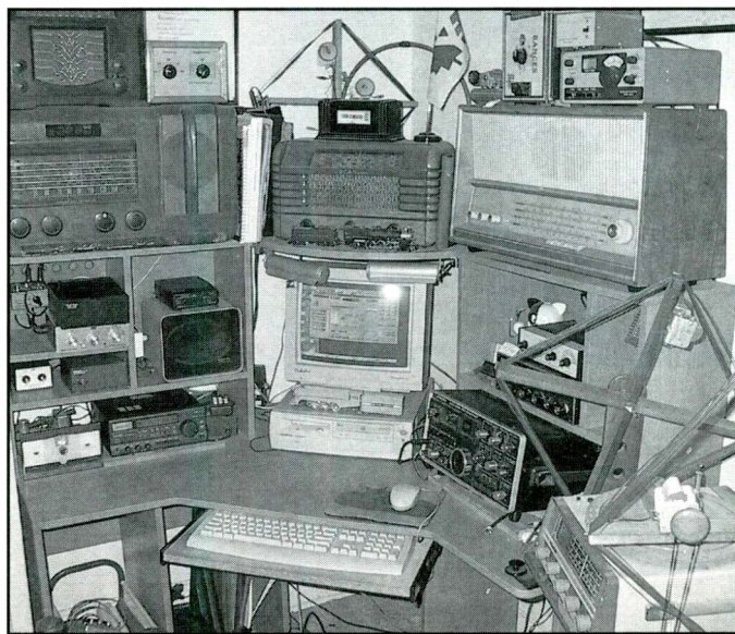
Radio has a long history, and is still undergoing many changes. The center of many monitoring stations is the personal computer with specialized software installed for logging, decoding, and the direct control of radios.
