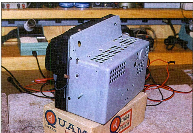
Photo 2. Rusted areas on the rear case and cover were sanded clean and sprayed with two coats using a gray protective enamel primer.
