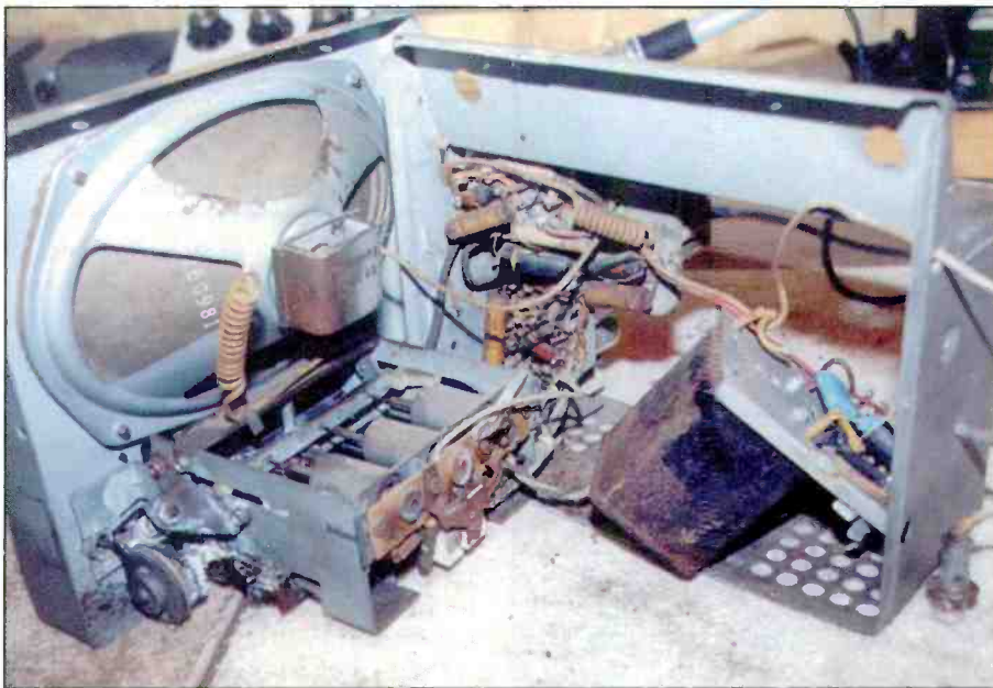
Photo 3. Peeking inside the front of the radio shows the various sub assemblies. This is not a first-time project for beginning restorers!
