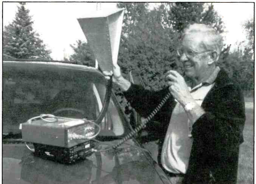
Gordo demos aircraft scatter, harmlessly bouncing 10,000 MHz off a low-flying Alaska floatplane. The green box on top of the Kenwood radio is the transverter.
