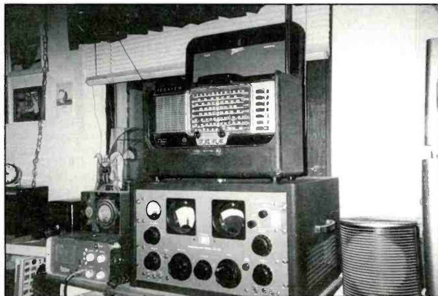
Here's a shot of "part of" Rick Barton's shack in Arizona, showing two classic radios — a Zenith Transoceanic sitting on top of one of those great Hammarlund 600 series.
