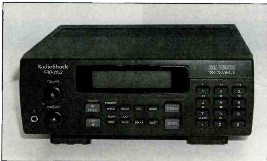
This unique base scanner features 20 banks of 50 channels each. Extra banks and channels make it very convenient to have event banks pre-loaded.
