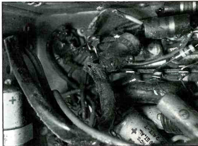
Photo 1: What can go wrong when a wax capacitor fails? This line-bypass let go with a spectacular display of smoke and flame!
