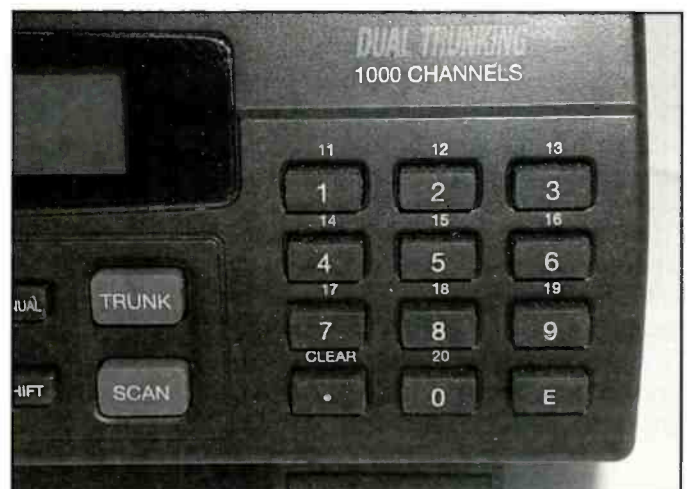
If you look closely above the keys, you'll see the designation for the second 10 banks. This is the PRO-2052 keypad, but a few other models also feature the 20-bank arrangement.
