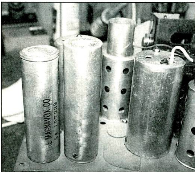
← Photo 1. The electrolytic capacitors after being cleaned and rebuilt. The aluminum shells were gently cleaned in a large ultrasonic cleaner.
