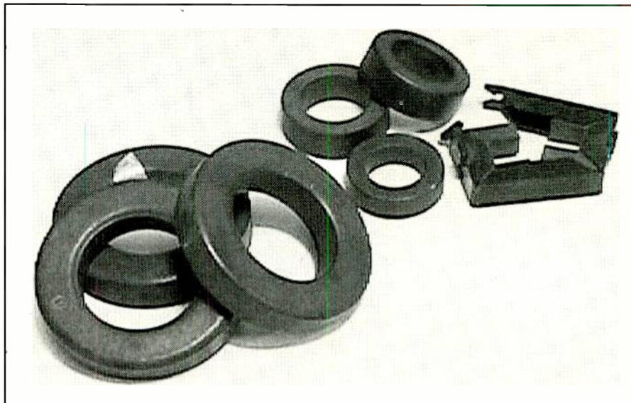
Ferrite cores from large to small. If RFI sleuthing is on your agenda, you'll probably be using these cores to build common-mode RFI chokes.
